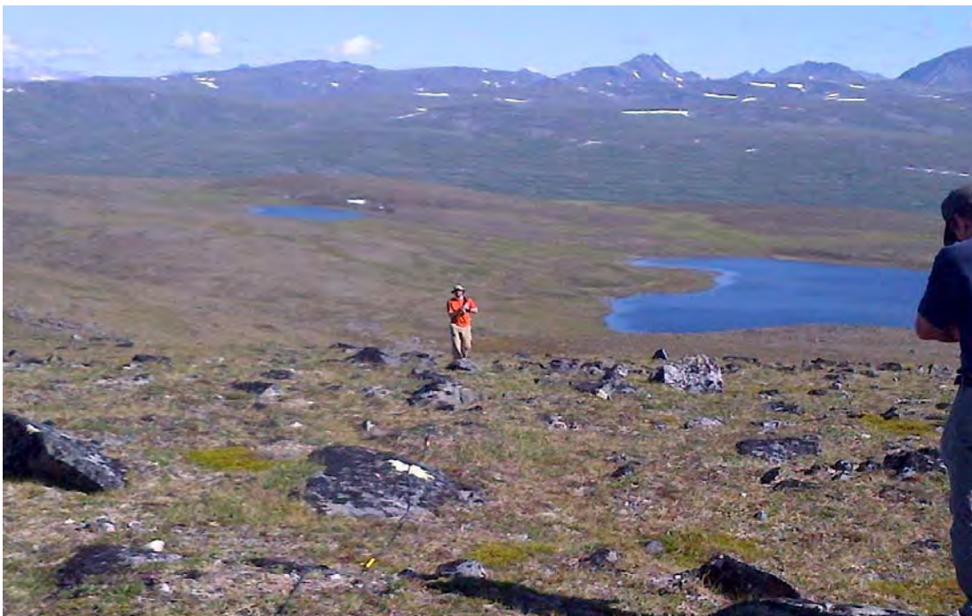
WAT-7, looking north, northeast along the N-S line towards the north end of the line. Fugro crew in orange shirt is performing sledgehammer hits during data acquisition.
