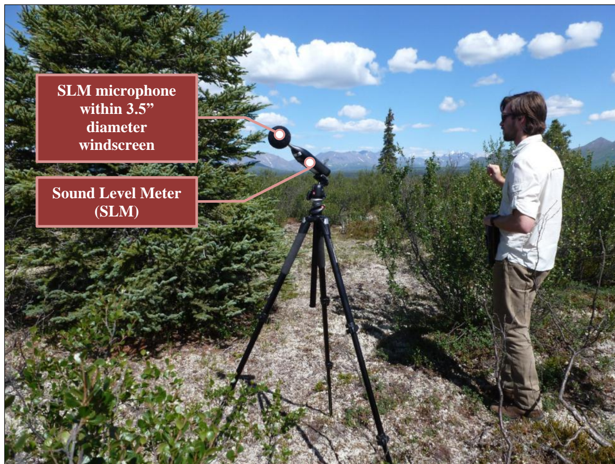
Figure 4-2. Typical Components of a Short-Term (ST) L_p Measurement Setup
