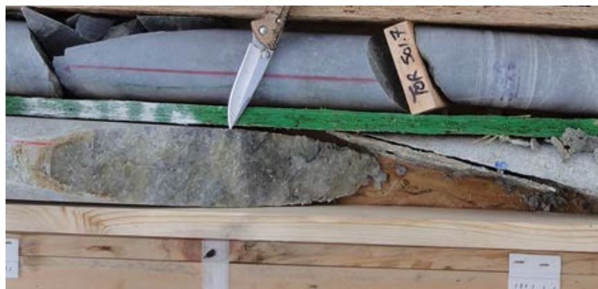
Figure 6.3-29. Close-up of Shear Zone with Slickensides in DH14-10 at Depth of 507 ft.
