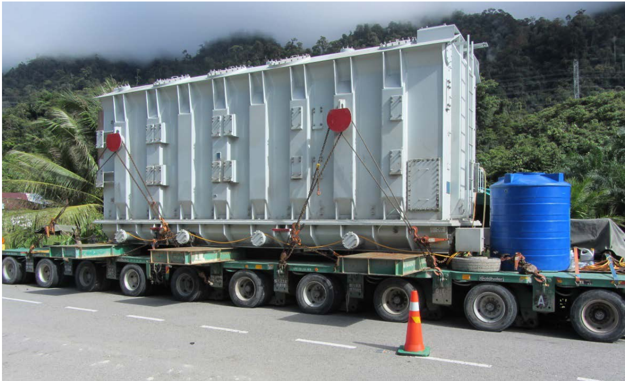
Figure 13.3-9. Transformer Transport by Road
