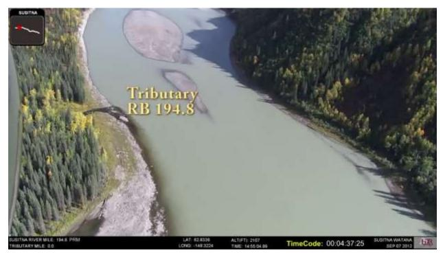
This unnamed tributary flows into the Susitna River on river right at PRM 194.7. The tributary drains over 200 km<sup>2</sup> (124 mi<sup>2</sup>) and includes a few tributaries and many lakes. The main stream channel is roughly 11.4 km (7.1 mi) long. This stream was assessed for the presence of adult salmon passage barriers in 2012; no barriers were identified.
