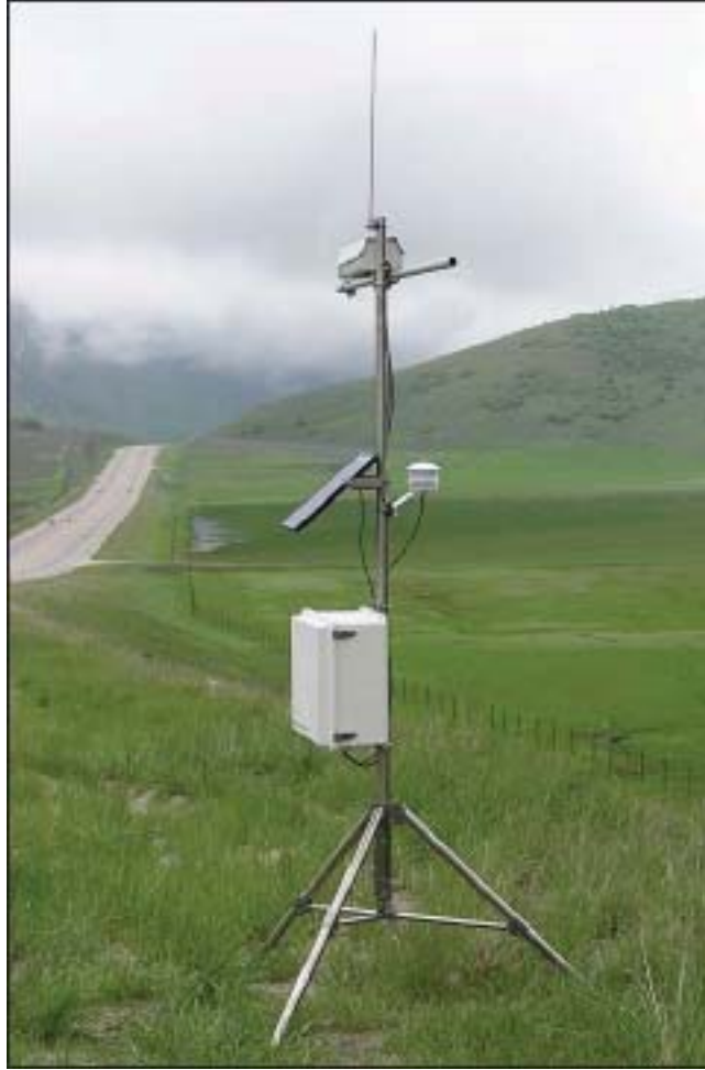
Figure 5.5-2. Example of a 10-foot (3-meter) tripod MET station (guy wires for stabilization and an enclosure will be installed).
