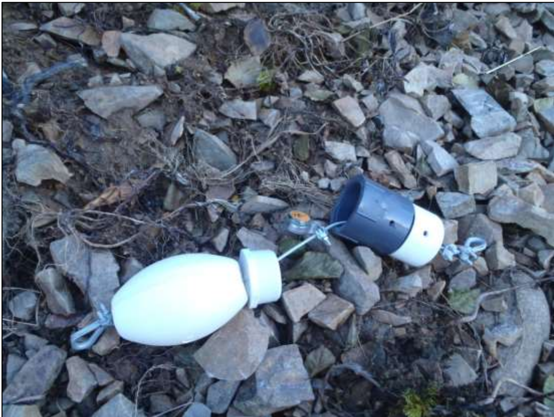
Winter buoy system prior to deployment at RM 181.3 – Tsusena Creek
