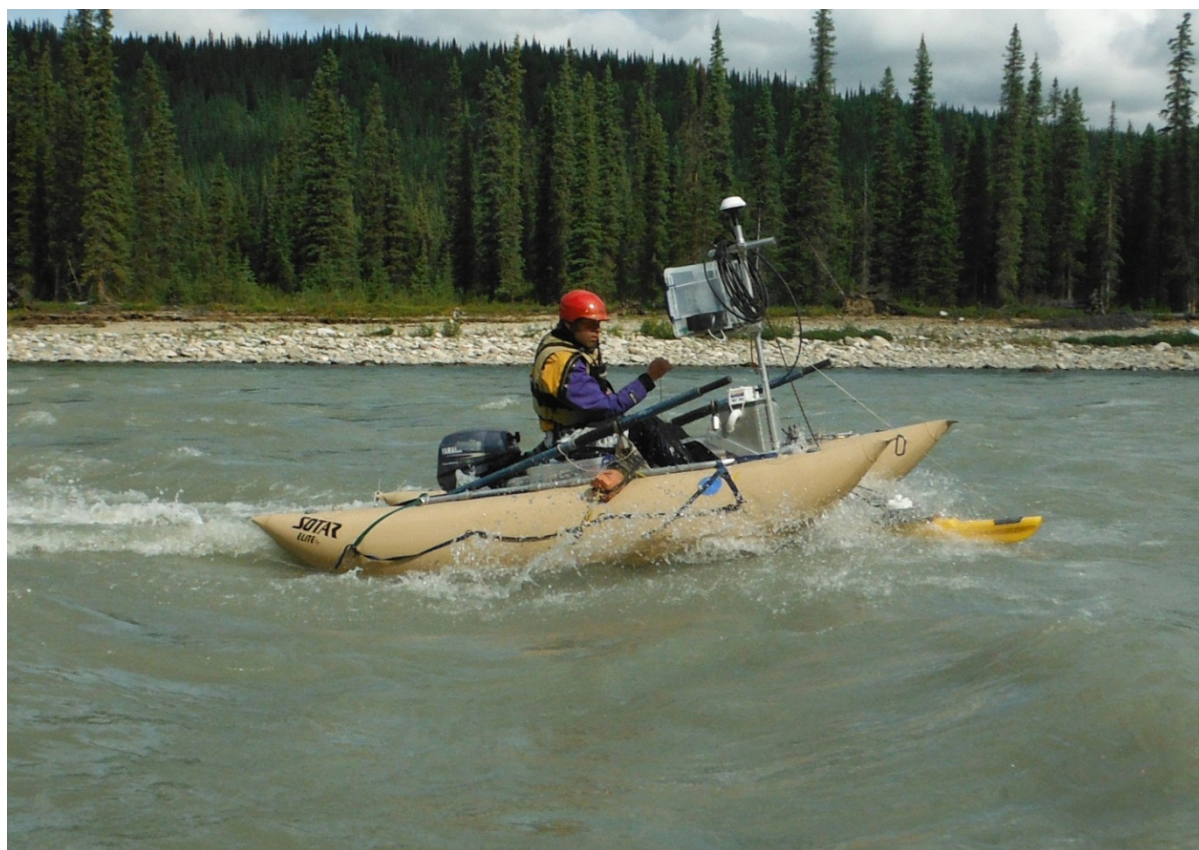
Figure 3.2-1. ADCP catamaran in 1-foot standing waves at PRM 183.5, August 7, 2012.
