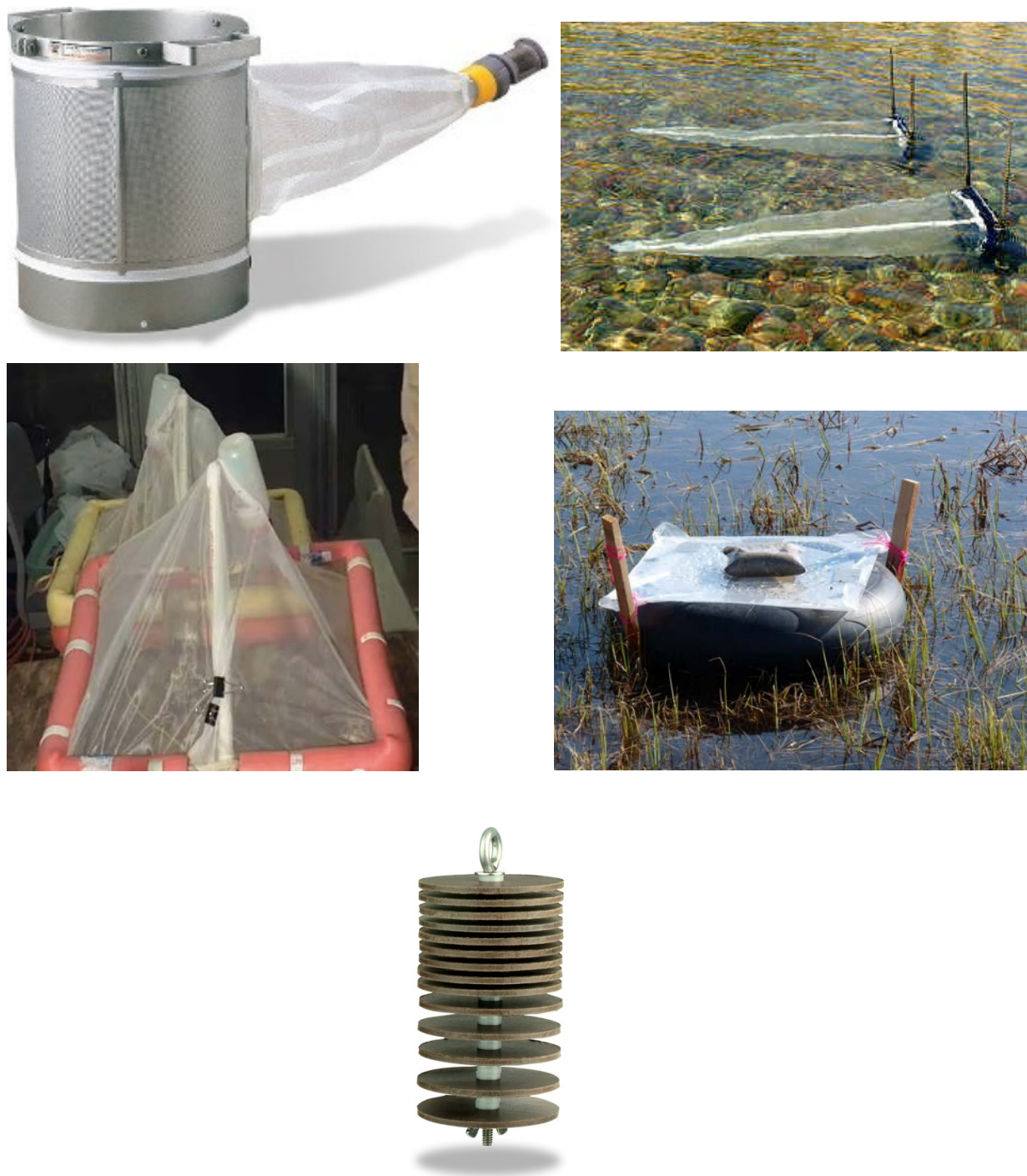
Figure 2.2-1. Sampling equipment used to collect benthic macroinvertebrates in streams and rivers. Top left: Hess stream sampler. Top right: drift net. Middle: examples of floating aquatic insect emergence traps. Bottom: Hester-Dendy multiplate sampler.
