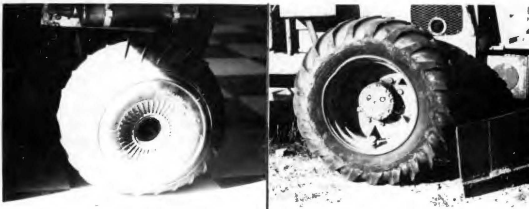
Fig. 4. (left) A typical six-wheel ATV tire on a flat, level surface. Note its similarity to the heavy treaded tire in Fig. 5. (right)
