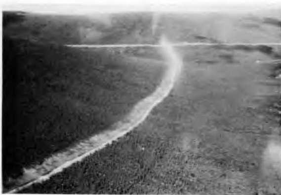
Fig. 1. (left) Water ditch--aerial view. The ditch was constructed in June 1974 by a miner to bring water to his claims. It has not been used. Located on d-1 lands near Eagle Summit on the Steese Highway, it is about 3 miles long. Fig. 2. (right) Water ditch--ground view. The miner constructed the ditch by bulldozing surface vegetation and mineral soil downhill to form a berm. The disturbed area is about 150 feet wide. Several breaks have occurred from normal surface runoff.
