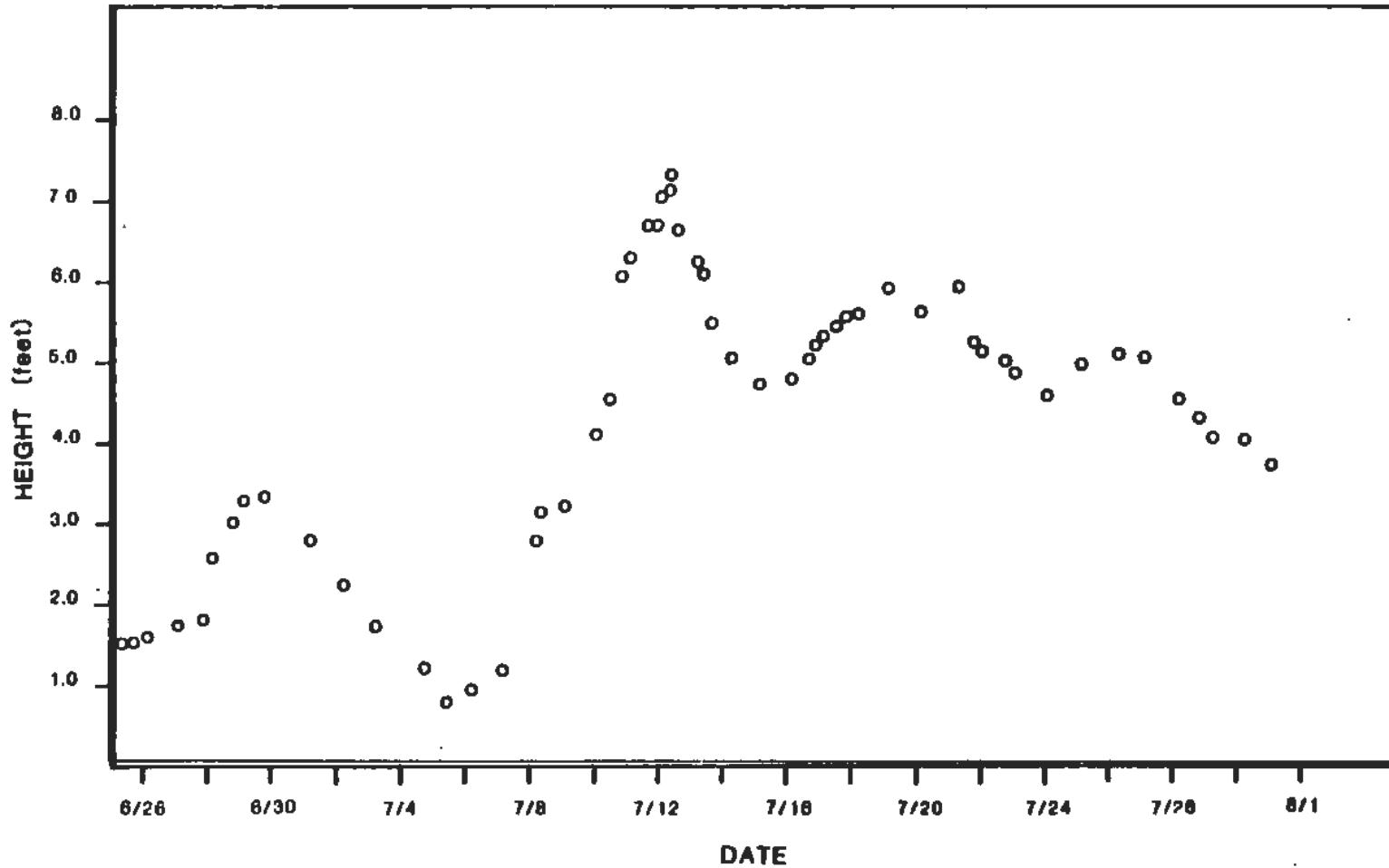
Figure 120. Stage versus time for the AA Talkeetna fishwheel and sonar site (RM 101.0, 27N05W26DDA).
