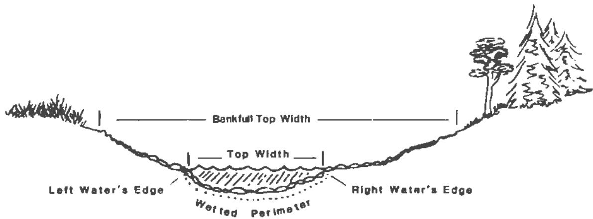
Figure 4. Cross-Sectional Profile Diagram.
