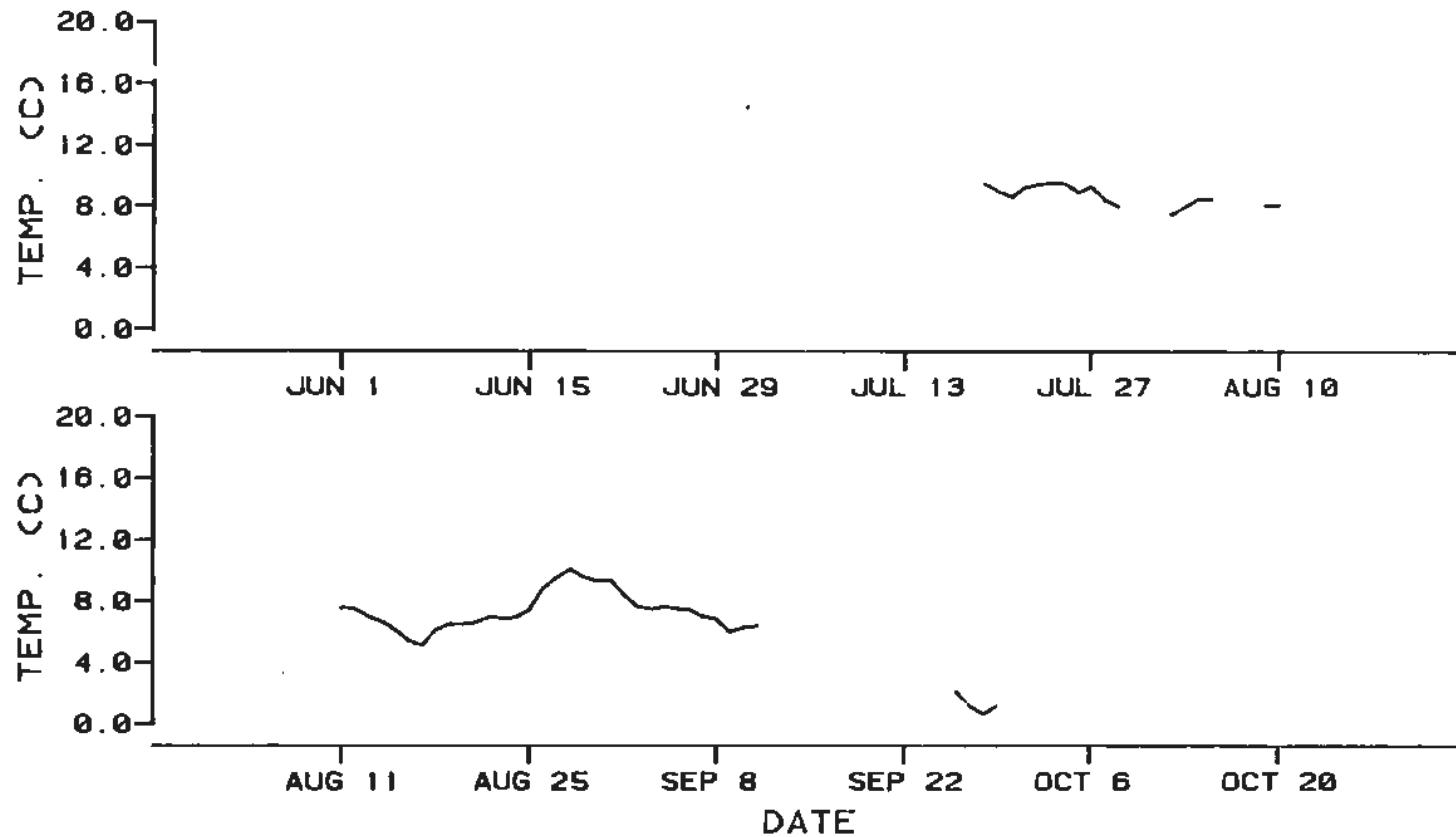
Figure 113. Water temperature versus time for the mainstem Susitna River above Indian River (R.M. 138.7, 31N02W09DCB).
