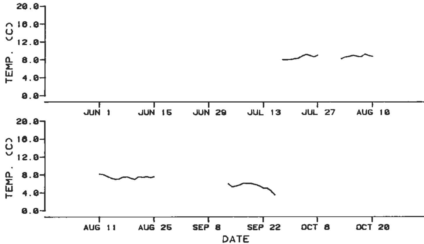
Figure 112. Water temperature versus time for Indian River (R.M. 138.7, 31N02W09CDA).
