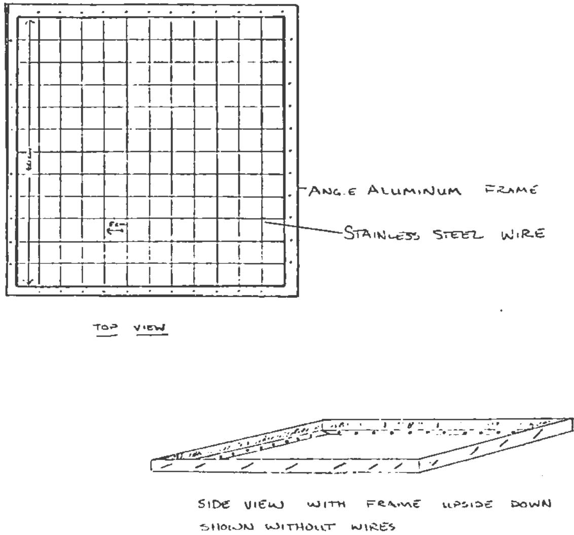
Figure 3. Substrate Grid Diagram.
