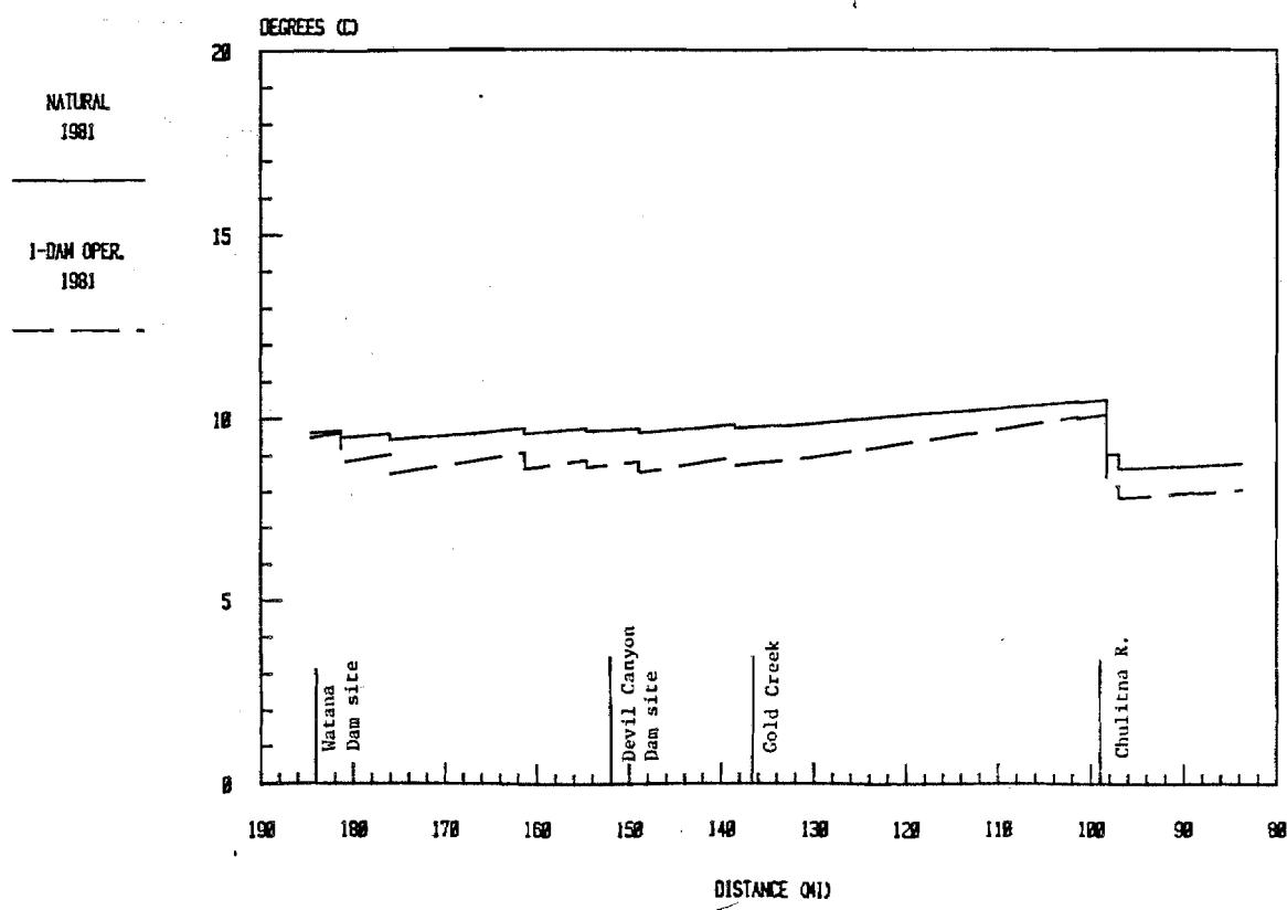
Figure 9 (Continued). River temperature profiles for natural and 1-dam operational conditions.
