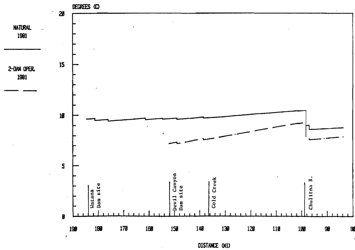
Figure 10 (Continued). River temperature profiles for natural and 2-dam operational conditions.
