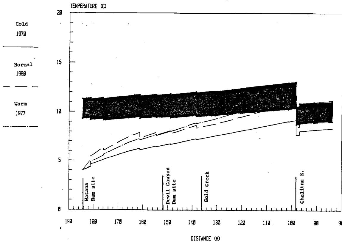
Figure 8 (Continued). River temperature profiles for second year of filling Watana reservoir. Shaded band represents range of simulated natural temperature conditions.
