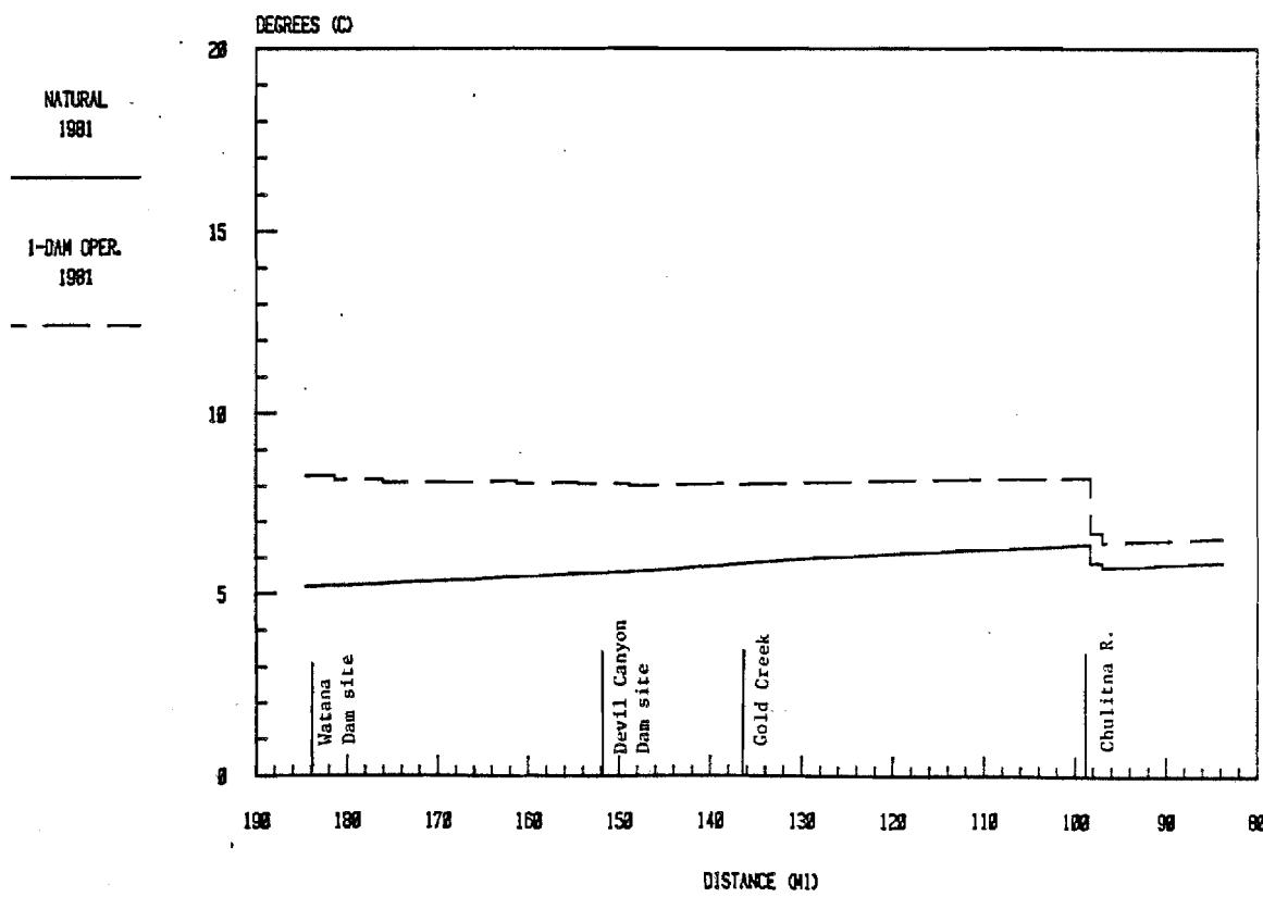
Figure 10. River temperature profiles for natural and 2-dam operational conditions.
