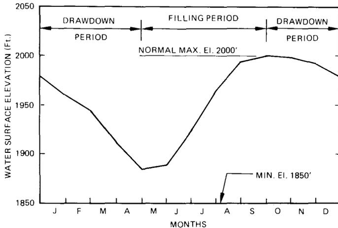
Figure 3. Example Rule Curve For Watana Operation, Year 2004
