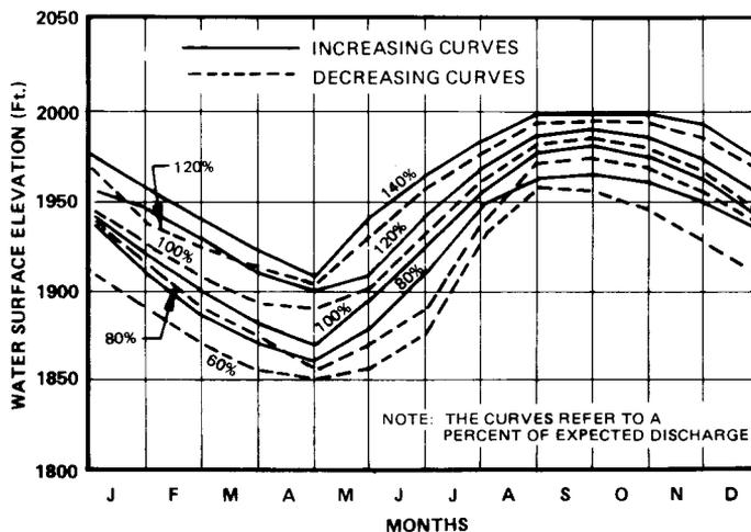
Figure 6. Operation Guide For Watana Operation, Year 2004
