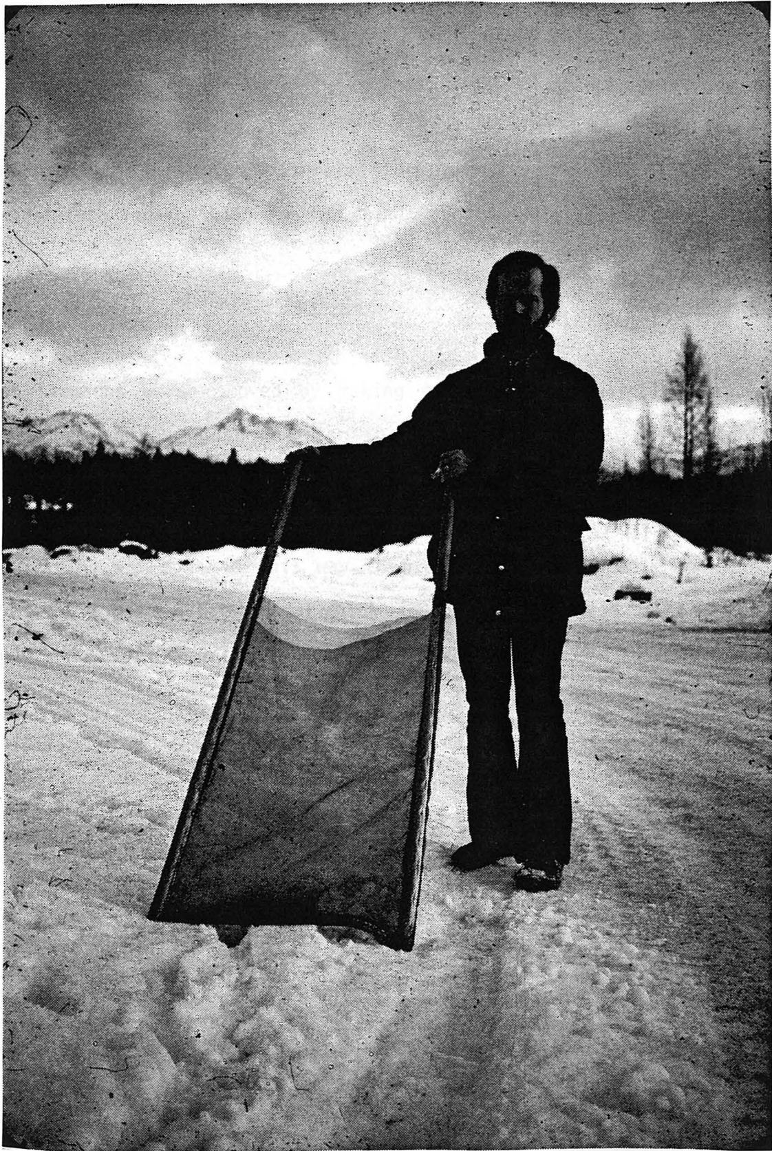
Plate 3-2-11, Kick screen used for sampling invertebrates.
