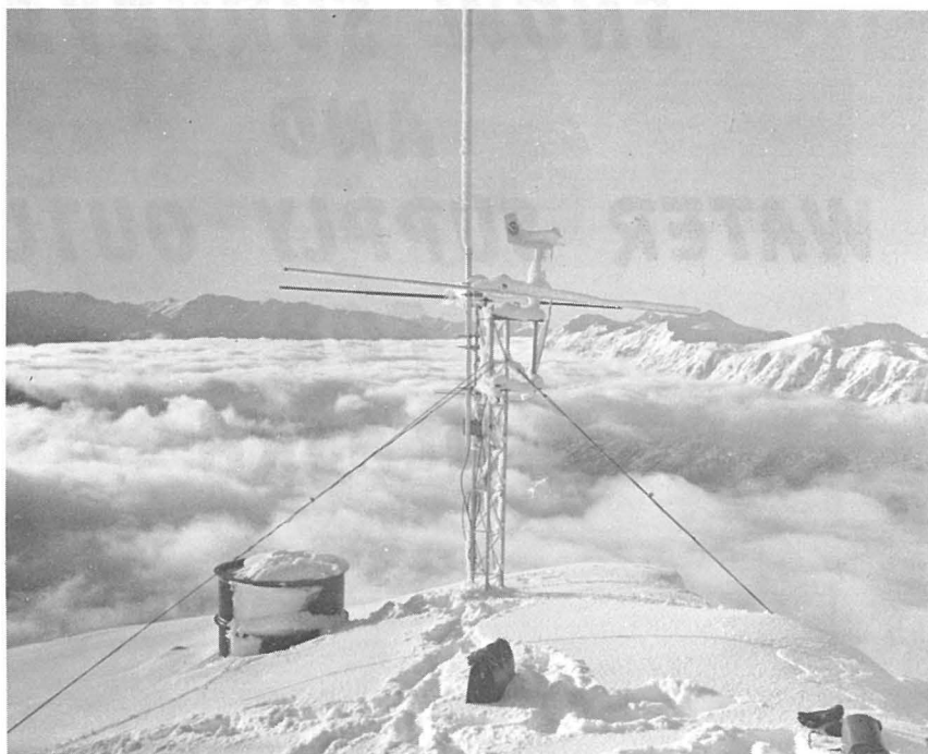
WIND DATA IS RADIO TELEMETERED FROM MAX'S MTN. AT GIRDWOOD FOR AVALANCHE CONTROL WORK
