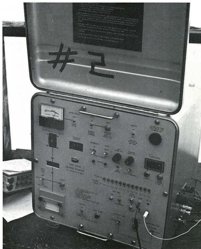
The solar panel (above left) being rotated into the sun; (above right) the sonar fish counter is powered by the solar panel.
