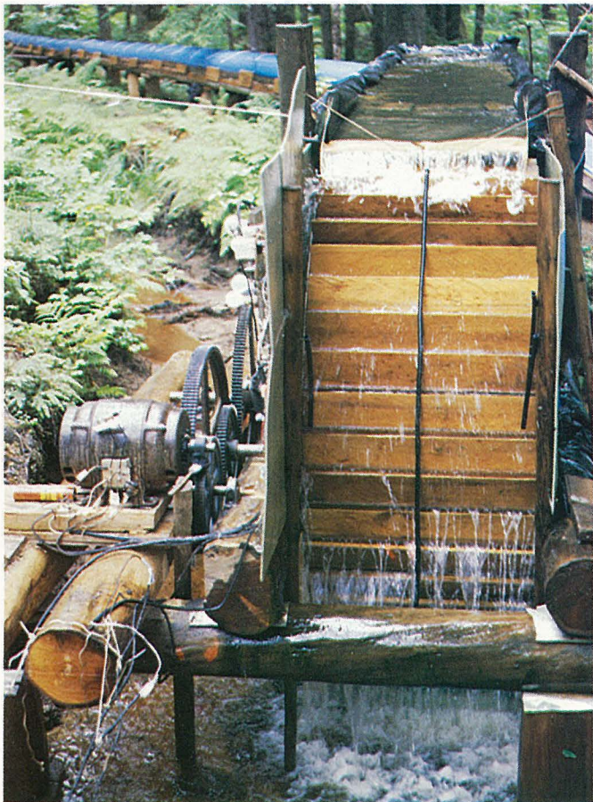
Plate 5 An overshot wheel built by Robert Nelson generates power at Thayer Lake (left). A collapsible pipeline transports water to wheel (top). Chester Johnson of Valdez performs the weekly greasing of his hydro turbine (above).
