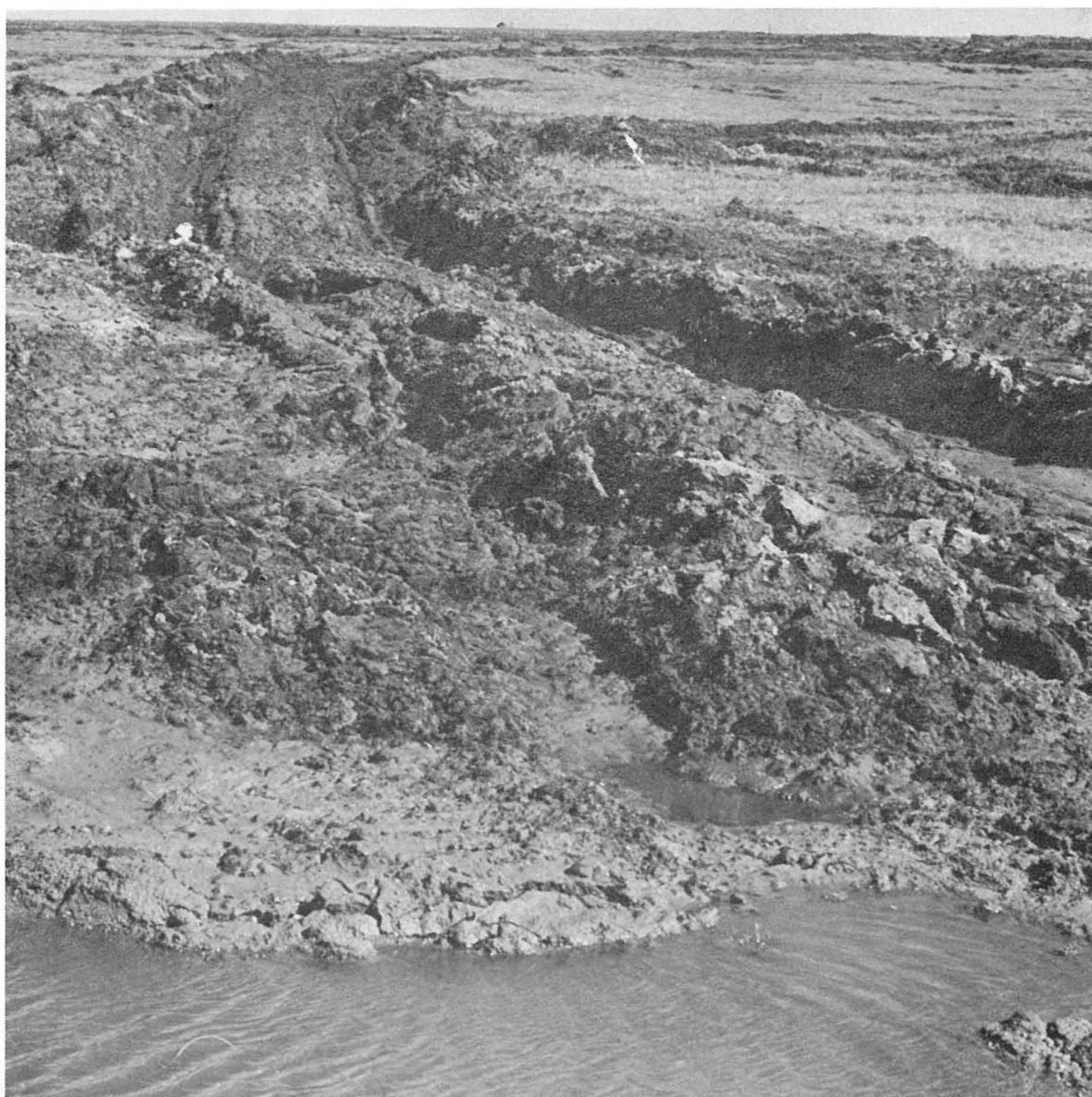
Photo 75: Result of repeated "cat" travel over thawed ground at Barrow.
