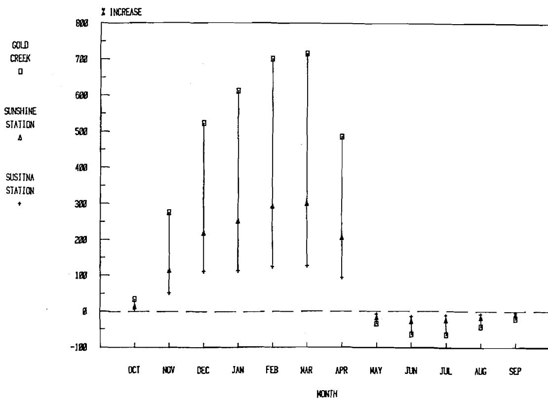
change in postproject flows over preproject flows for Gold Creek, Sunshine and Susitna Station mainstem locations. Patterns of skewness and kurtosis for natural and operational flows were similar in this case to those in the single-dam case. Consequently, testing for river reaches with significant flow differences was not pursued. Flow profiles of natural and two-dam operational conditions are shown in Appendix E.
