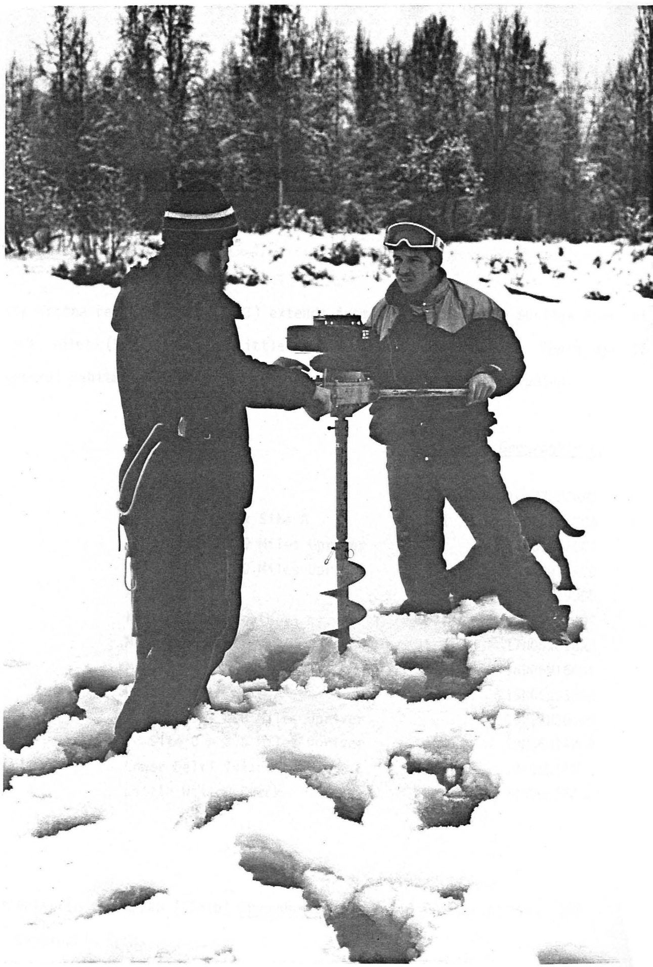
Plate 5. Use of an ice auger for winter sampling.
