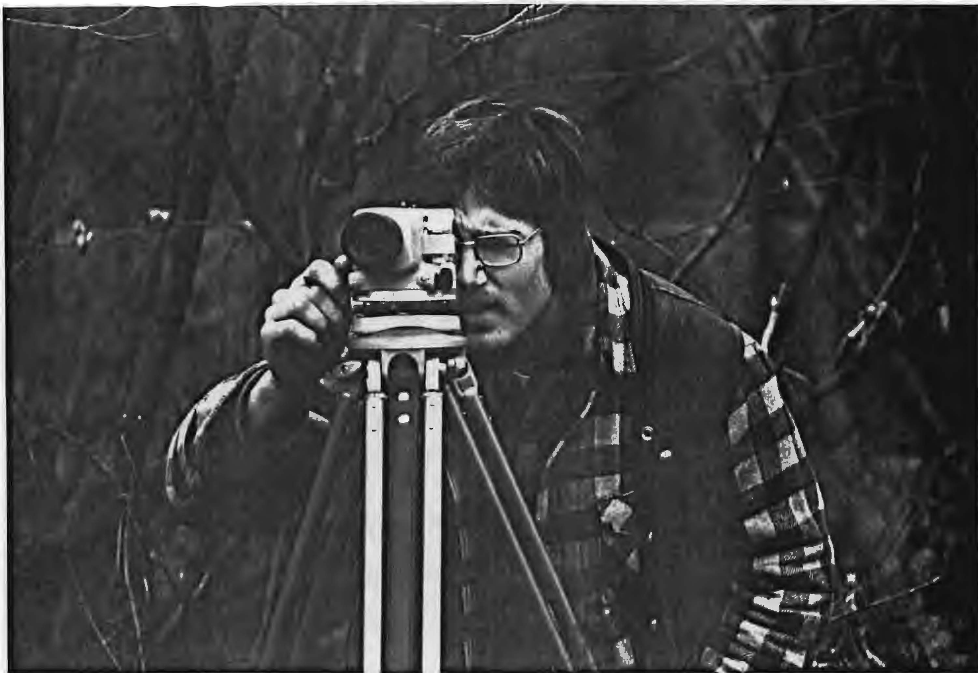
Plate 8. Use of a Leitz B-2 survey level for surveying in the selected habitat study sloughs.
