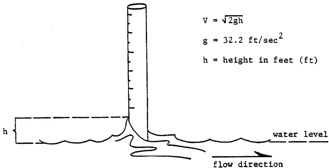
Figure 8. The relationship between height (h) and mean reach velocity as depicted by the rise of the water column against a staff held perpendicular to the flow.
