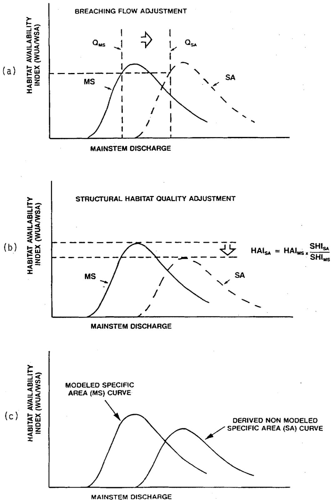
Figure 12. Derivation of a HAI versus discharge curve for a nonmodeled specific area (SA) from the representative curve of a modeled specific area (MS) showing: (a) breaching flow adjustment; (b) structural habitat quality adjustment; and (c) the derived curve.
