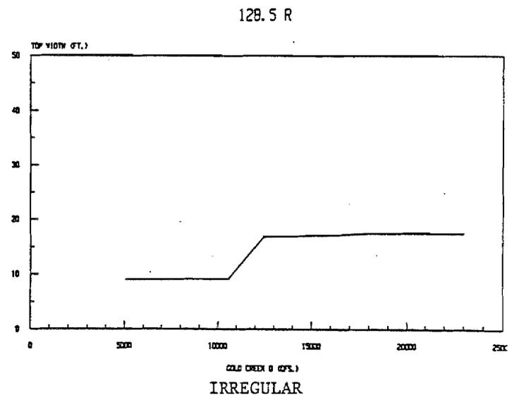
Figure 11. Representative wetted top width versus discharge plots for each category of curve slope.
