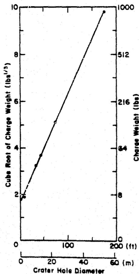
Figure 3-2. Relationship of explosive weight to crater hole (good for ice 1 to 10 feet thick).
