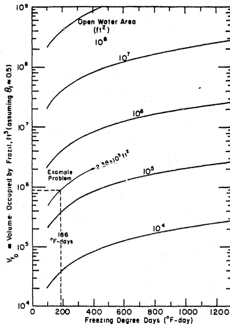
Figure 2-2. Frazil ice accumulation as a function of degree-days.
