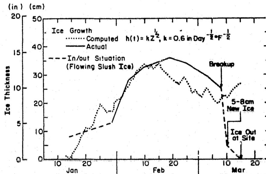
Figure 2-4. Actual measured ice thickness vs. computed growth at Shelburne Point, Vermont: Winter 1975-76.
