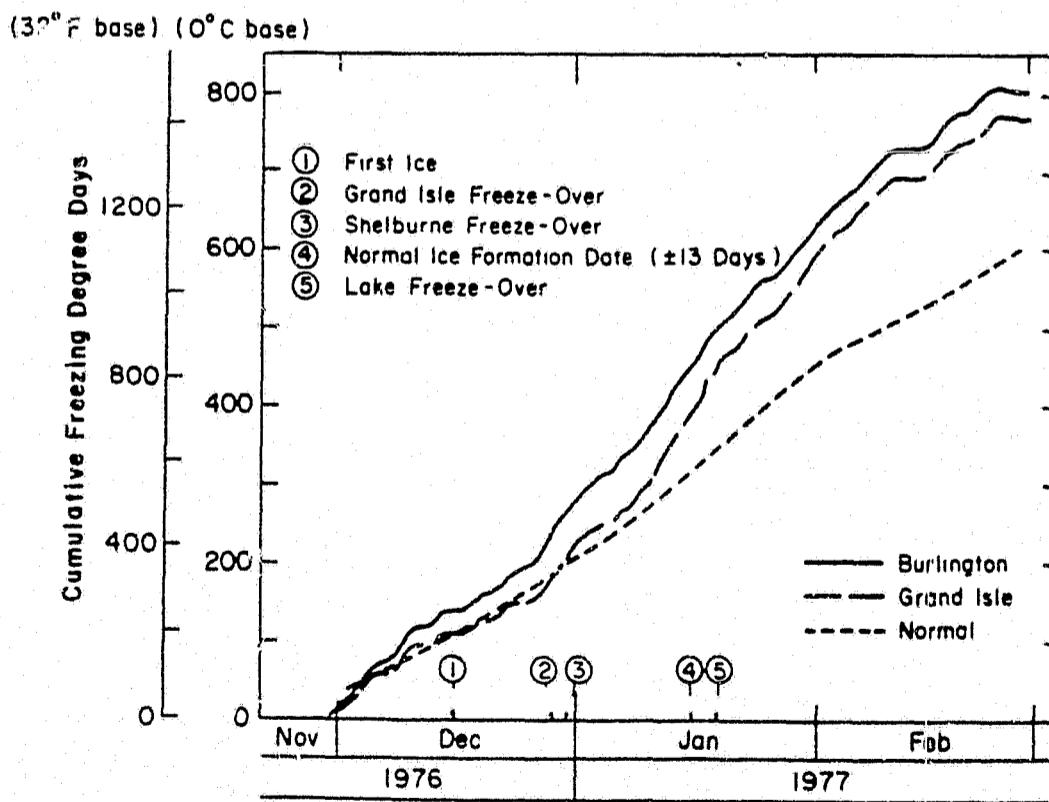
Figure 2-3. Accumulated freezing degree-days at two sites:
