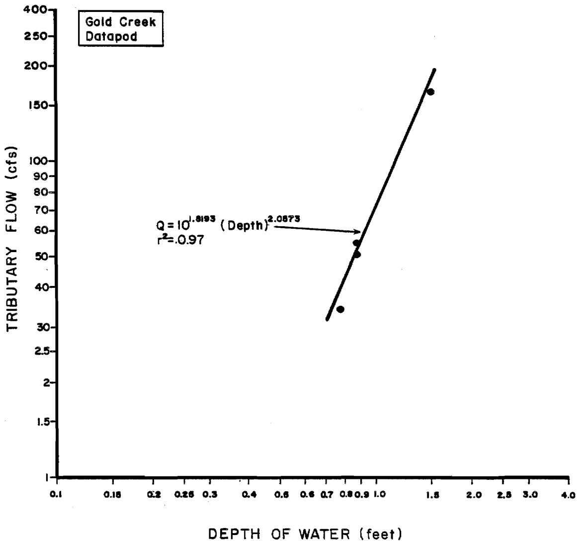
Figure 1-65. Depth of Water (feet) versus tributary flow rating curve for Gold Creek continuous stage recorder.
