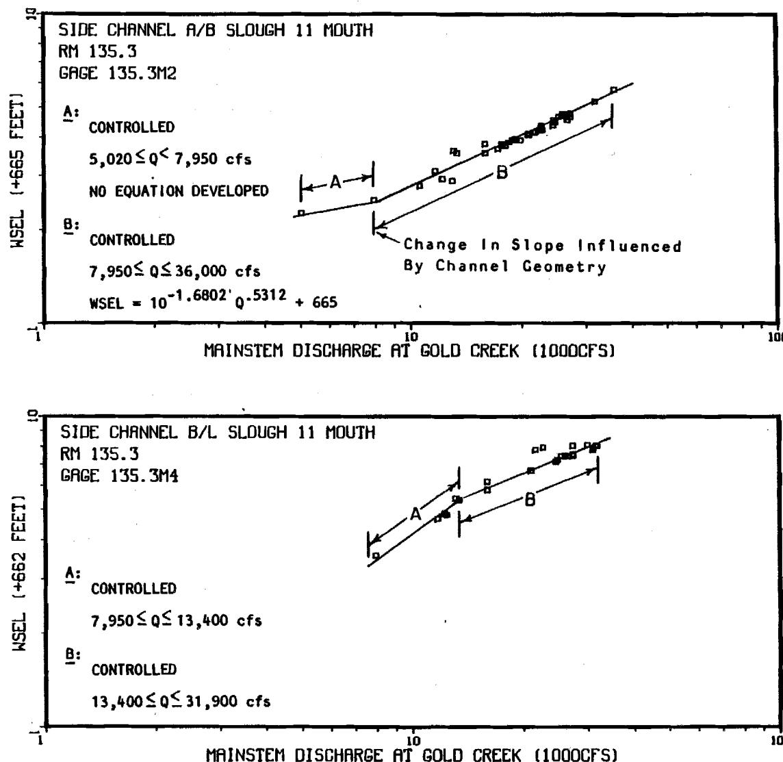
Appendix Figure 1-A-41 Non-Mainstem discharge (Provisional USGS 1983) versus the water surface elevation at Side Channel below Slough 11 mouth and Side Channel above Slough 11 mouth.
