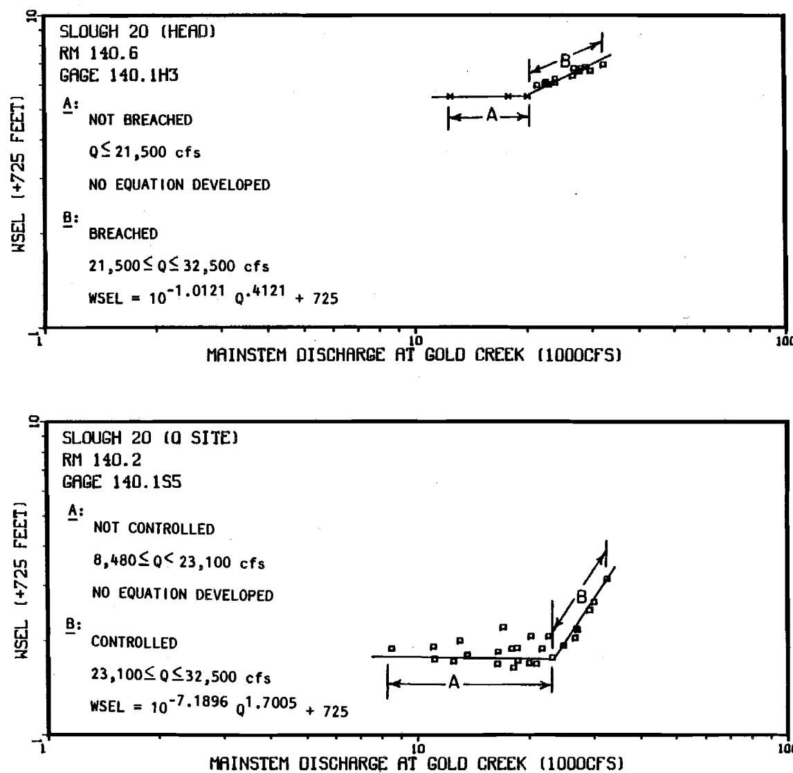
Appendix Figure 1-A-49 Non-Mainstem discharge (Provisional USGS 1983) versus the water surface elevation at Slough 20 discharge site and head.
