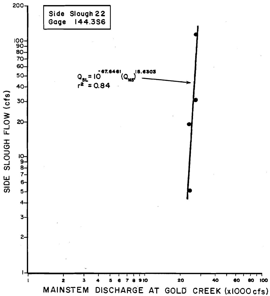
Figure 1-52. Slough flow versus mainstem discharge rating curve for Side Slough 22, staff gage 144.3S6.
