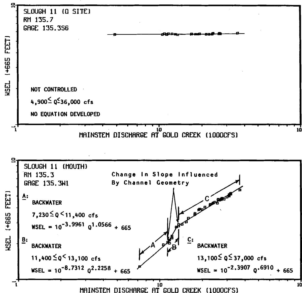
Appendix Figure 1-A-42 Non-Mainstem discharge (Provisional USGS 1983) versus the water surface elevation at Slough 11 mouth and discharge site.
