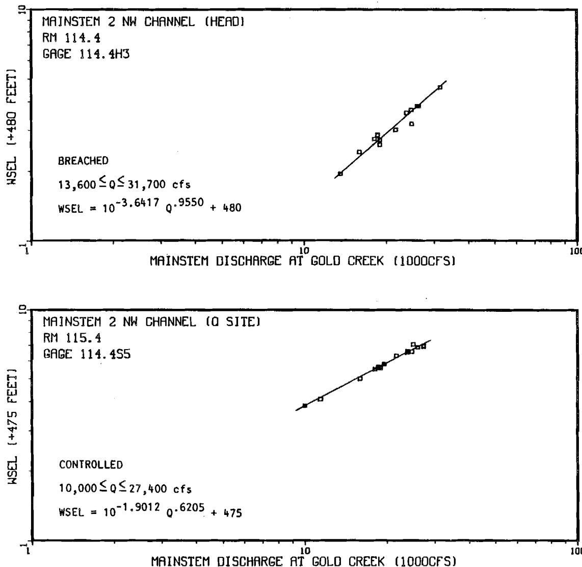
Figure 1-A-30. Non-Mainstem discharge (Provisional USGS 1983) versus the water surface elevation at Mainstem 2 NW Channel discharge site and head.
