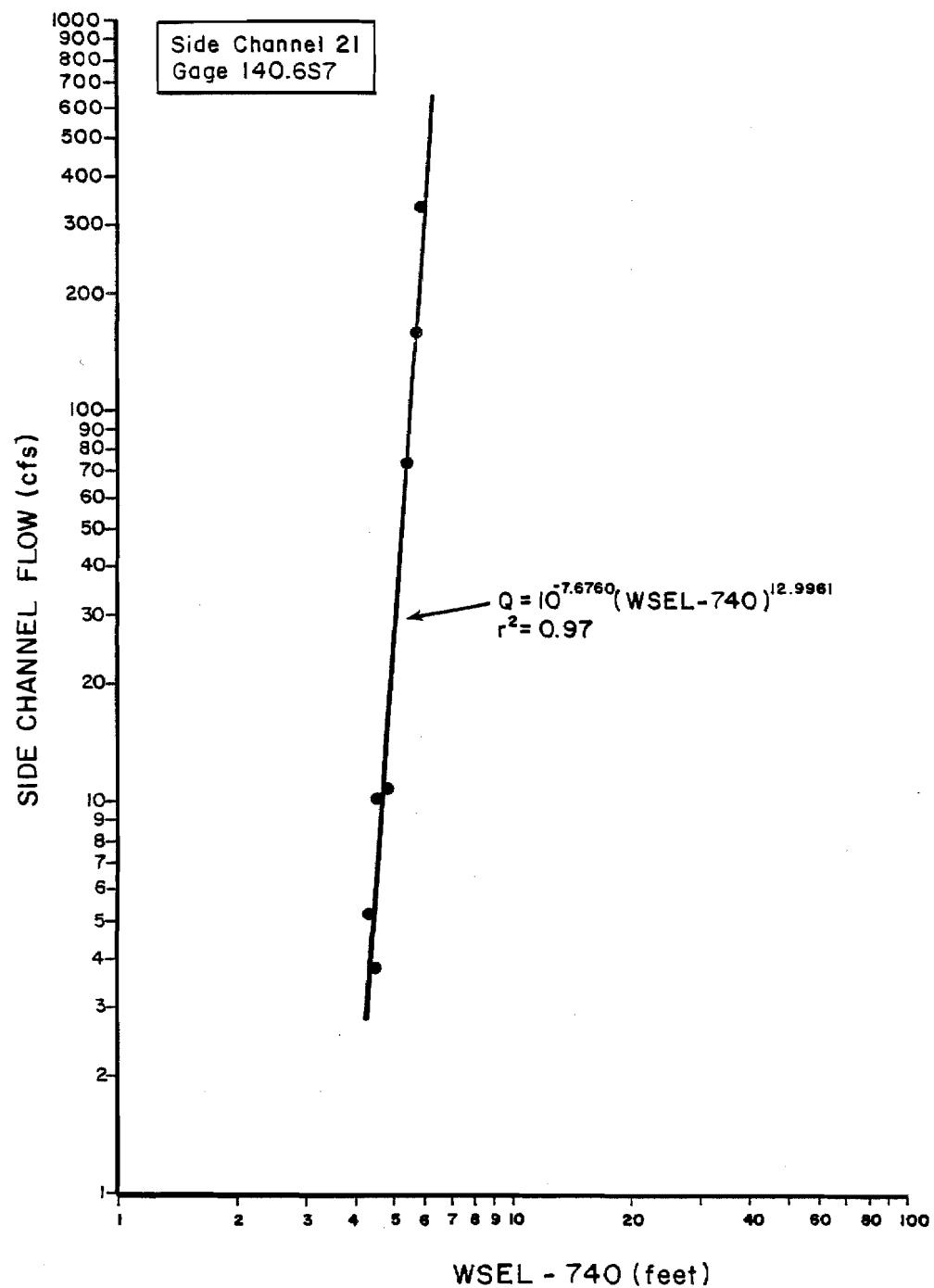
Figure 1-22. Stage versus flow rating curve for Side Channel 21, staff gage 140.6S7.
