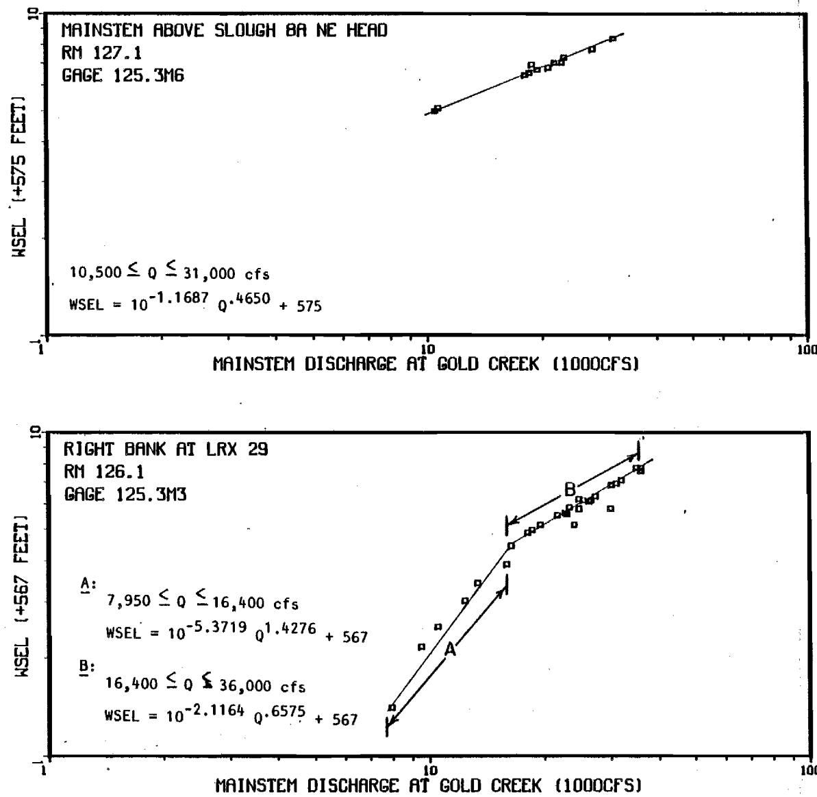
Appendix Figure 1-A-11. Mainstem discharge (Provisional USGS 1983) versus mainstem water surface elevation at the right bank at LRX 29 and above Slough 8A NE head.
