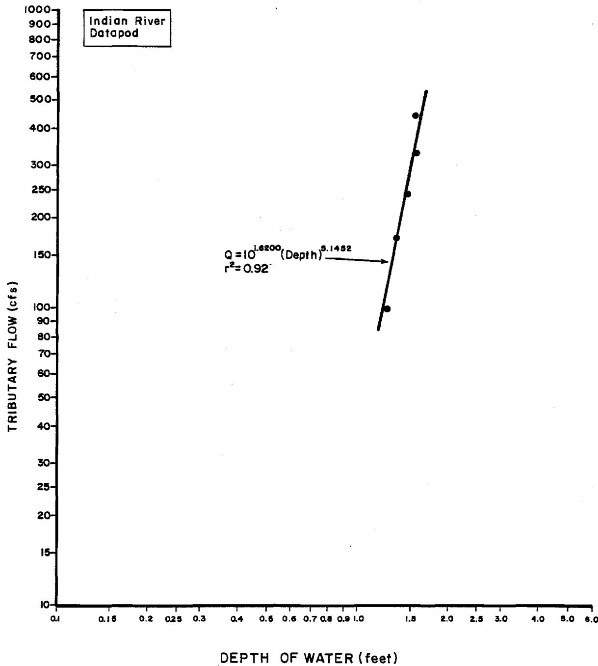
Figure 1-67. Depth of water (feet) versus tributary flow rating curve for Indian River, continuous stage recorder.
