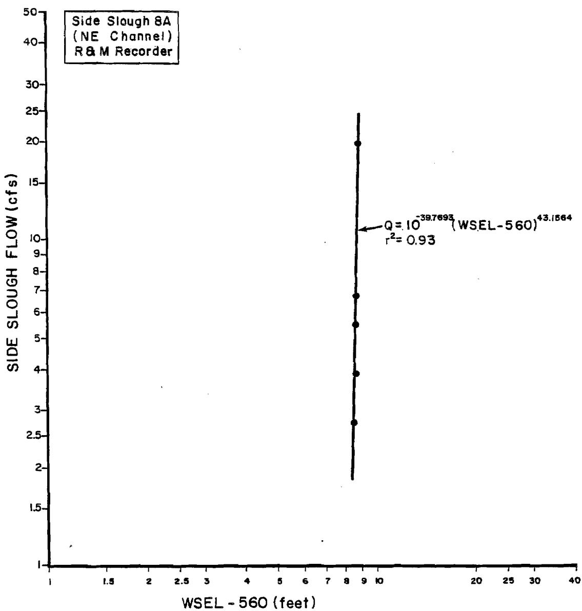
Figure 1-33. Stage versus flow rating curve for Side Slough 8A, staff gage at R&M recorder.
