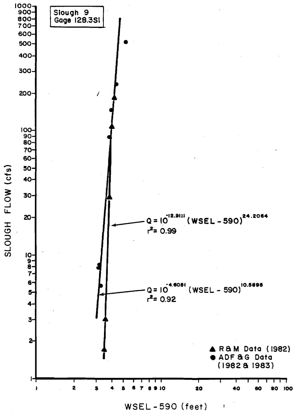
Figure 1-37. Stage versus flow rating curve for Side Slough 9, staff gage 128.3S1.
