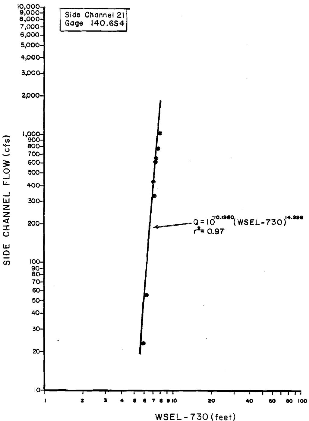
Figure 1-21. Stage versus flow rating curve for Side Channel 21, staff gage 140.6S4.
