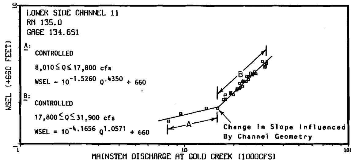
Appendix Figure 1-A-40. Non-Mainstem discharge (Provisional USGS 1983) versus the water surface elevation at Lower Side Channel 11 physical habitat modeling cross-sections 1 and 3 (staff gages 134.6S1 and 134.6S2).
