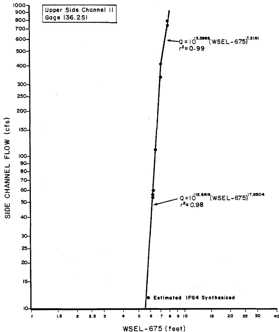
Figure 1-18. Stage versus flow rating curve for Upper Side Channel 11, staff gage 136.2S1.
