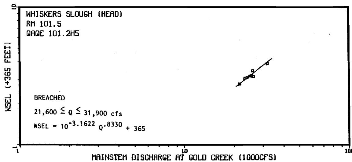
Appendix Figure 1-A-25 Non-Mainstem discharge (Provisional USGS 1983) versus the water surface elevation at Whiskers Slough head.
