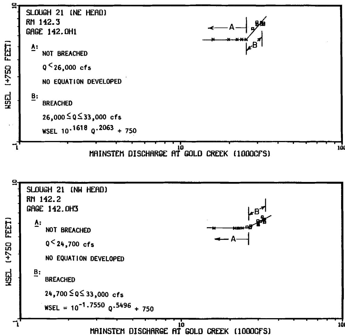
Appendix Figure 1-A-54 Non-Mainstem discharge (Provisional USGS 1983) versus the water surface elevation at Slough 21 NW head and NE head.
