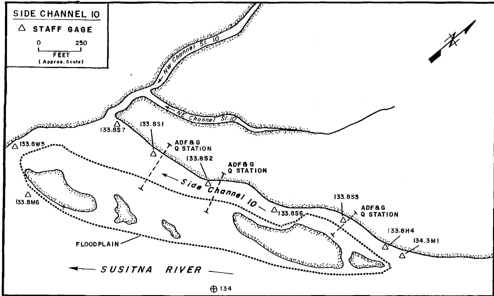
Figure 1-11. Site map of Side Channel 10, which is located on the west bank of the Susitna River at river mile 133.8.
