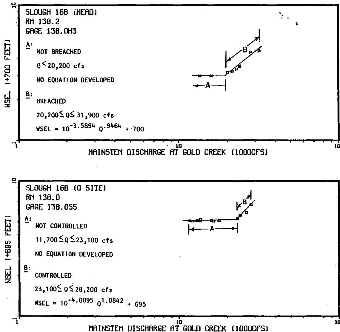
Appendix Figure 1-A-46 Non-Mainstem discharge (Provisional USGS 1983) versus the water surface elevation at Slough 16B discharge site and head.
