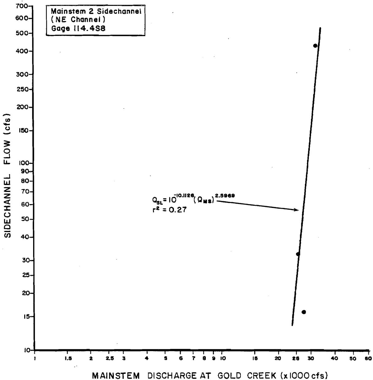
Figure 1-10. Side Channel flow versus mainstem discharge rating curve for Mainstem 2 (N.E. Channel), staff gage 114.4S8.
