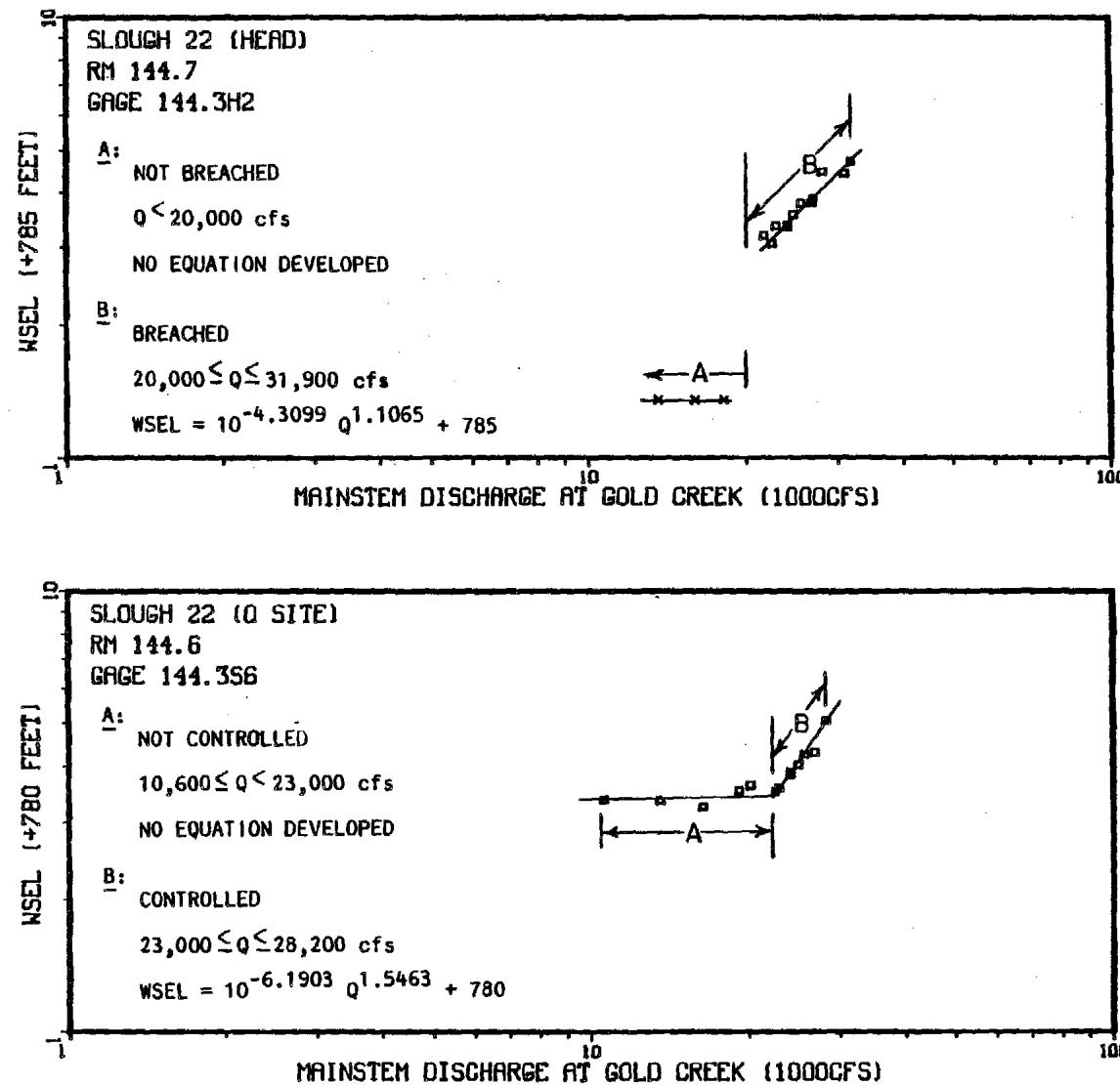
Appendix Figure 1-A-56 Non-Mainstem discharge (Provisional USGS 1983) versus the water surface elevation at Slough 22 discharge site and head.
