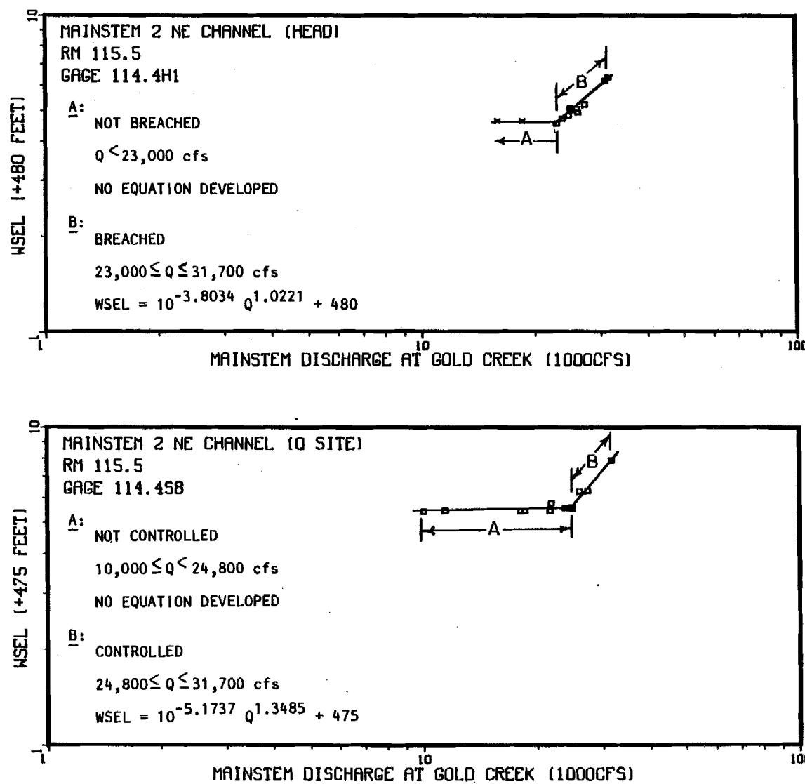
Appendix Figure 1-A-31 Non-Mainstem discharge (Provisional USGS 1983) versus the water surface elevation at Mainstem 2 NE Channel discharge site and head.
