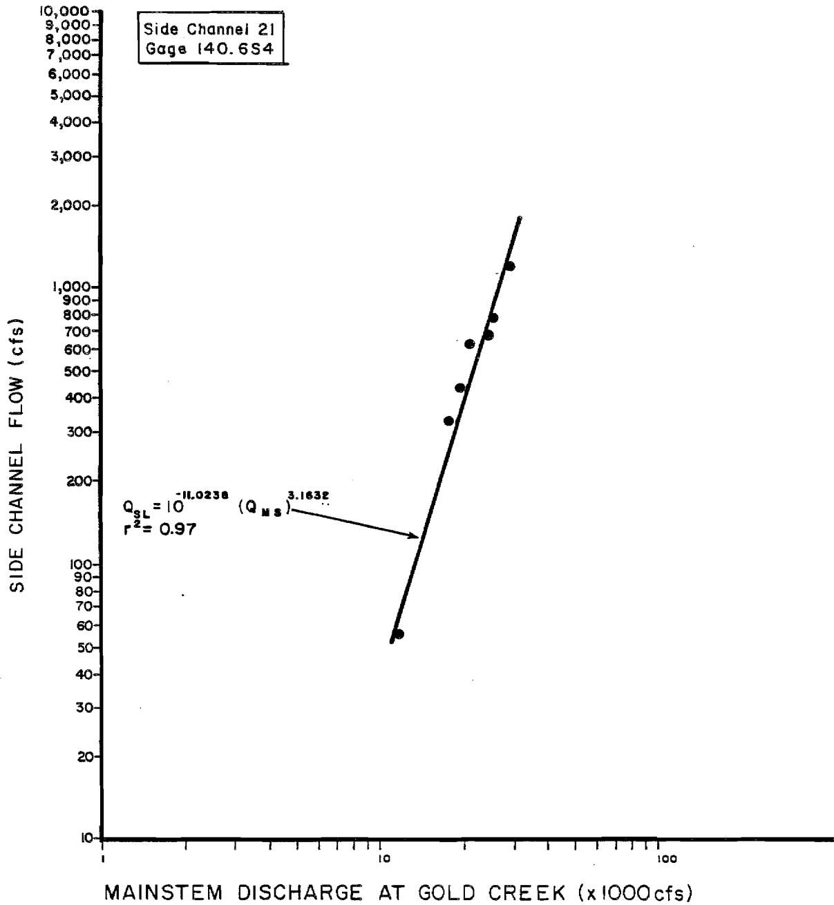
Figure 1-23. Side Channel flow versus mainstem discharge rating curve for Side Channel 21, staff gage 140.6S4.
