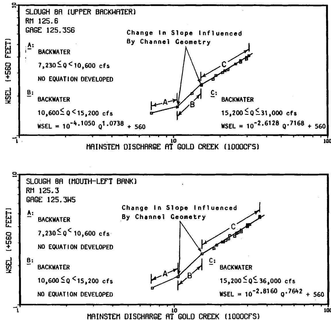
Appendix Figure 1-A-32 Non-Mainstem discharge (Provisional USGS 1983) versus the water surface elevation at Slough 8A mouth and upper backwater.
