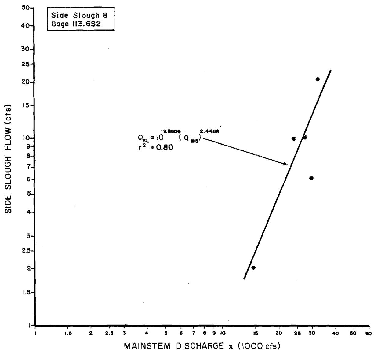
Figure 1-29. Slough flow versus mainstem discharge rating curve for Side Slough 8, staff gage 113.6S2.
