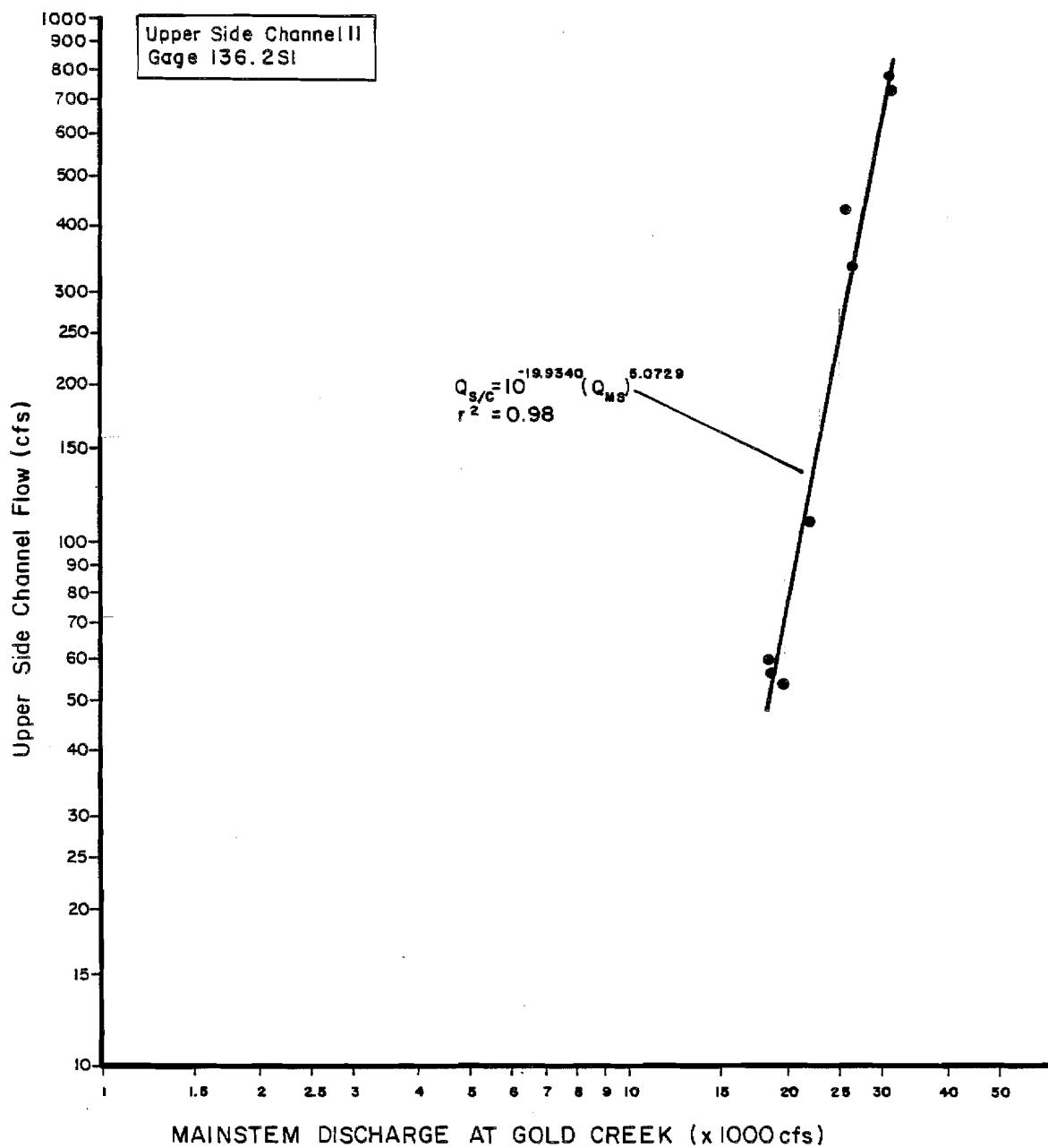
Figure 1-19. Side Channel flow versus mainstem discharge rating curve for Upper Side Channel 11, staff gage 136.2S1.
