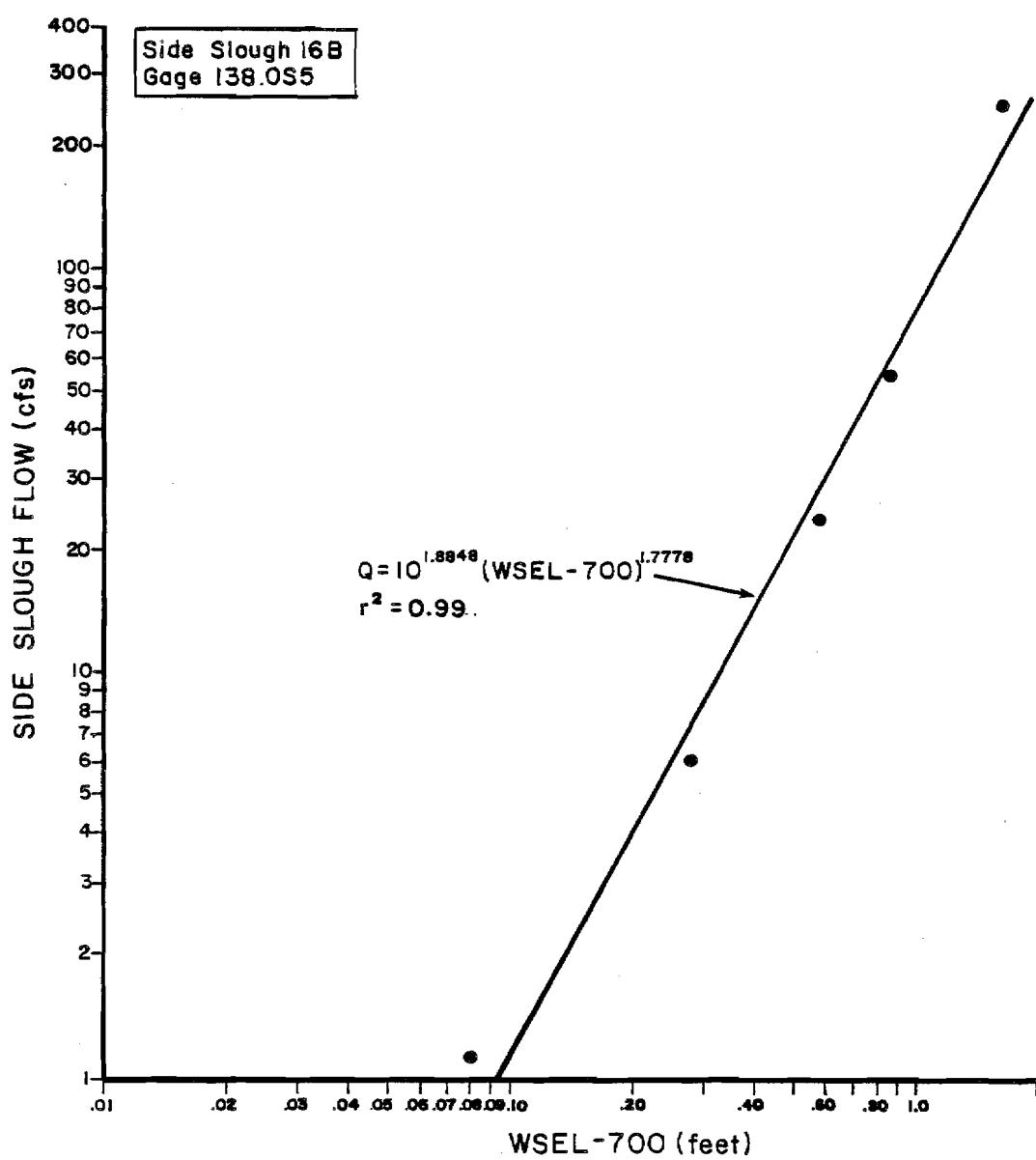
Figure 1-42. Stage versus flow rating curve for Side Slough 16B, staff gage 138.0S5.
