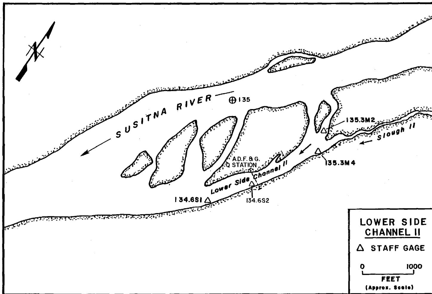
Figure 1-14. Site map of Lower Side Channel 11, which is located at the east bank of the Susitna River at river mile 134.6.
