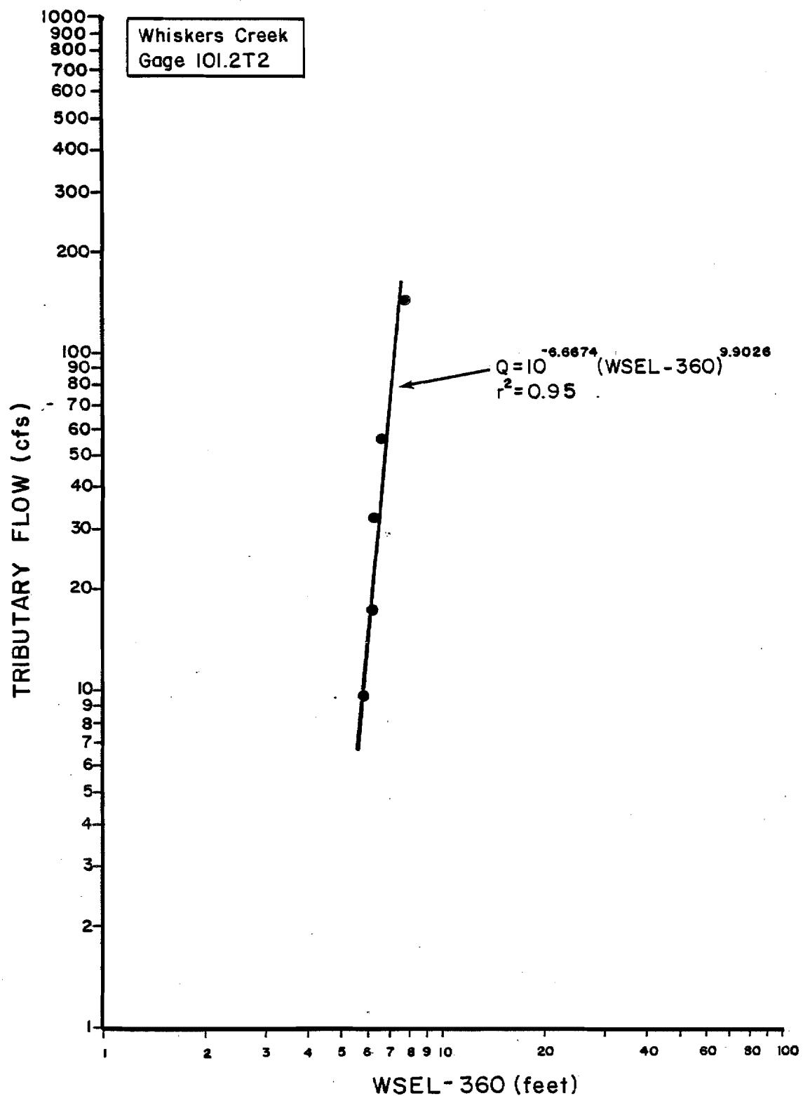
Figure 1-56. Stage versus flow rating curve for Whiskers Creek, staff gage 101.2T2.
