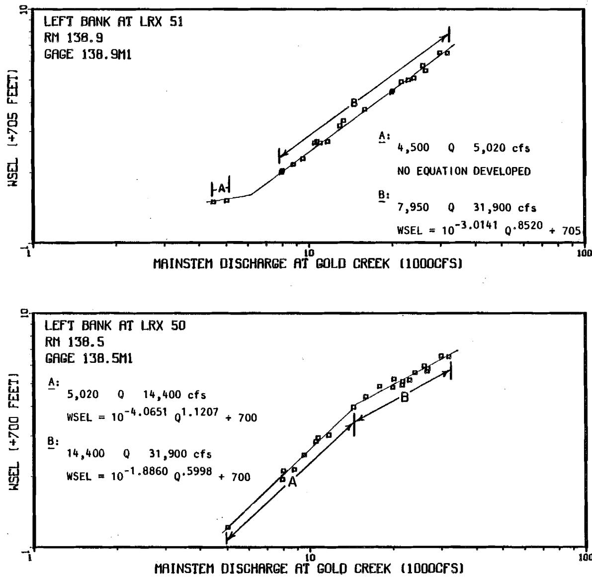
Appendix Figure 1-A-18. Mainstem discharge (Provisional USGS 1983) versus mainstem water surface elevation at the left bank at LRX 50 and the left bank LRX 51.
