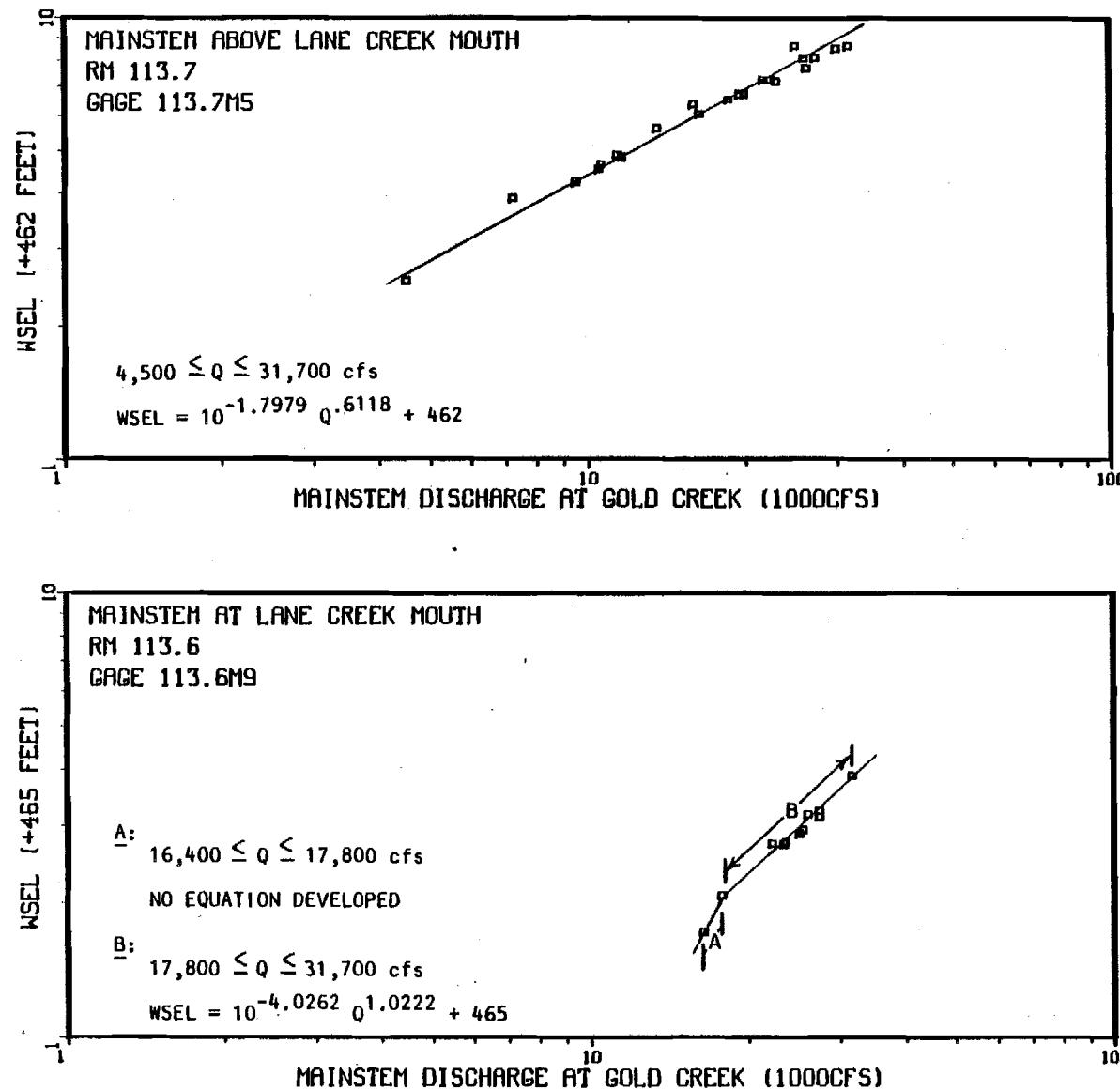
Appendix Figure 1-A-7. Mainstem discharge (Provisional USGS 1983) versus mainstem water surface elevation at Lane Creek Mouth and above Lane Creek Mouth.
