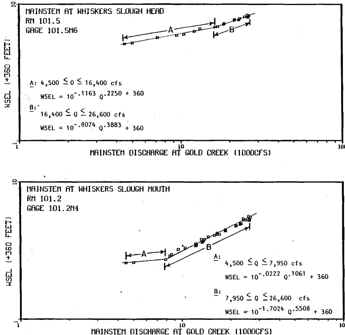
Appendix Figure 1-A-1. Mainstem discharge (Provisional USGS 1983) versus mainstem water surface elevation at Whiskers Slough head and mouth.
