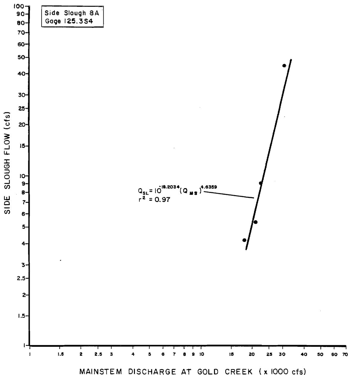
Figure 1-34. Slough flow versus mainstem discharge rating curve for Side Slough 8A, staff gage 125.3S4.
