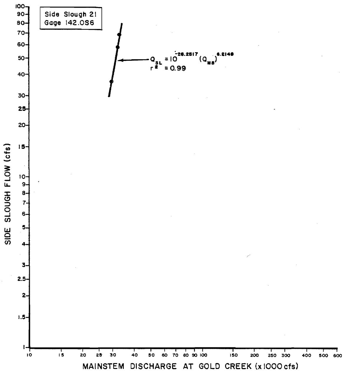
Figure 1-49. Slough flow versus mainstem discharge rating curve for Side Slough 21, staff gage 142.0S6.
