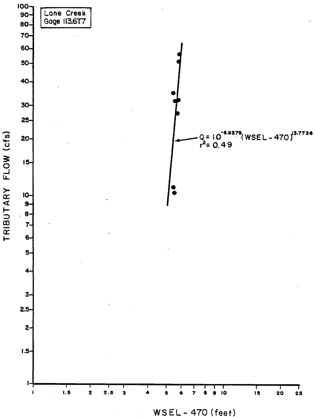
Figure 1-58. Stage versus flow rating curve for Lane Creek, staff gage 113.6T7.
