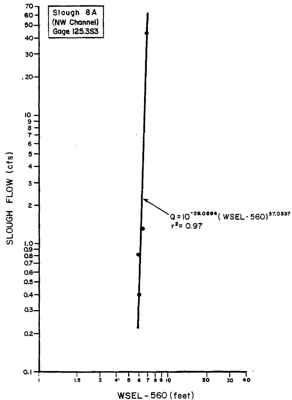
Figure 1-32. Stage versus flow rating curve for Side Slough 8A, staff gage 125.3S3.
