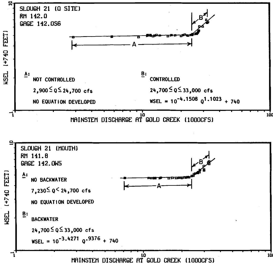
Appendix Figure 1-A-53 Non-Mainstem discharge (Provisional USGS 1983) versus the water surface elevation at Slough '21 mouth and discharge site.
