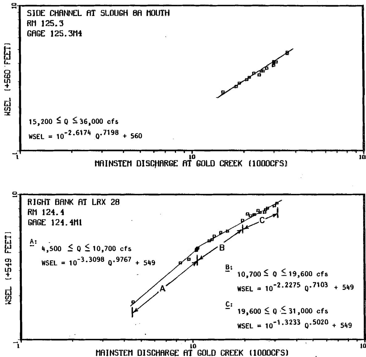
Appendix Figure 1-A-10. Mainstem (Provisional USGS 1983) versus mainstem water surface elevation at the right bank at LRX 28 and at Side Slough 8A Mouth.
