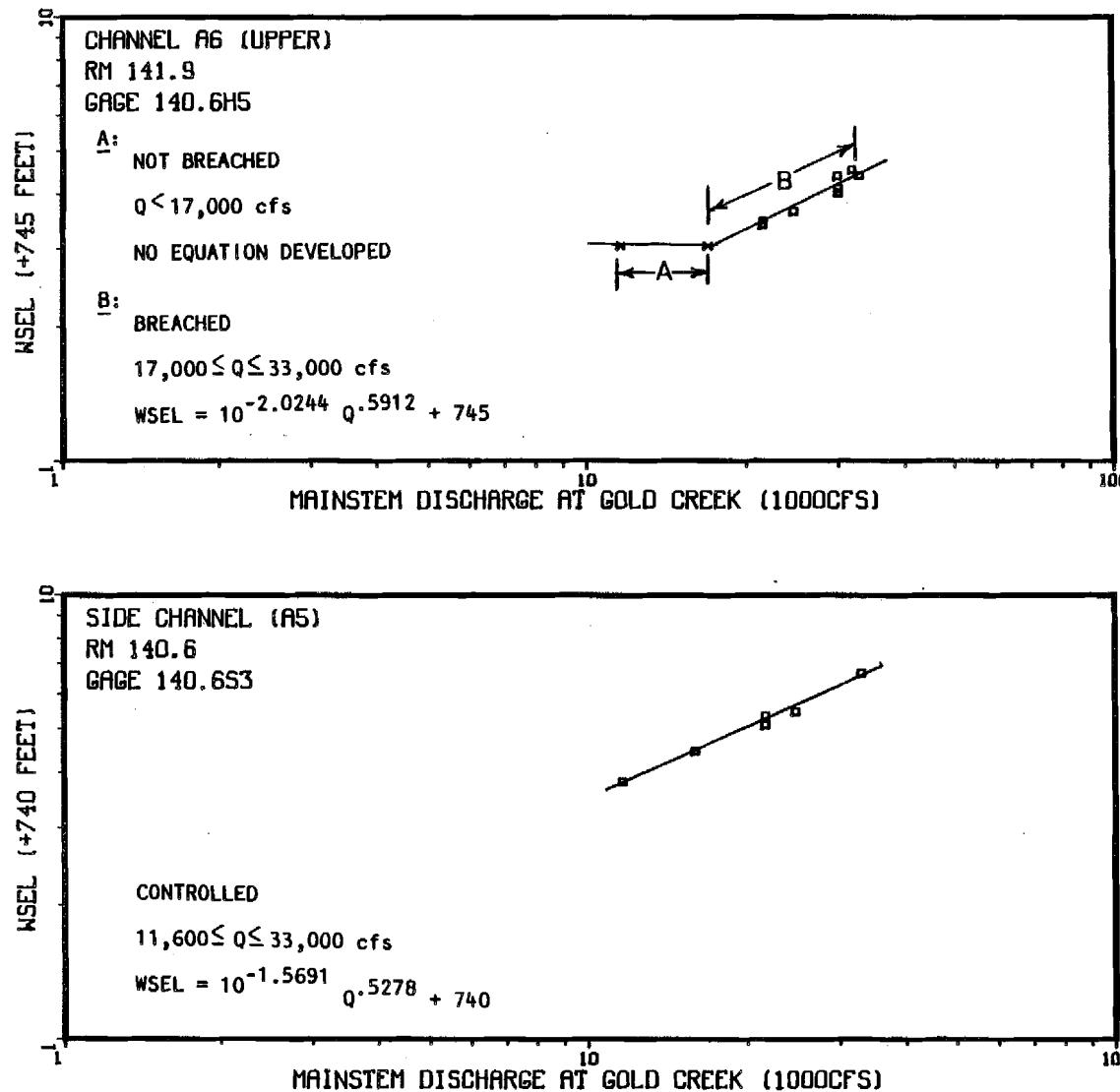
Appendix Figure 1-A-52 Non-Mainstem discharge (Provisional USGS 1983) versus the water surface elevation at Side Channels A5 and A6 Upper.
