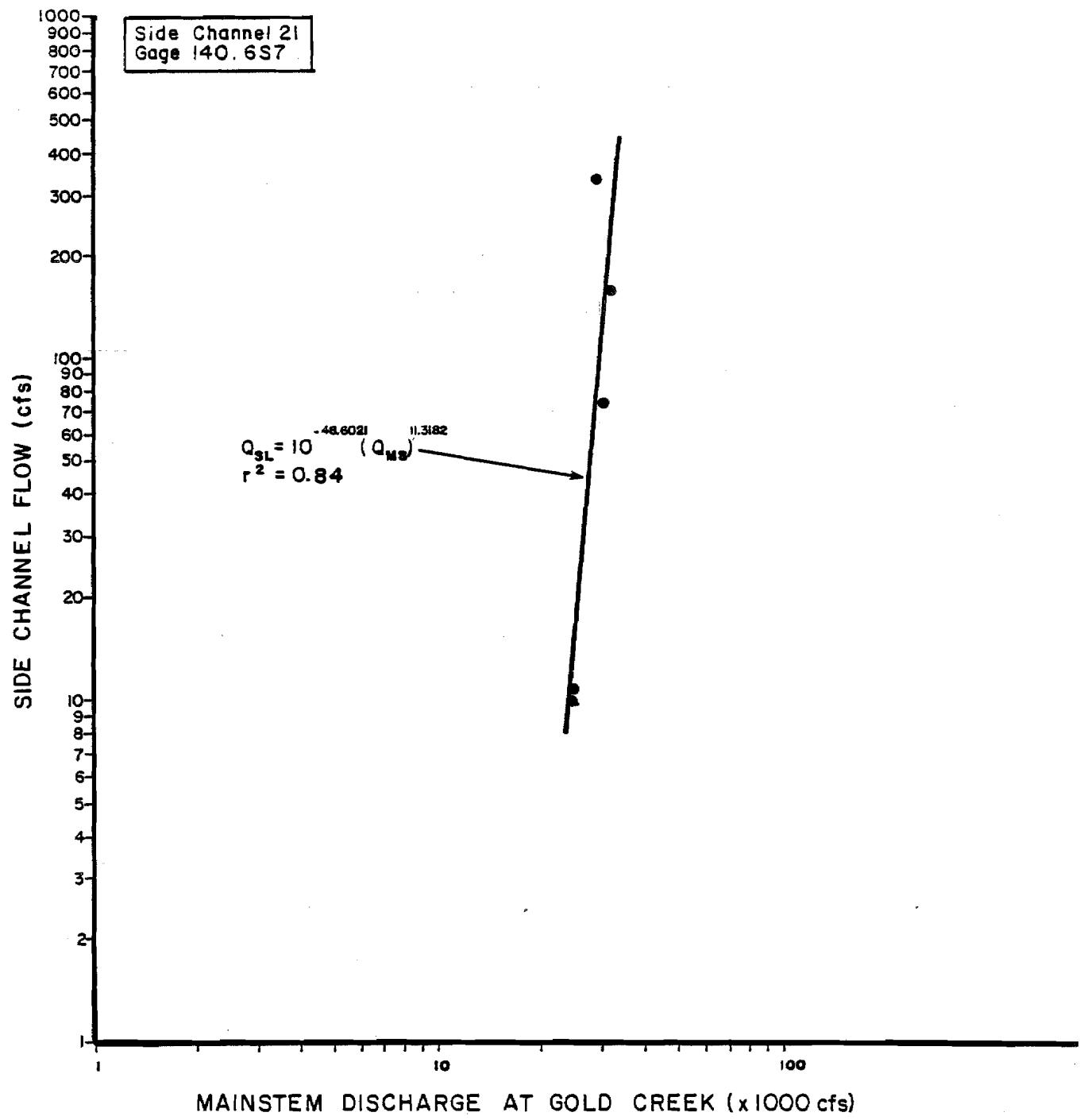
Figure 1-24. Side Channel flow versus mainstem discharge rating curve for Side Channel 21, staff gage 140.6S7.
