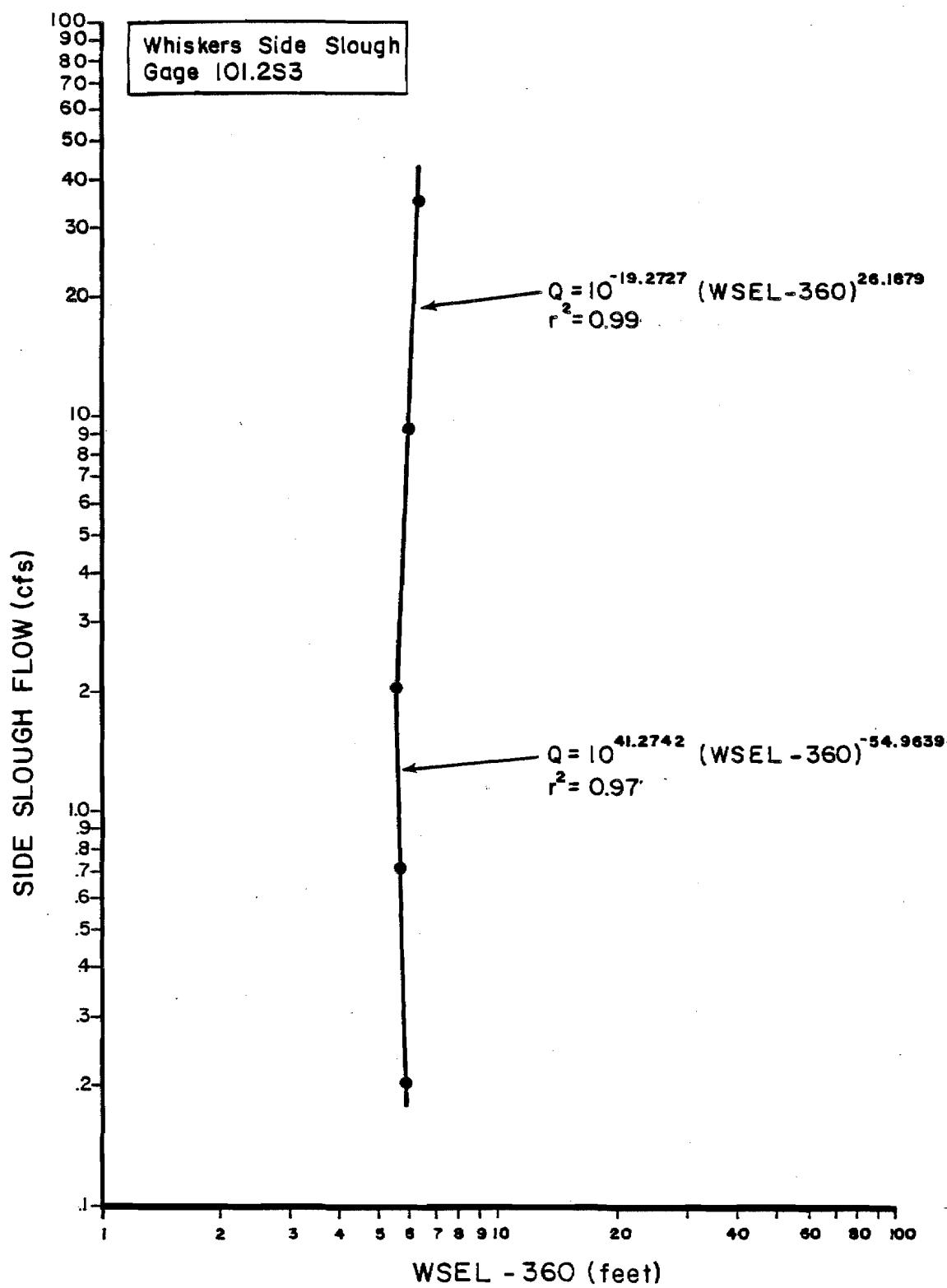
Figure 1-26. Stage versus flow rating curve for Whiskers Side Slough, staff gage 101.2S3.
