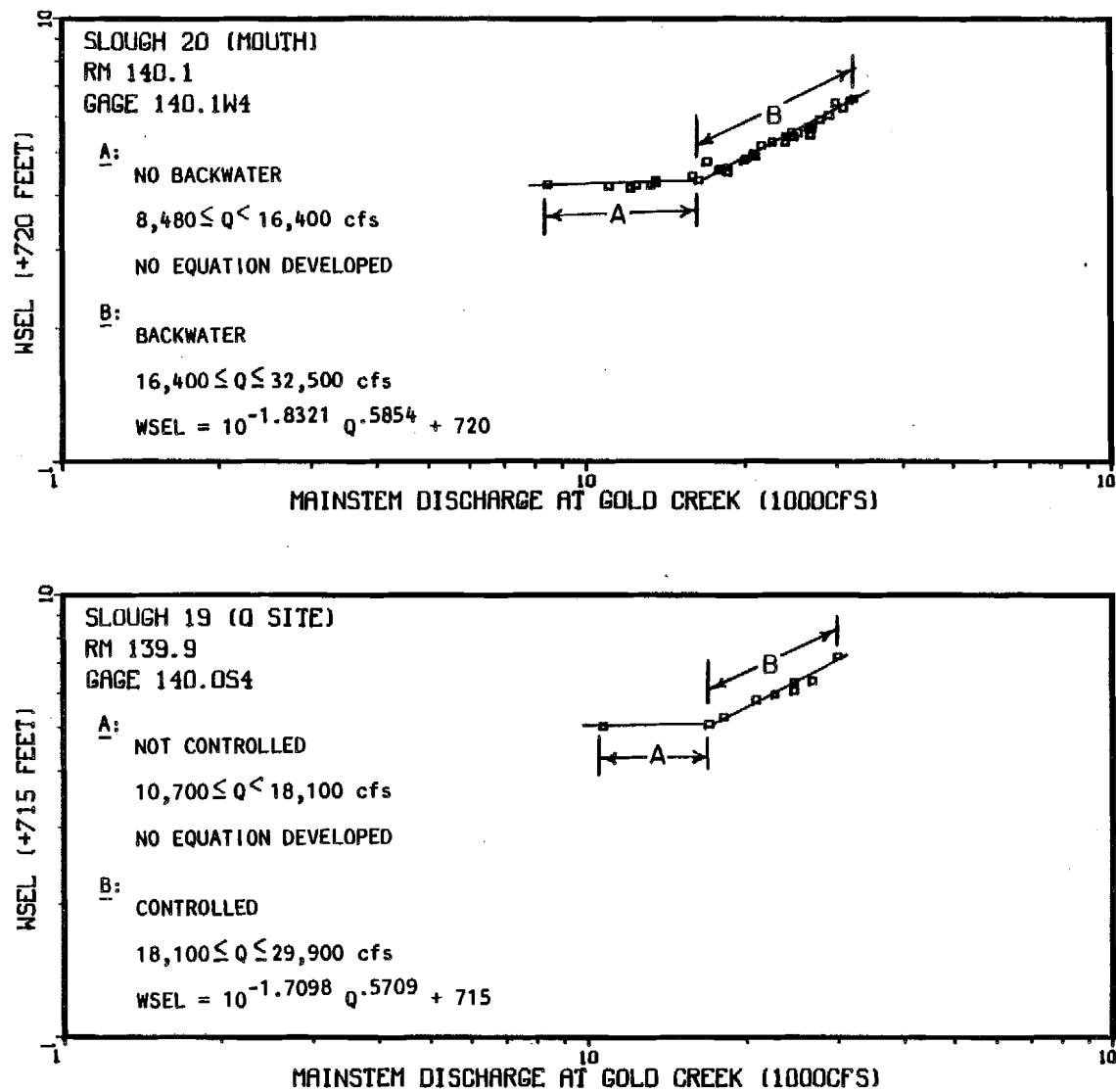
Appendix Figure 1-A-48 Non-Mainstem discharge (Provisional USGS 1983) versus the water surface elevation at Slough 19 discharge site and Slough 20 mouth.
