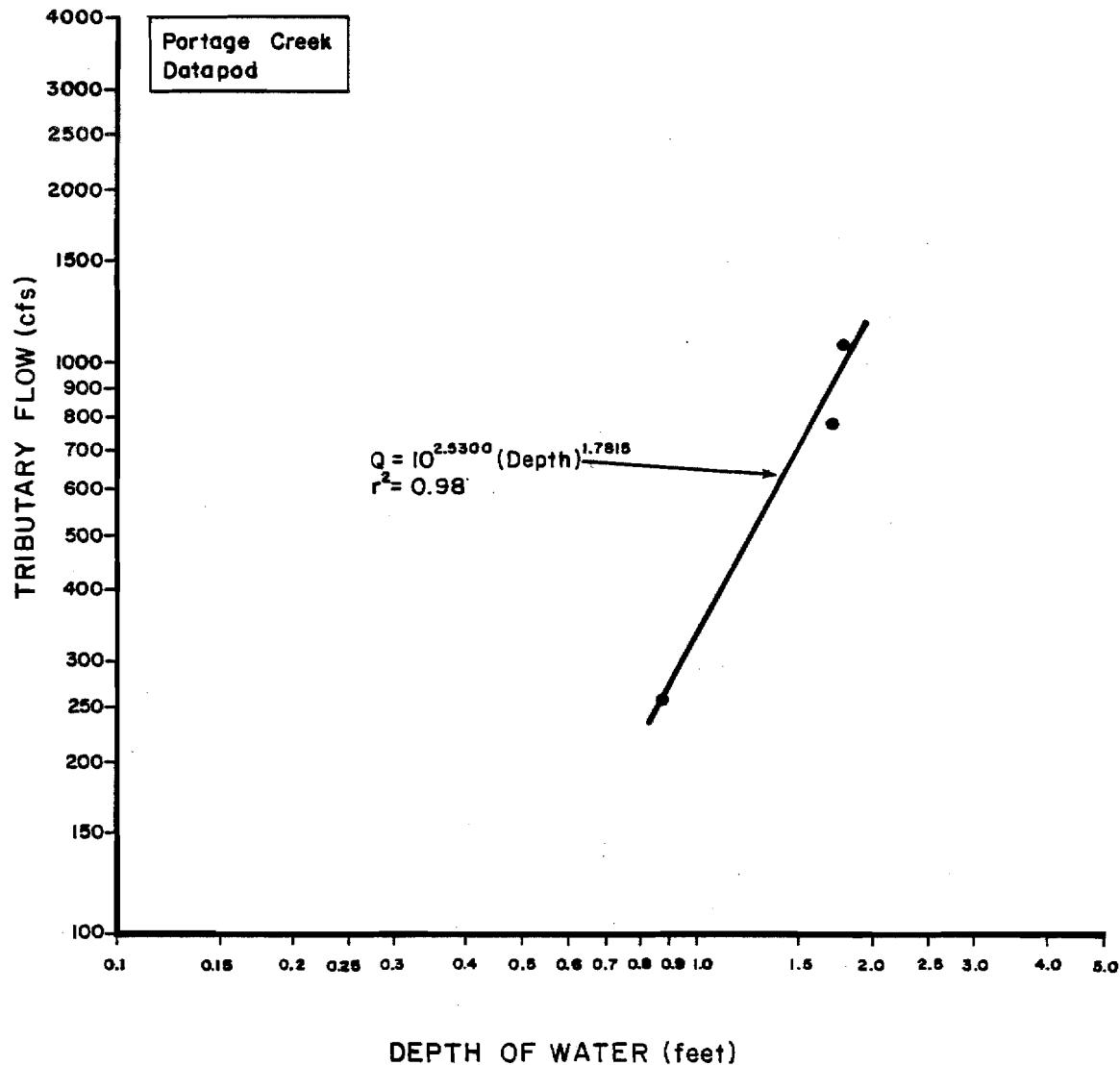
Figure 1-69. Depth of water (feet) versus tributary flow for Portage Creek, continuous stage recorder.
