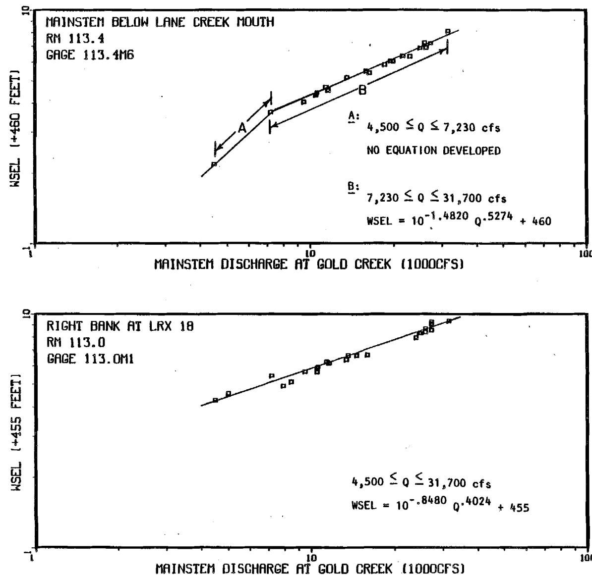
Appendix Figure 1-A-6. Mainstem discharge (Provisional USGS 1983) versus mainstem water surface elevation at right bank at LRX 18 and mainstem below Lane Creek Mouth.
