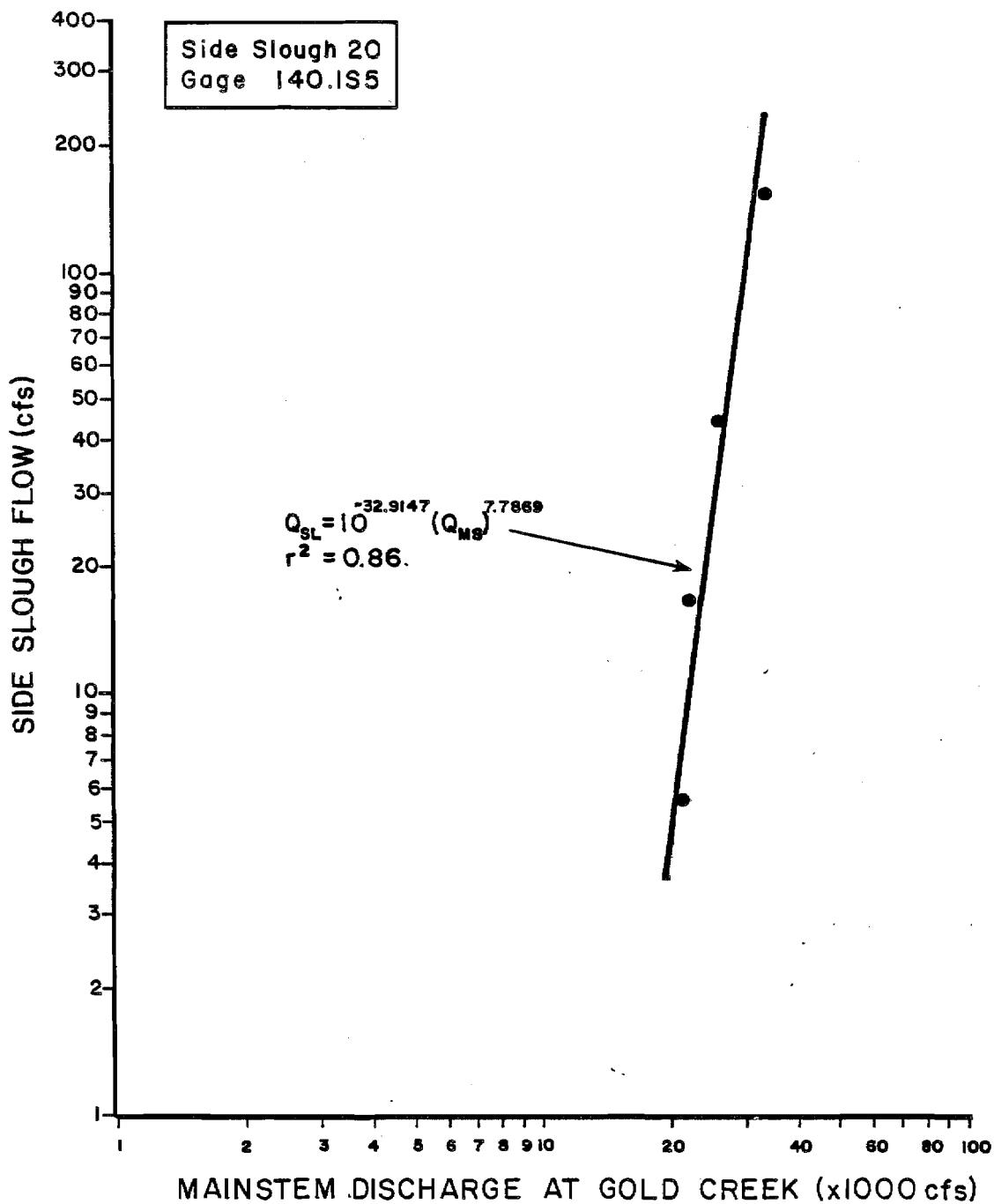
Figure 1-46. Slough flow versus mainstem discharge rating curve for Side Slough 20, staff gage 140.1S5.
