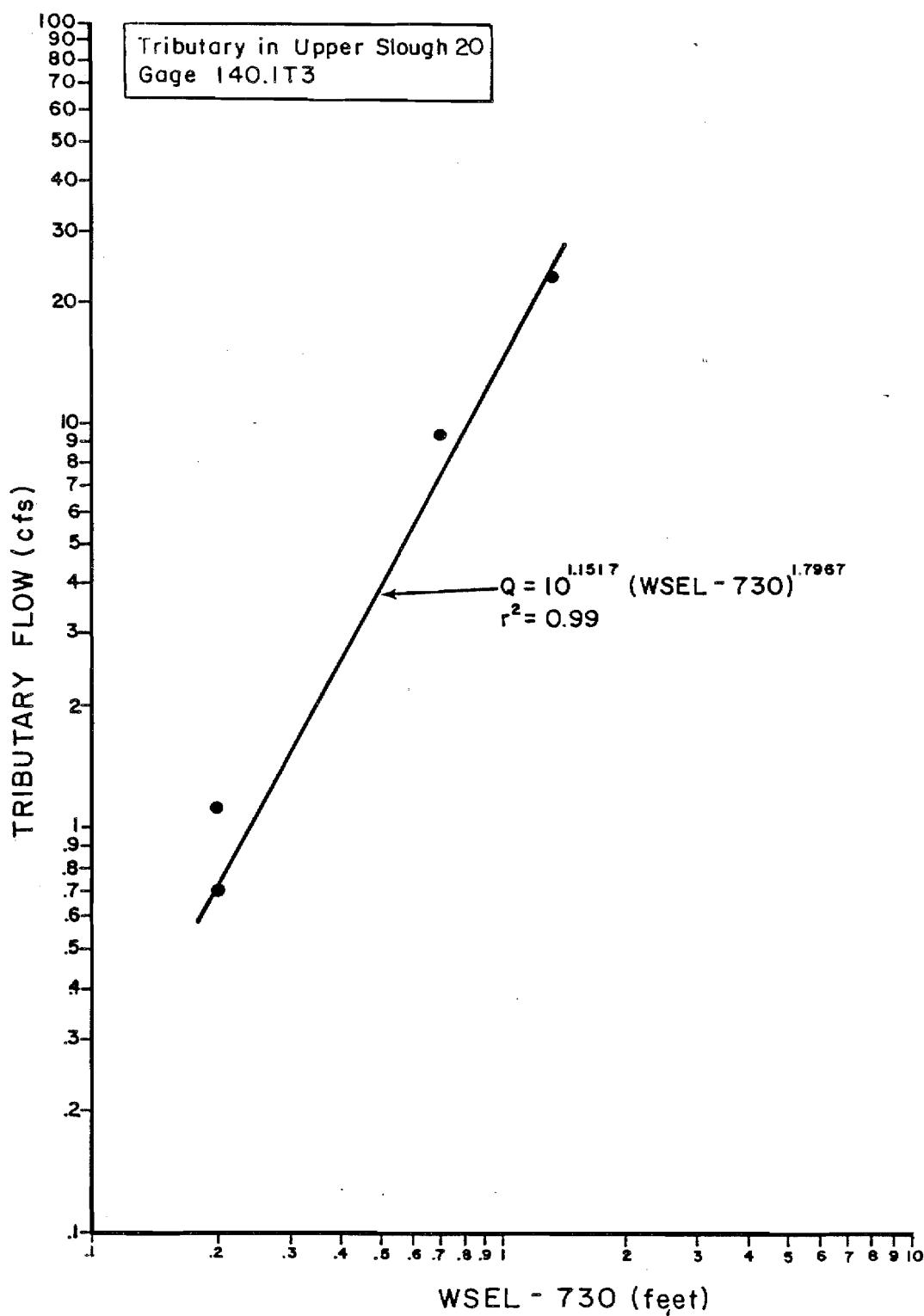
Figure 1-63. Stage versus flow rating curve for tributary in Upper Slough 20, staff gage 140.1T3.
