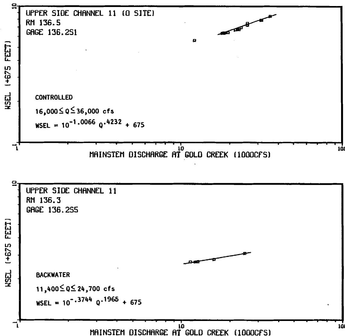
Appendix Figure 1-A-44 Non-Mainstem discharge (Provisional USGS 1983) versus the water surface elevation at Upper Side Channel 11 physical habitat modeling cross section 3 (136.2S5) and discharge site.
