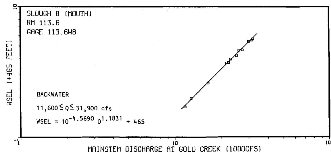
Appendix Figure 1-A-27. Non-Mainstem discharge (Provisional USGS 1983) versus the water surface elevation at Slough 8 mouth and discharge site.
