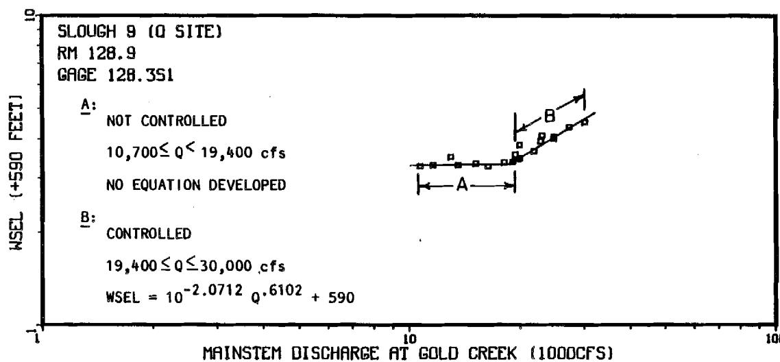
Appendix Figure 1-A-36 Non-Mainstem discharge (Provisional USGS 1983) versus the water surface elevation at Slough 9 discharge site and head.
