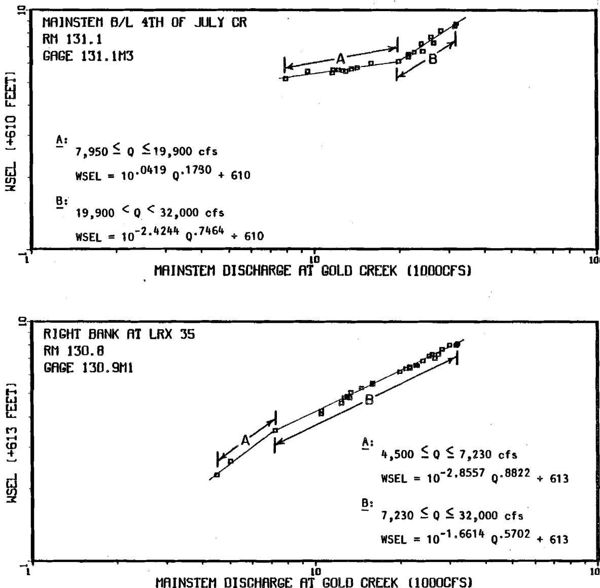
Appendix Figure 1-A-14. Mainstem discharge (Provisional USGS 1983) versus mainstem water surface elevation at the right bank at LRX 35 and below the mouth of Fourth of July Creek.
