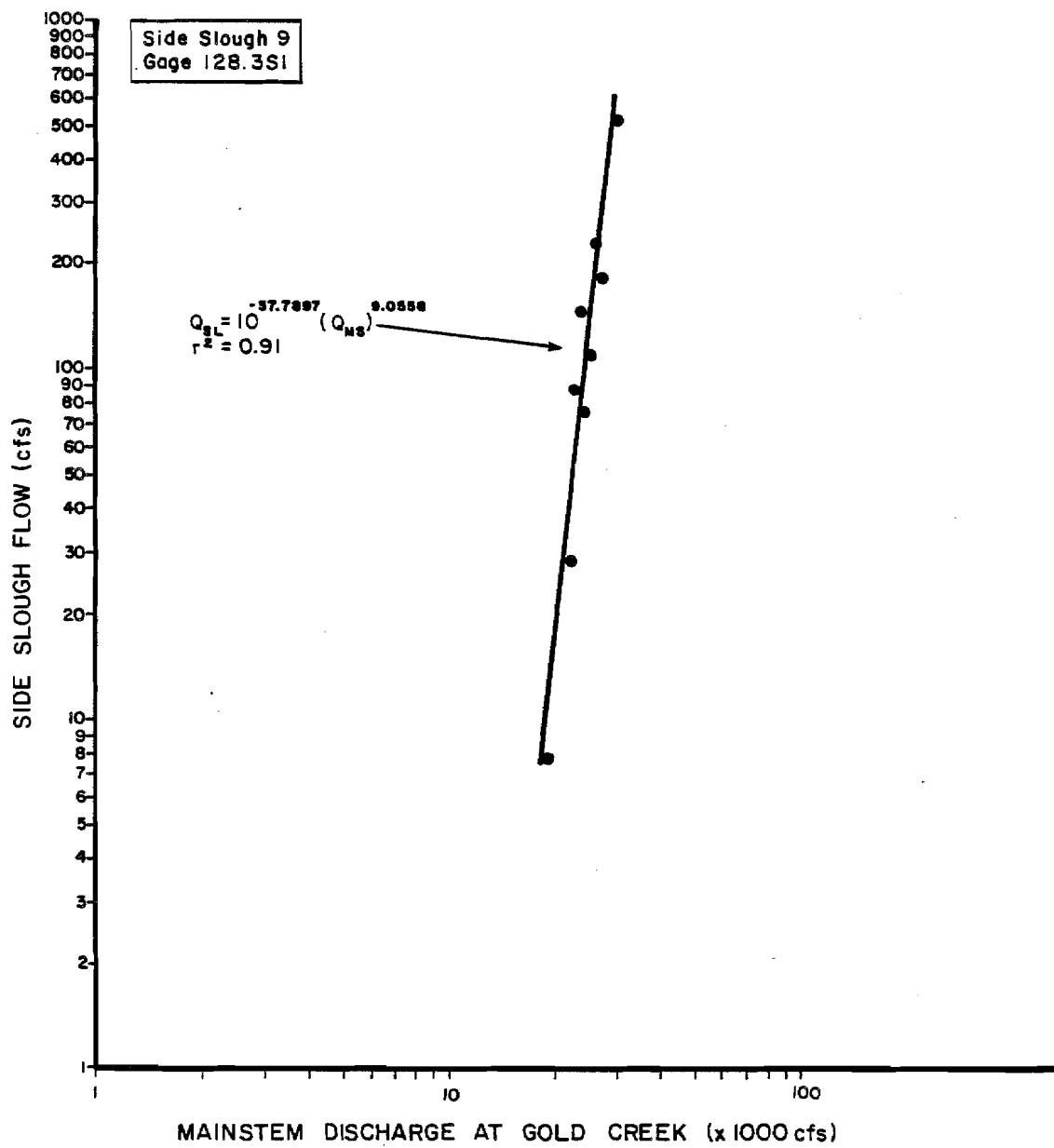
Figure 1-38. Slough flow versus mainstem discharge rating curve for Side Slough 9, staff gage 128.3S1.
