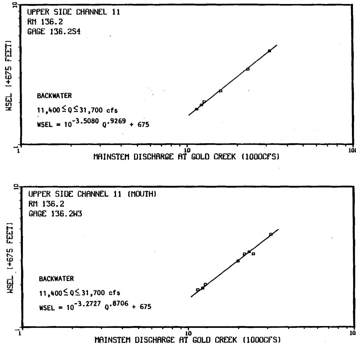
Appendix Figure 1-A-43 Non-Mainstem discharge (Provisional USGS 1983) versus the water surface elevation at Upper Side Channel 11 mouth and physical habitat modeling cross section 2 (136.2S4).
