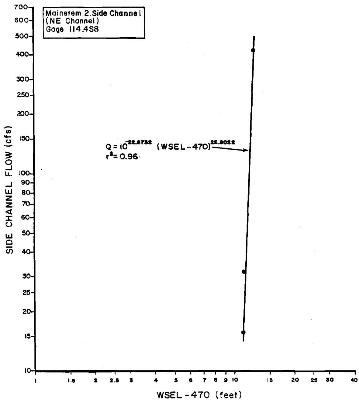
Figure 1-8. Stage versus flow rating curve for Mainstem 2 Side Channel (N.E. Channel), staff gage 114.4S8.
