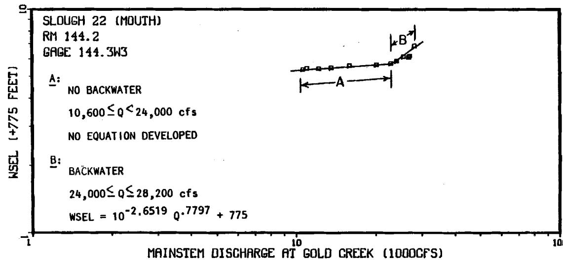
Appendix Figure 1-A-55 Non-Mainstem discharge (Provisional USGS 1983) versus the water surface elevation at Slough 22 mouth and mid slough.
