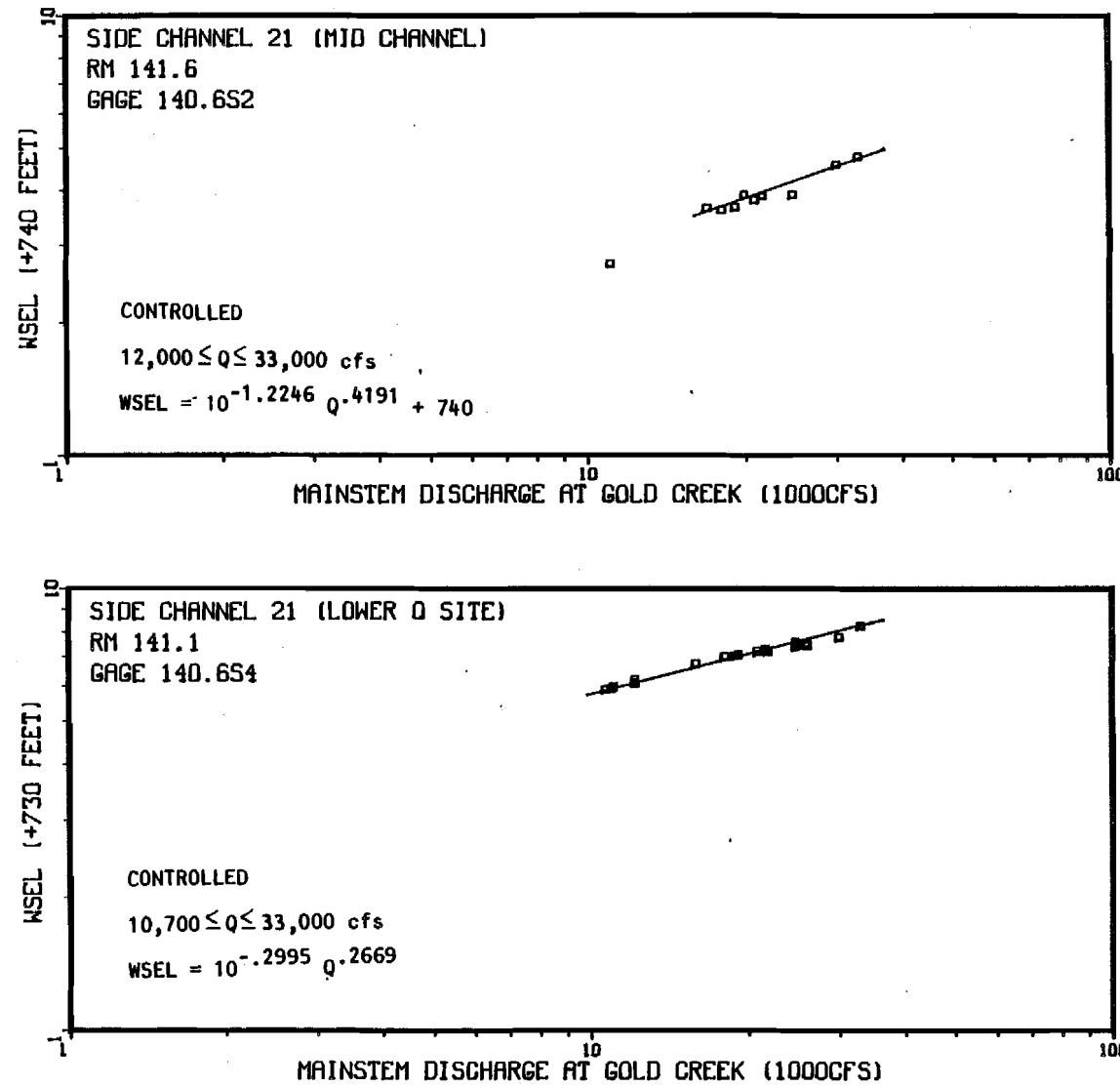
Appendix Figure 1-A-51 Non-Mainstem discharge (Provisional USGS 1983) versus the water surface elevation at Side Channel 21 Lower discharge site and mid channel.
