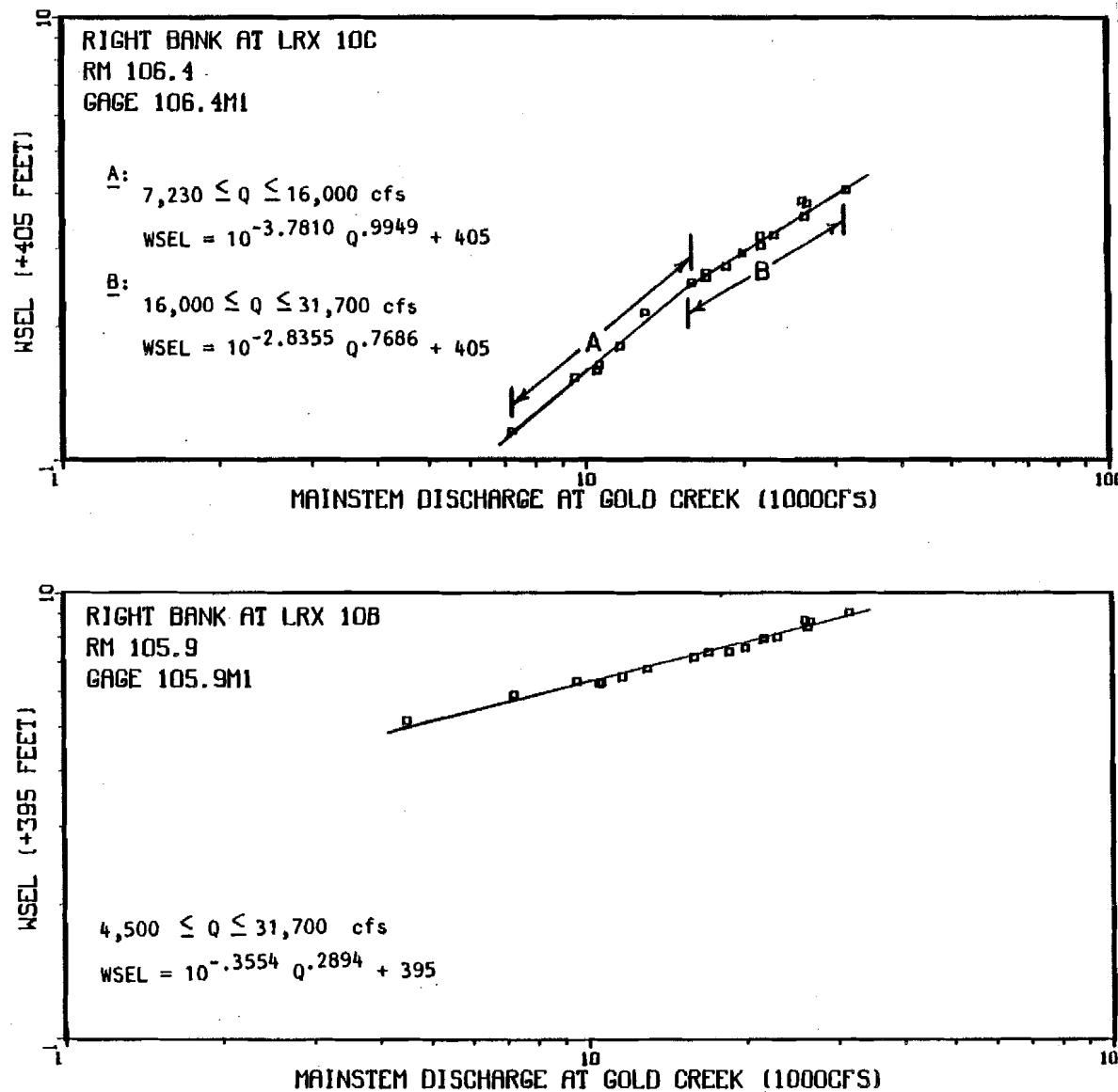
Appendix Figure 1-A-3. Mainstem discharge (Provisional USGS 1983) versus mainstem water surface elevation at LRX 10B and right bank at LRX 10C.
