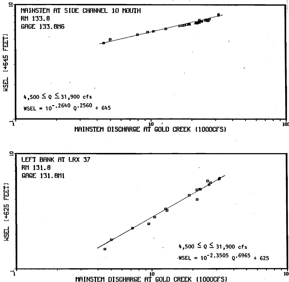
Appendix Figure 1-A-15. Mainstem discharge (Provisional USGS 1983) versus mainstem water surface elevation at the left bank at LRX 37 and at Side Channel 10 mouth.
