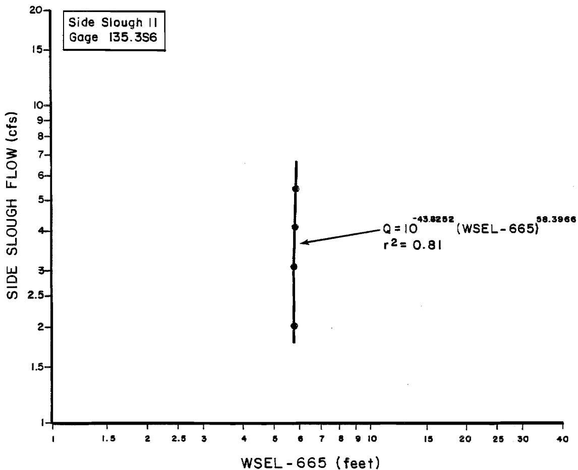
Figure 1-40. Stage versus flow rating curve for Side Slough II, staff gage 135.3S6.
