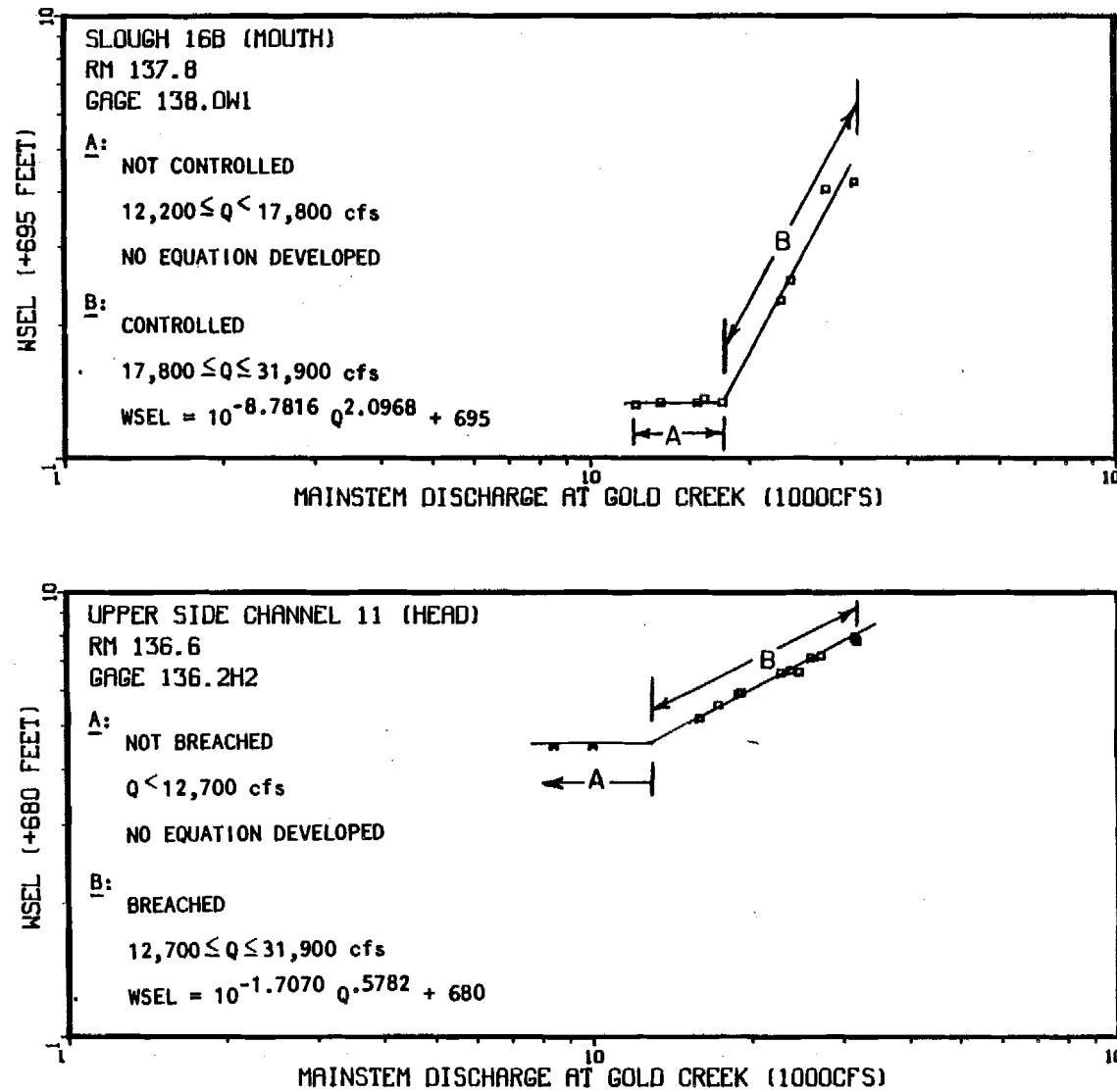
Appendix Figure 1-A-45 Non-Mainstem discharge (Provisional USGS 1983) versus the water surface elevation at Upper Side Channel 11 head and Slough 16B mouth.
