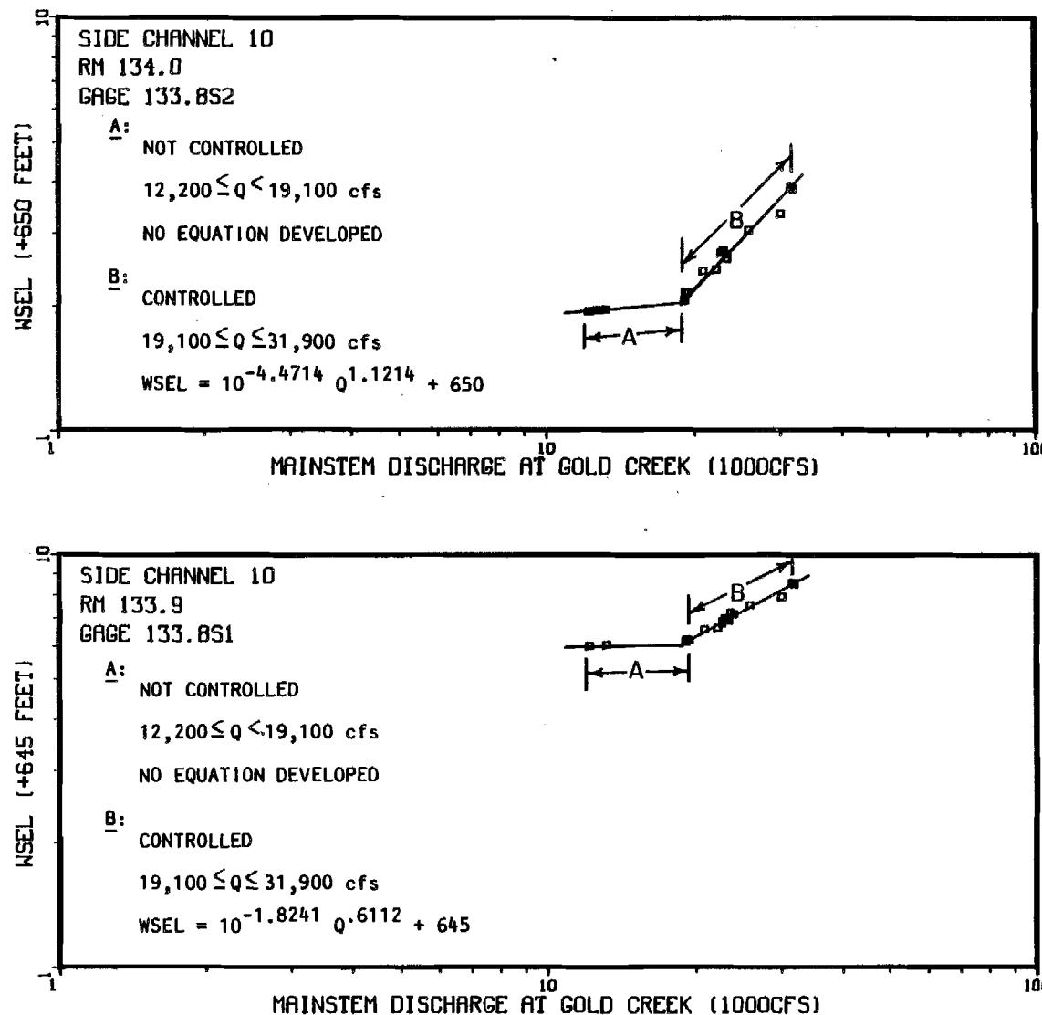
Appendix Figure 1-A-38 Non-Mainstem discharge (Provisional USGS 1983) versus the water surface elevation at Side Channel 10 physical habitat modeling cross sections 1 and 2 (staff gages 133.8S1 and 133.8S2).
