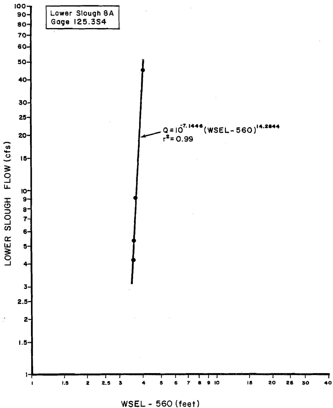
Figure 1-31. Stage versus flow rating curve for Side Slough 8A, staff gage 125.3S4.
