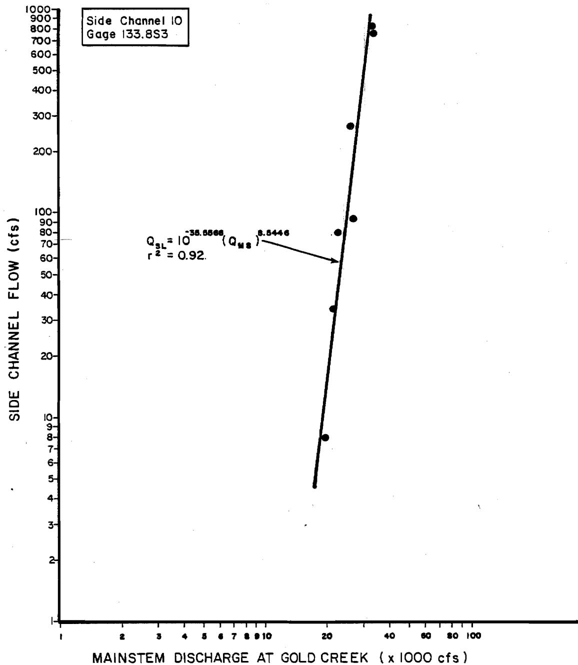
Figure 1-13. Side Channel flow versus mainstem discharge rating curve for Side Channel 10, staff gage 133.8S3.
