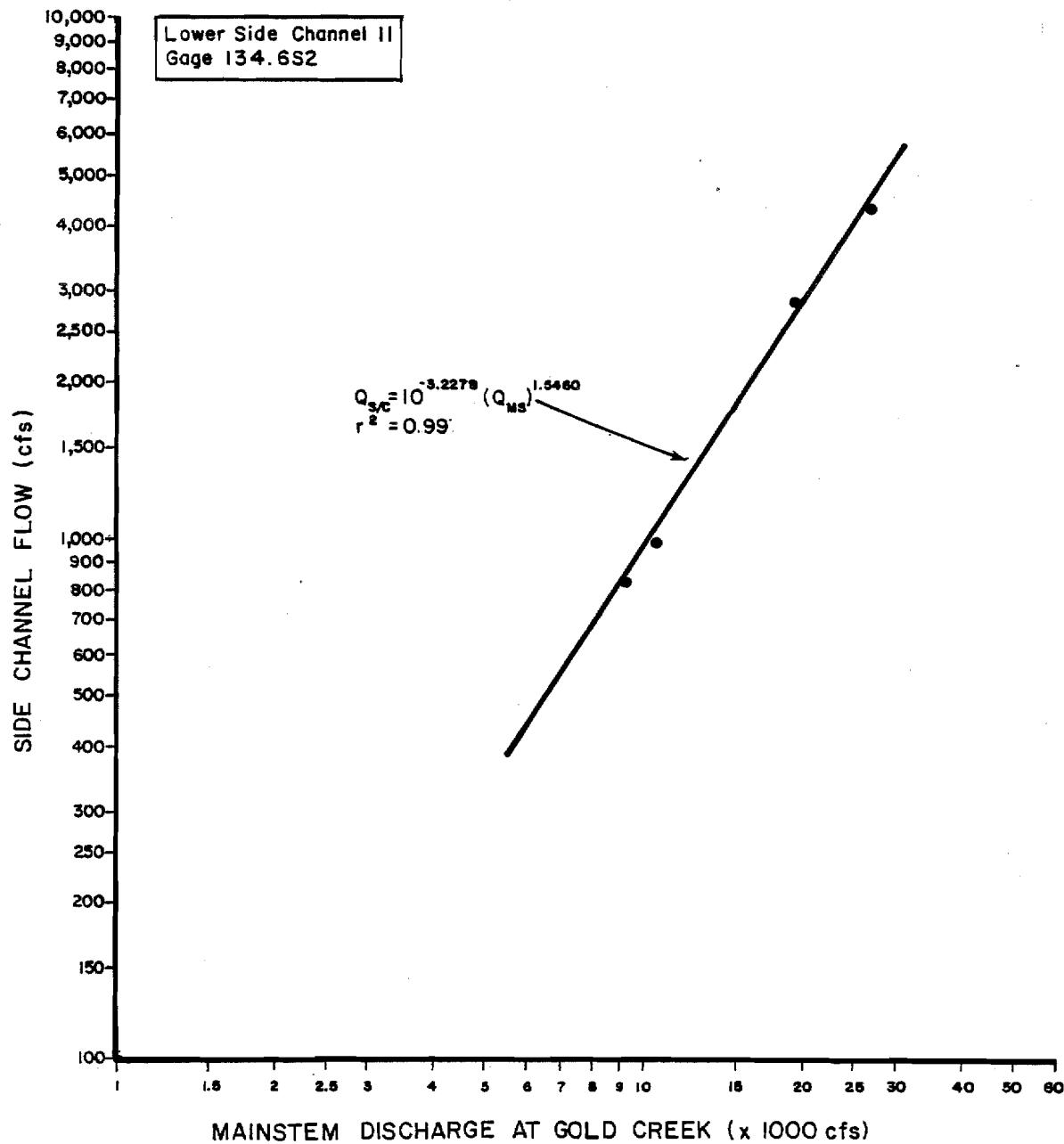
Figure 1-16. Side Channel flow versus mainstem discharge rating curve for Lower Side Channel 11, staff gage 134.6S2.
