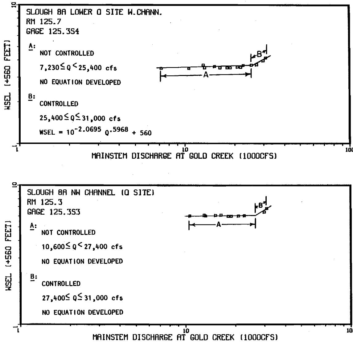
Appendix Figure 1-A-33 Non-Mainstem discharge (Provisional USGS 1983) versus the water surface elevation at Slough 8A NW Channel discharge site and lower discharge site west channel.
