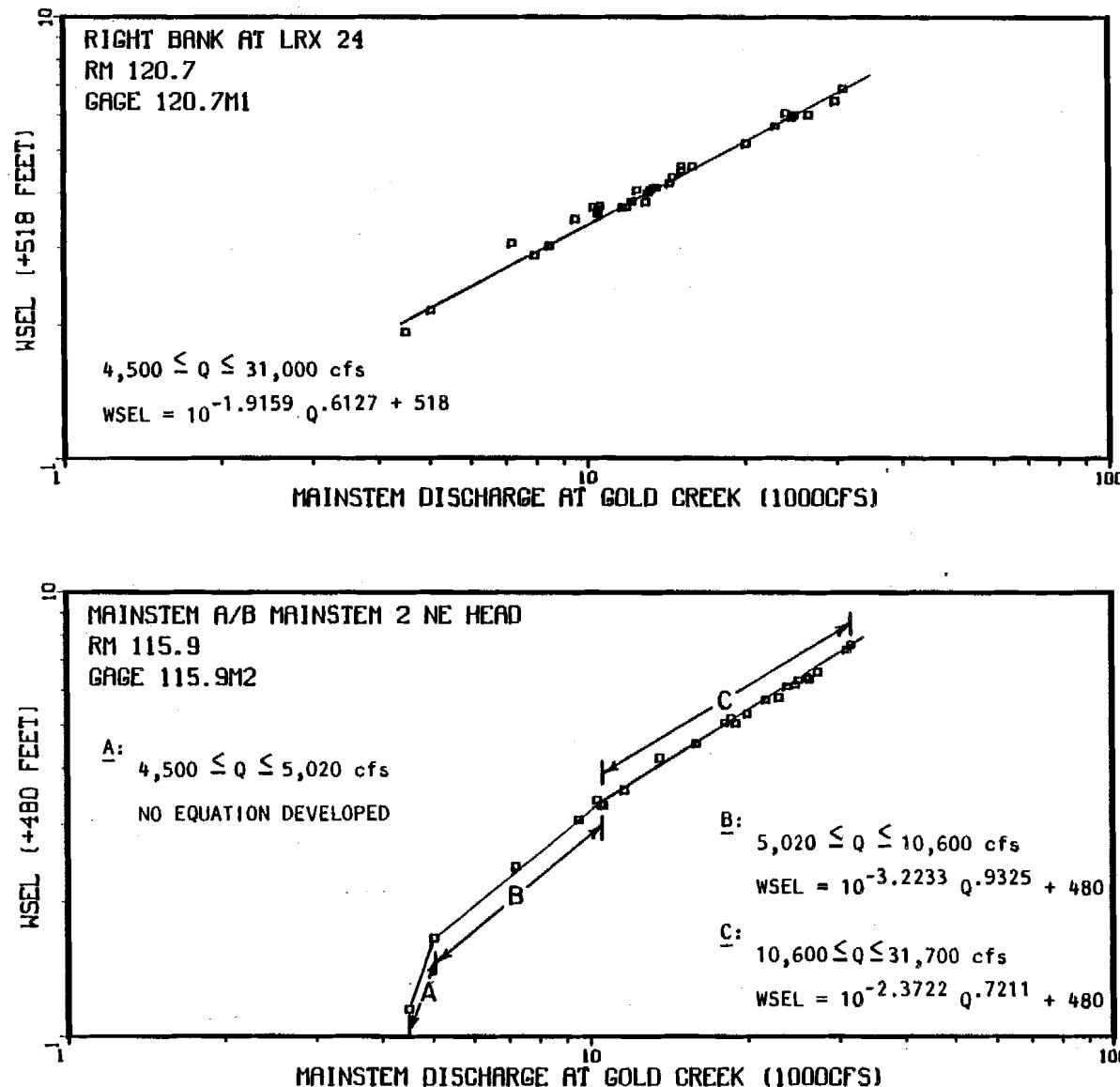
Appendix Figure 1-A-9. Mainstem discharge (Provisional USGS 1983) versus mainstem water surface elevation above Mainstem 2 Side Channel NE head and the right bank at LRX 24.
