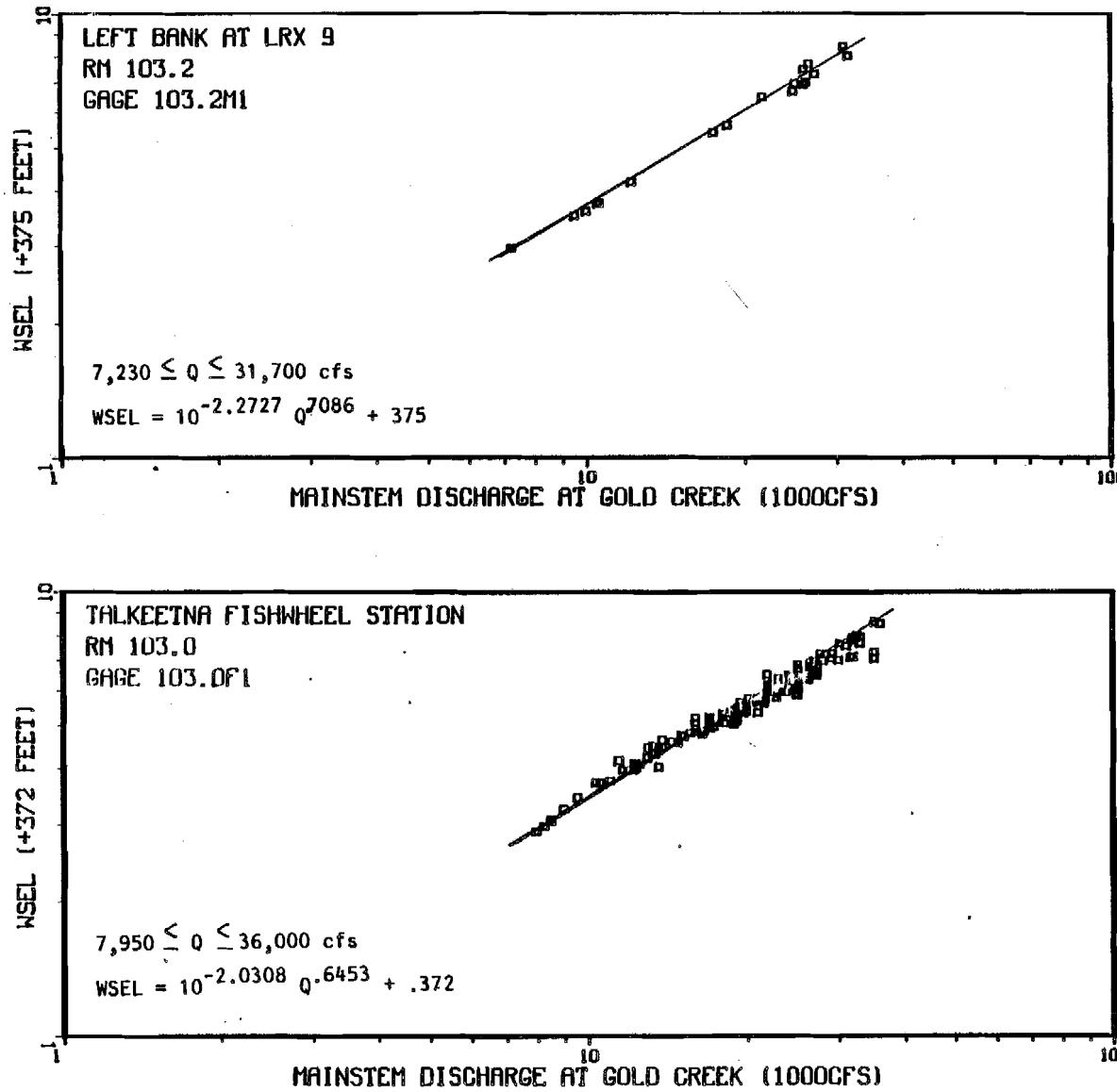
Appendix Figure 1-A-2. Mainstem discharge (Provisional USGS 1983) versus mainstem water surface elevation at Talkeetna Fishwheel Station and left bank at LRX 9.
