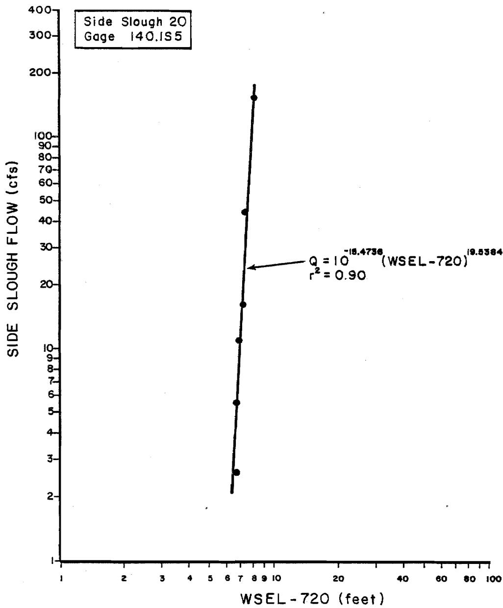
Figure 1-45. Stage versus flow rating curve for Side Slough 20, staff gage 140.1S5.
