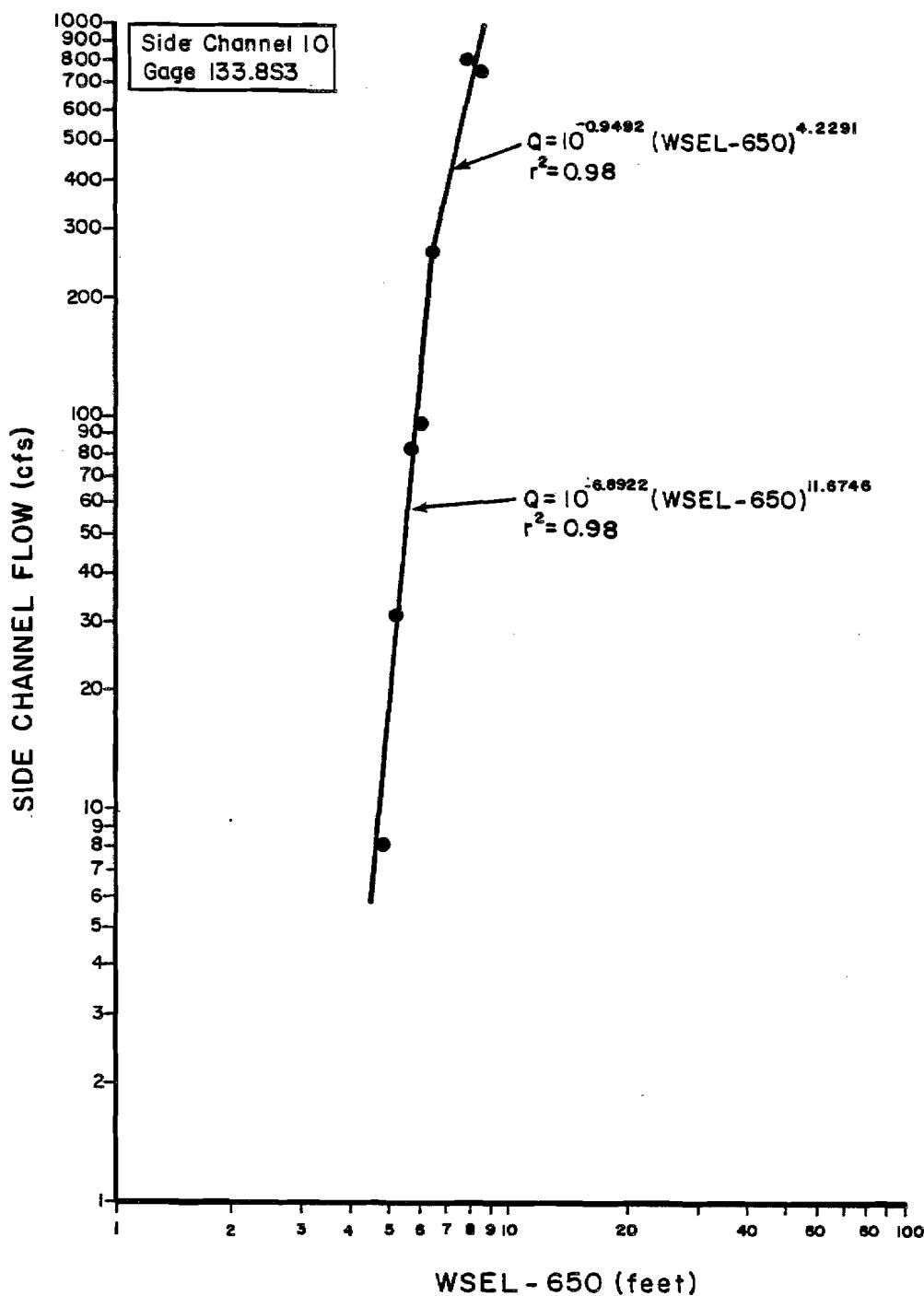
Figure 1-12. Stage versus flow rating curve for Side Channel 10, staff gage 133.8S3.
