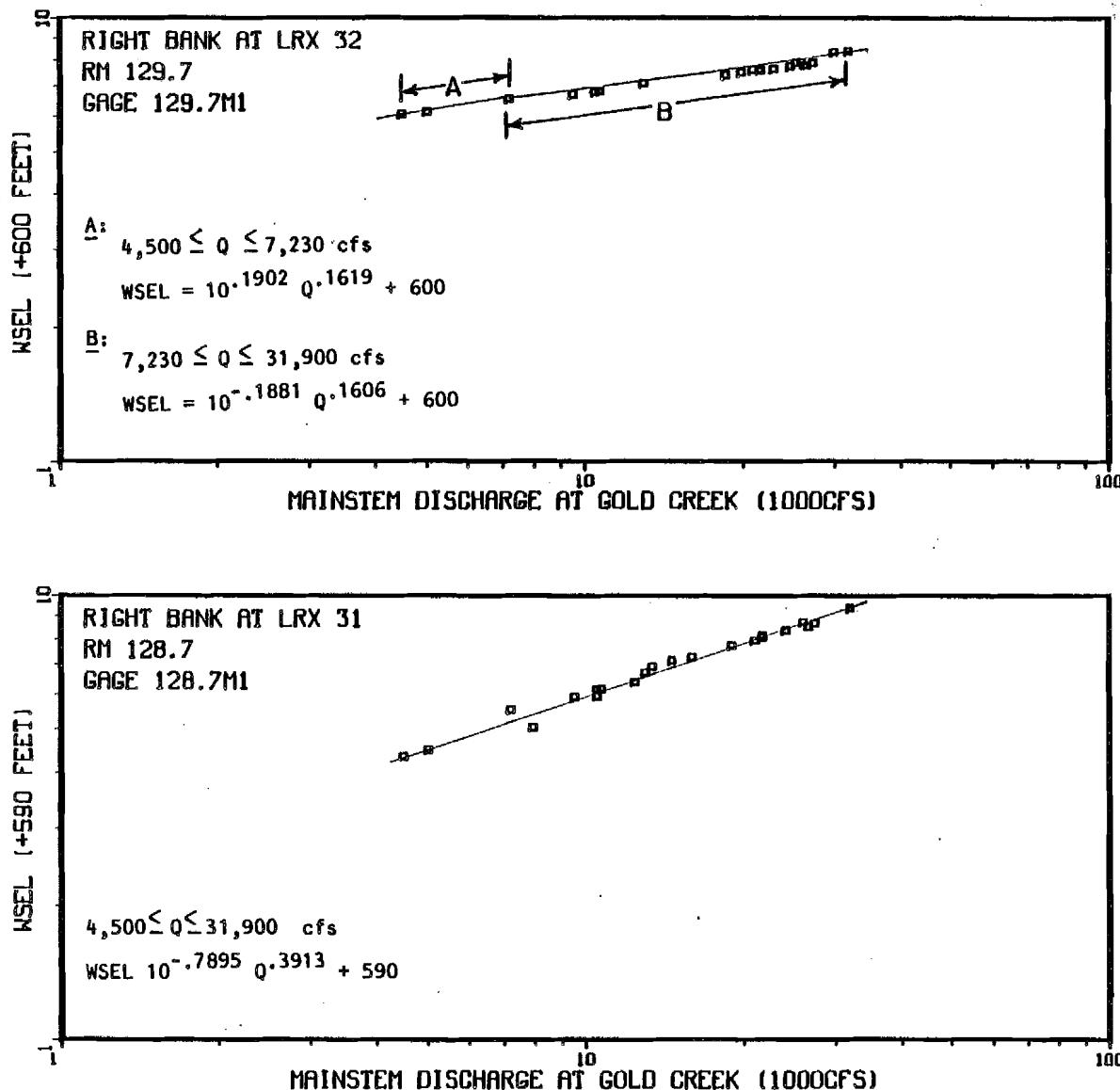
Appendix Figure 1-A-12. Mainstem discharge (Provisional USGS 1983) versus mainstem water surface elevation at the right bank at LRX 31 and LRX 32.
