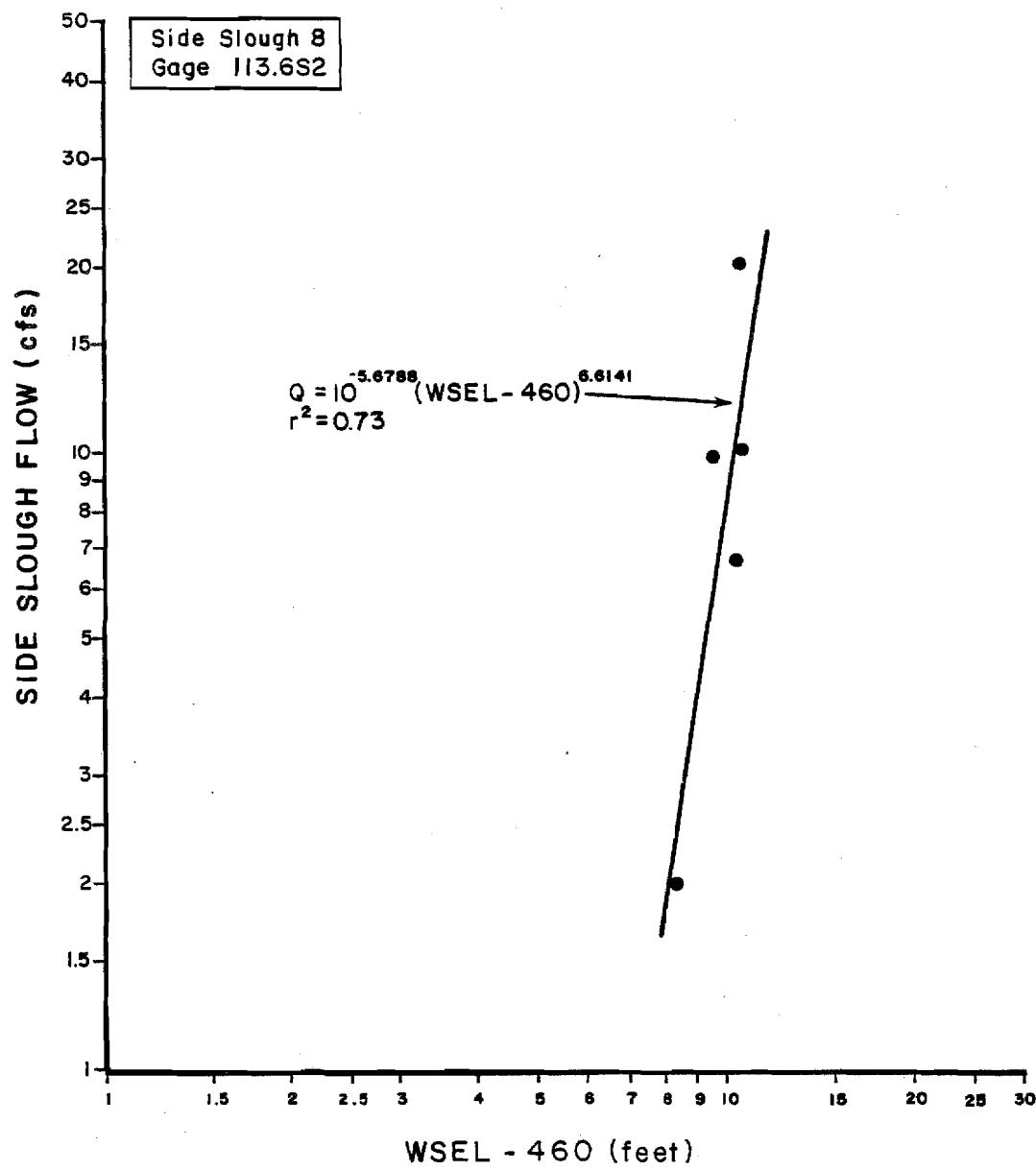
Figure 1-28. Stage versus flow rating curve for Slough 8, staff gage 113.6S2.
