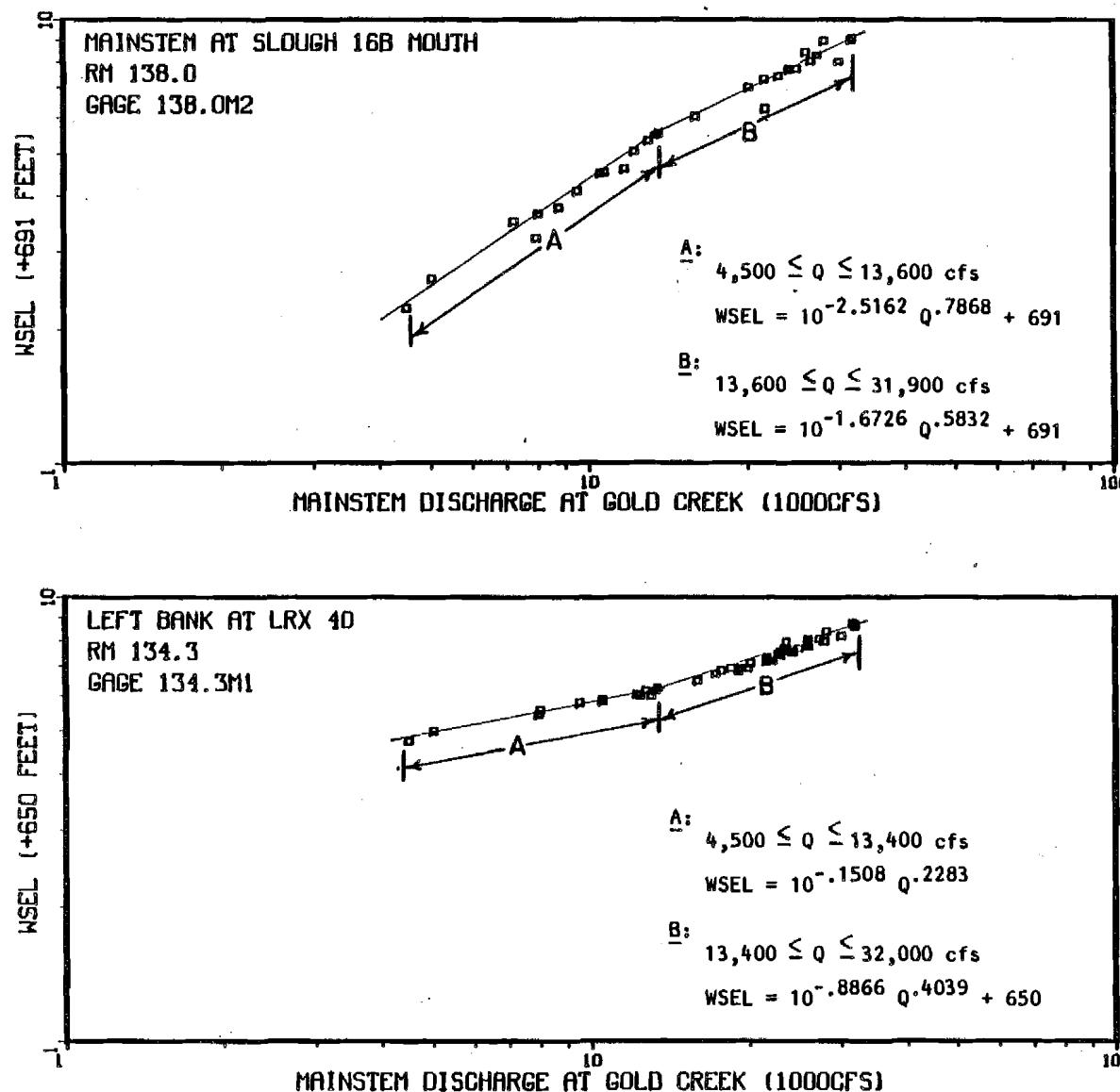
Appendix Figure 1-A-16. Mainstem discharge (Provisional USGS 1983) versus mainstem water surface elevation at the left bank at LRX 40 and at Side Slough 16B mouth.
