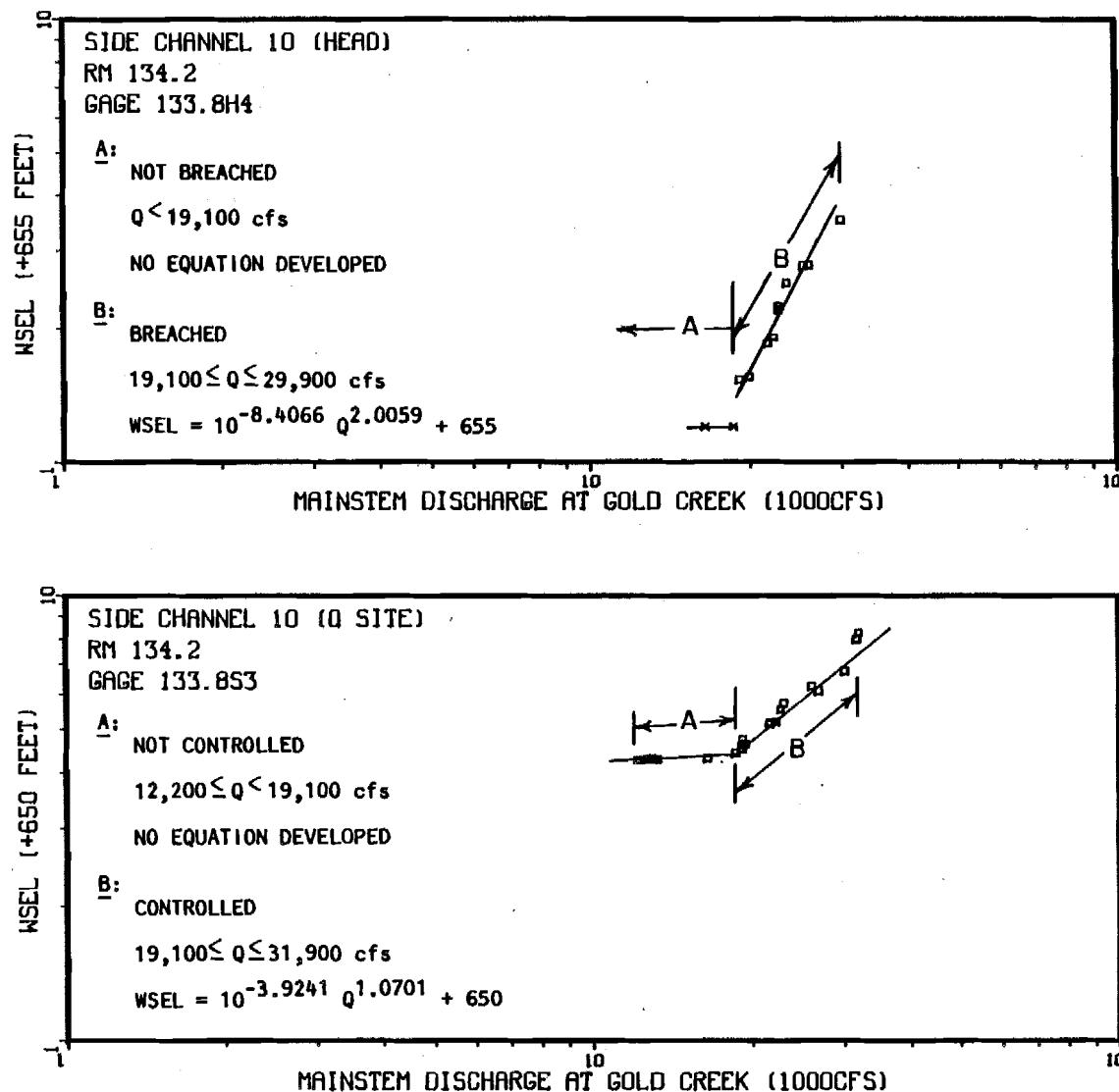
Appendix Figure 1-A-39 Non-Mainstem discharge (Provisional USGS 1983) versus the water surface elevation at Side Channel 10 physical habitat modeling cross section 4 (discharge site) and head.
