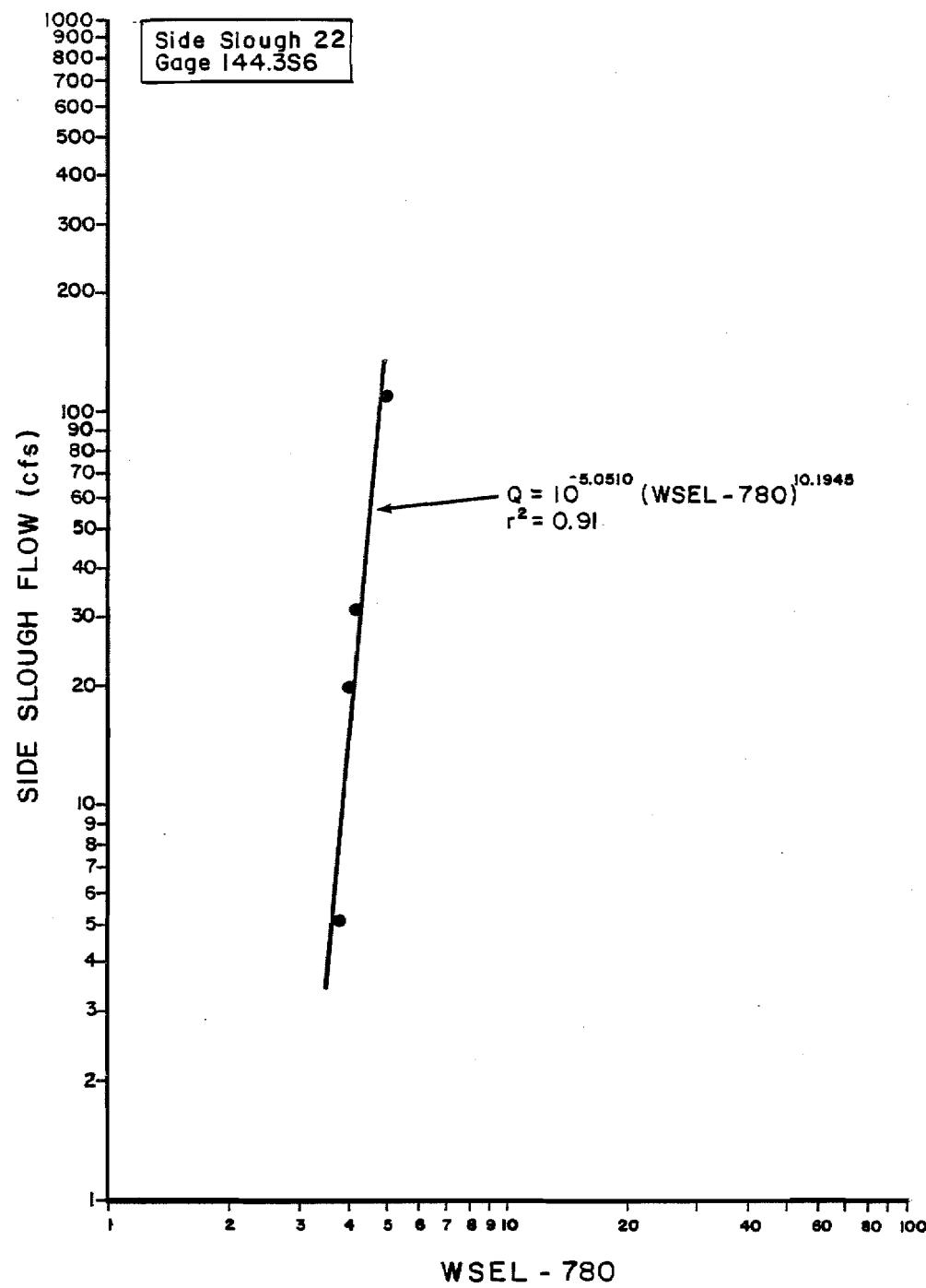
Figure 1-51. Stage versus flow rating curve for Side Slough 22, staff gage 144.3S6.
