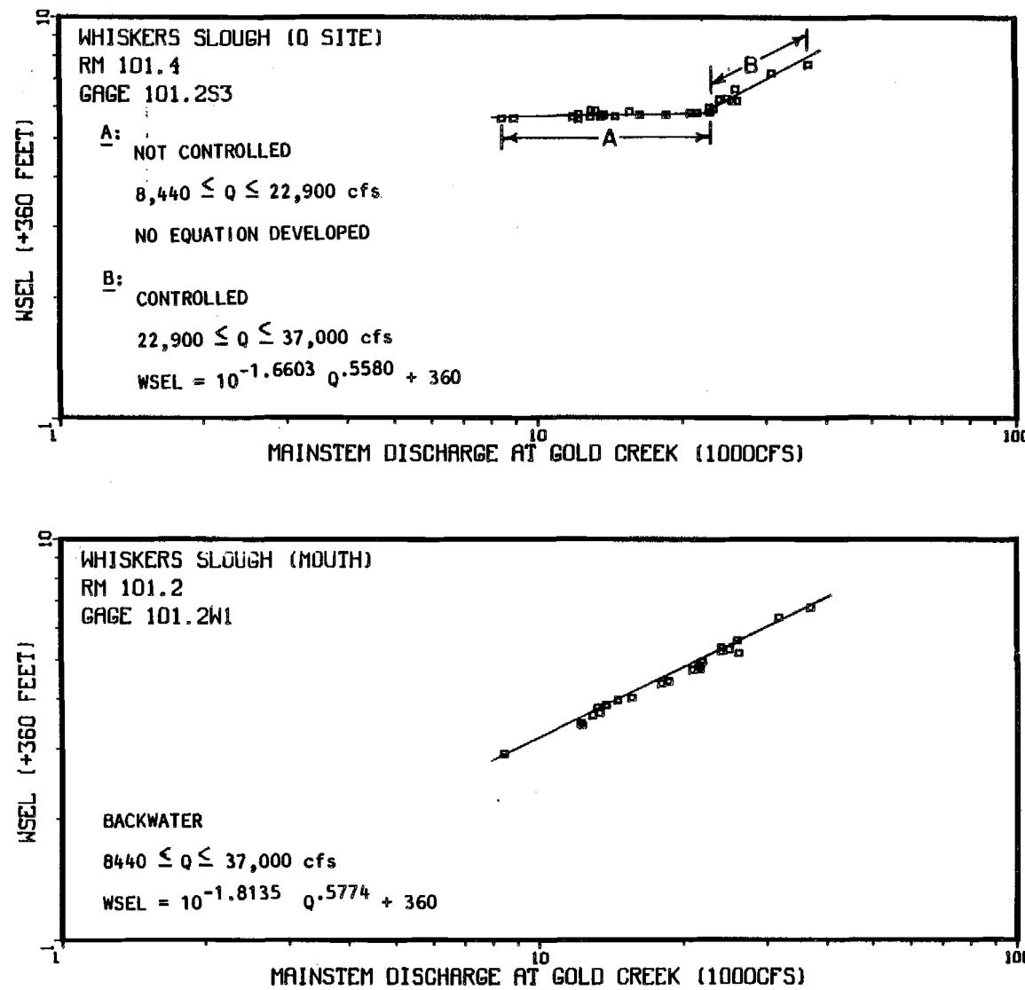
Appendix Figure 1-A-24 Non-mainstem discharge (Provisional USGS 1983) versus the water surface elevation at Whiskers Slough Mouth and discharge site.
