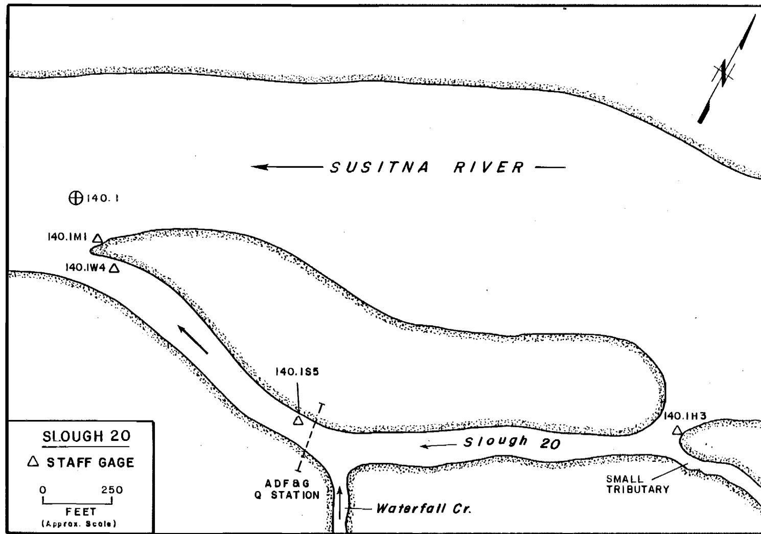
Figure 1-44. Site map for Side Slough 20, which is located on the east bank of the Susitna River at river mile 140.2.
