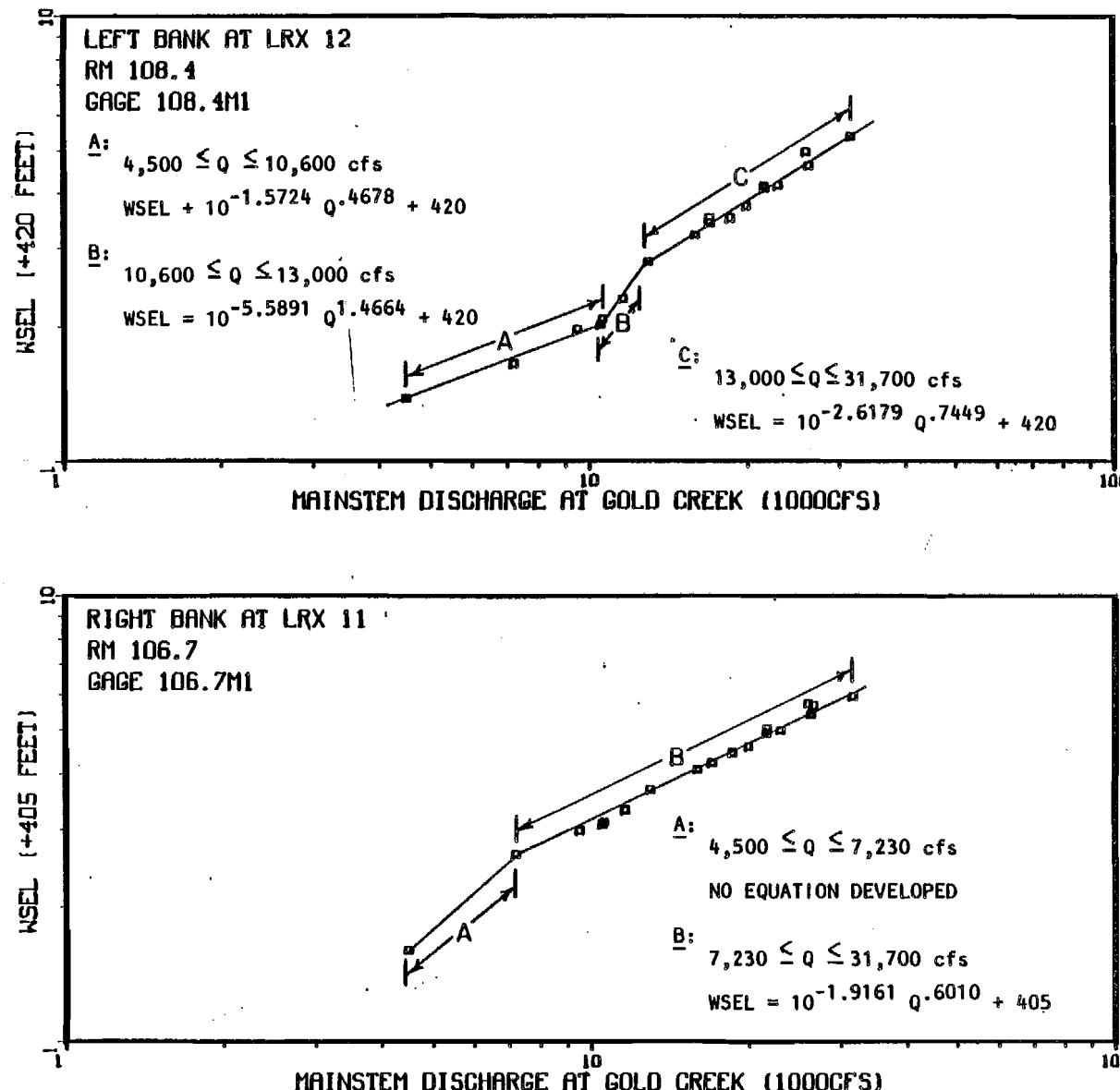
Appendix Figure 1-A-4. Mainstem discharge (Provisional USGS 1983) versus mainstem water surface elevation at right bank at LRX 11 and left bank at LRX 12.
