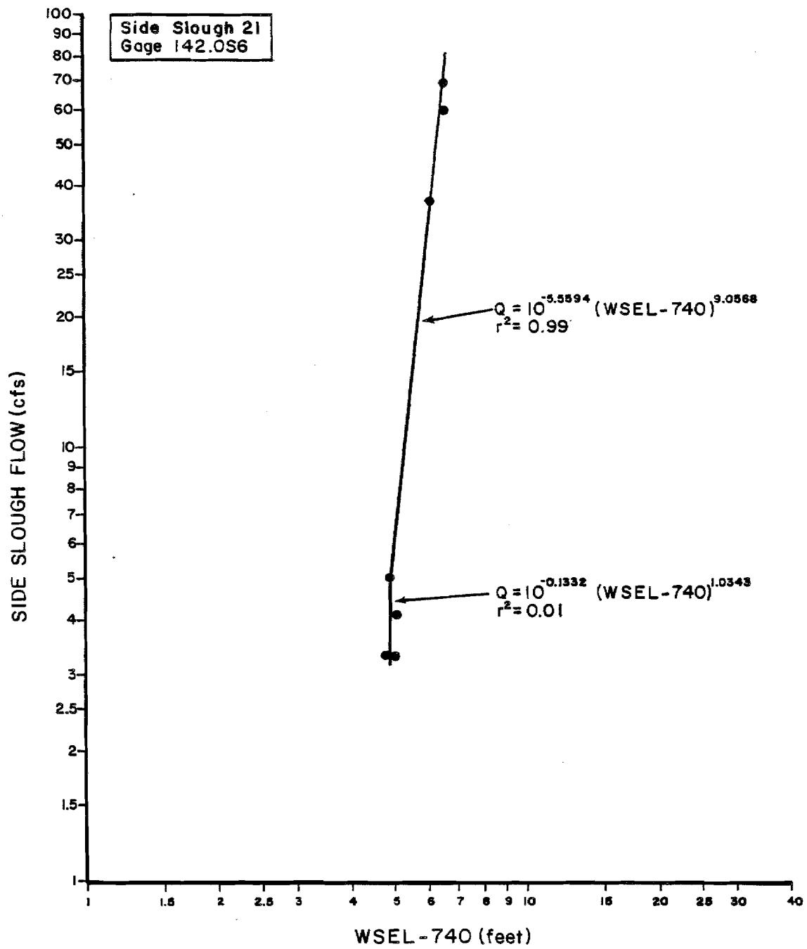
Figure 1-48. Stage versus flow rating curve for Side Slough 21, staff gage 142.056.
