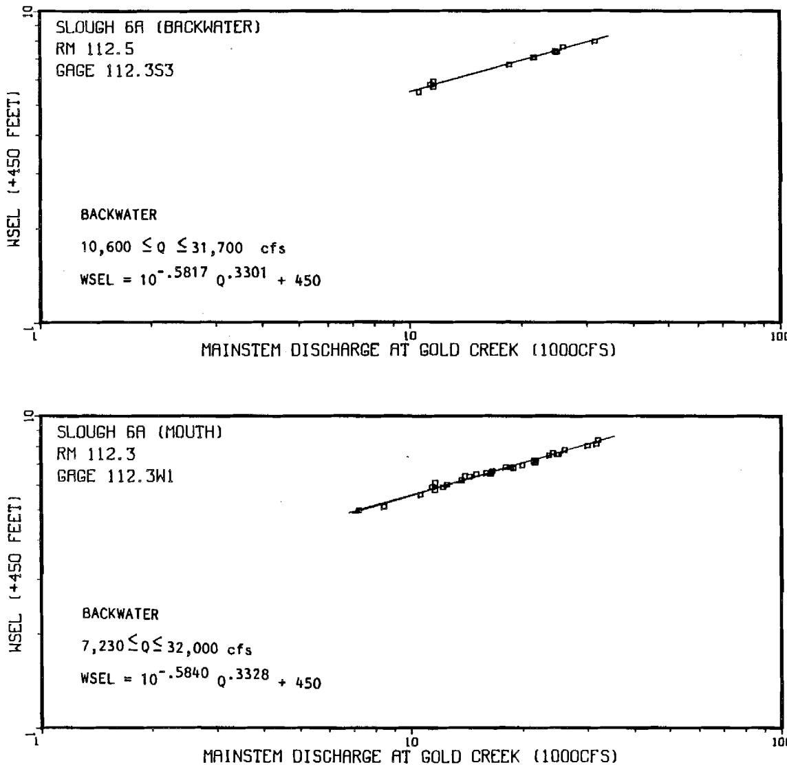
Appendix Figure 1-A-26. Non-Mainstem discharge (Provisional USGS 1983) versus the water surface elevation at Slough 6A mouth and backwater.
