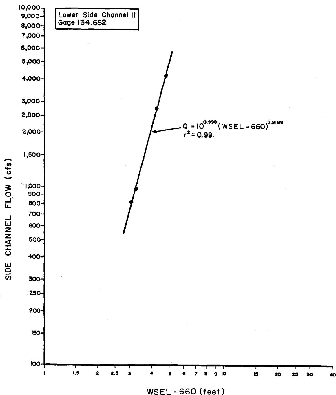
Figure 1-15. Stage versus flow rating curve for Lower Side Channel 11, staff gage 134.6S2.
