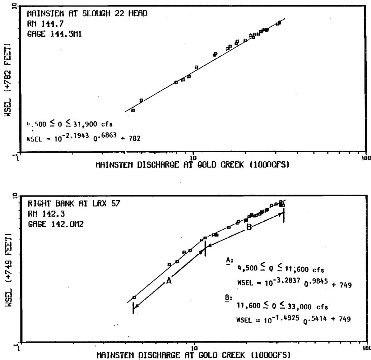
Appendix Figure 1-A-22. Mainstem discharge (Provisional USGS 1983) versus mainstem water surface elevation at the right bank at LRX 57 and at the mainstem at Side Slough 22 head.
