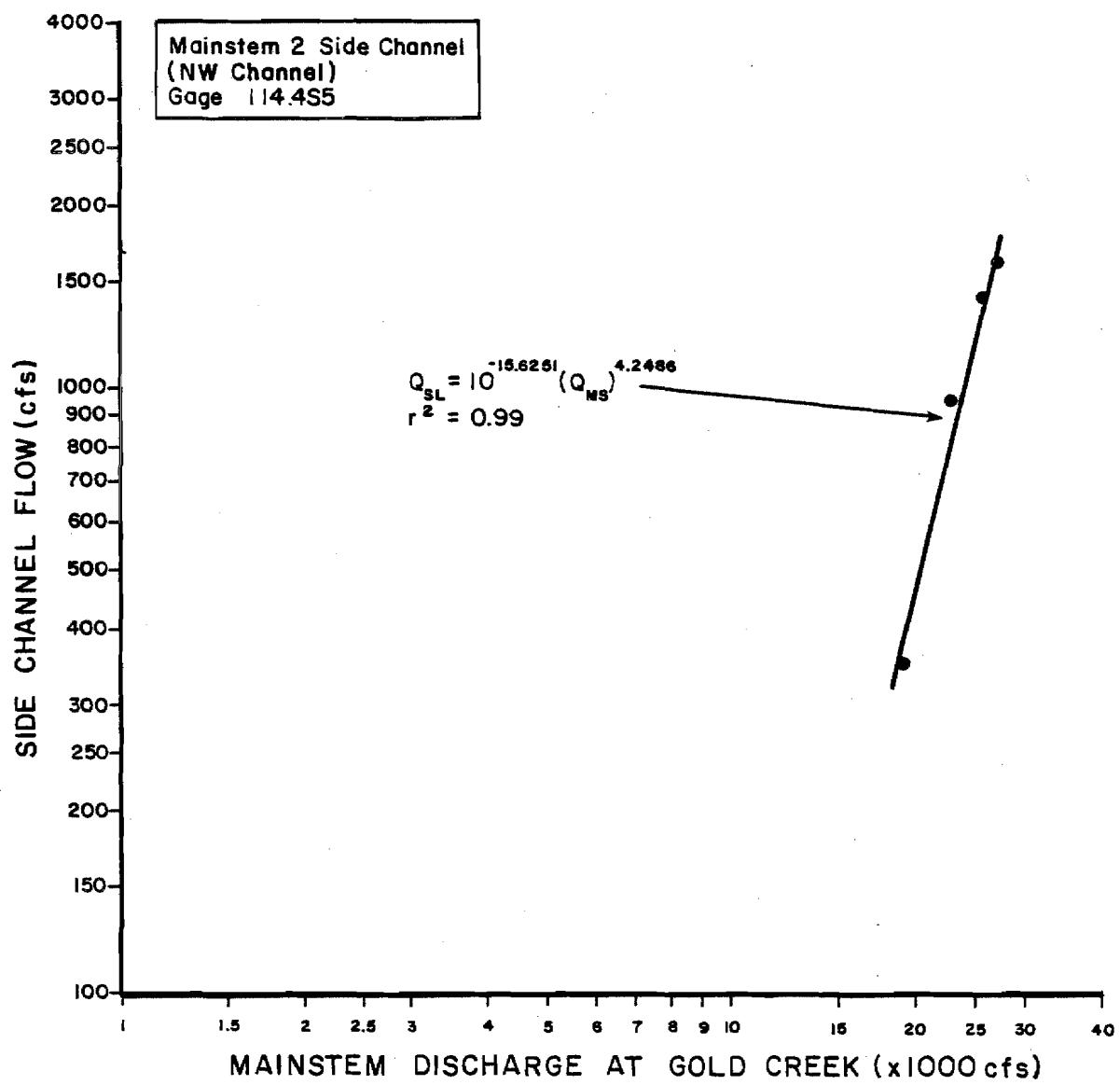
Figure 1-9. Side Channel flow versus mainstem discharge rating curve for Mainstem 2 (N.W. Channel), staff gage 114.4S5.
