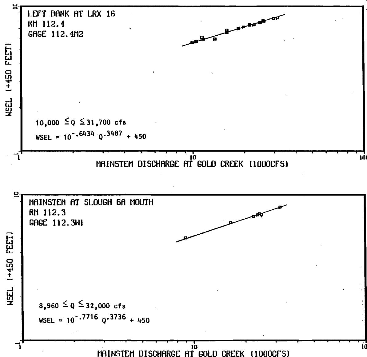
Appendix Figure 1-A-5. Mainstem discharge (Provisional USGS 1983) versus mainstem water surface elevation at Upland Slough 6A Mouth and left bank at LRX 16.
