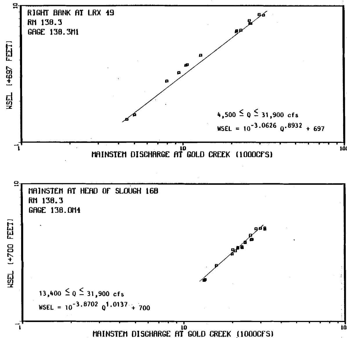
Appendix Figure 1-A-17. Mainstem discharge (Provisional USGS 1983) versus mainstem water surface elevation at the mainstem at the head of Side Slough 16B and the right bank at LRX 49.
