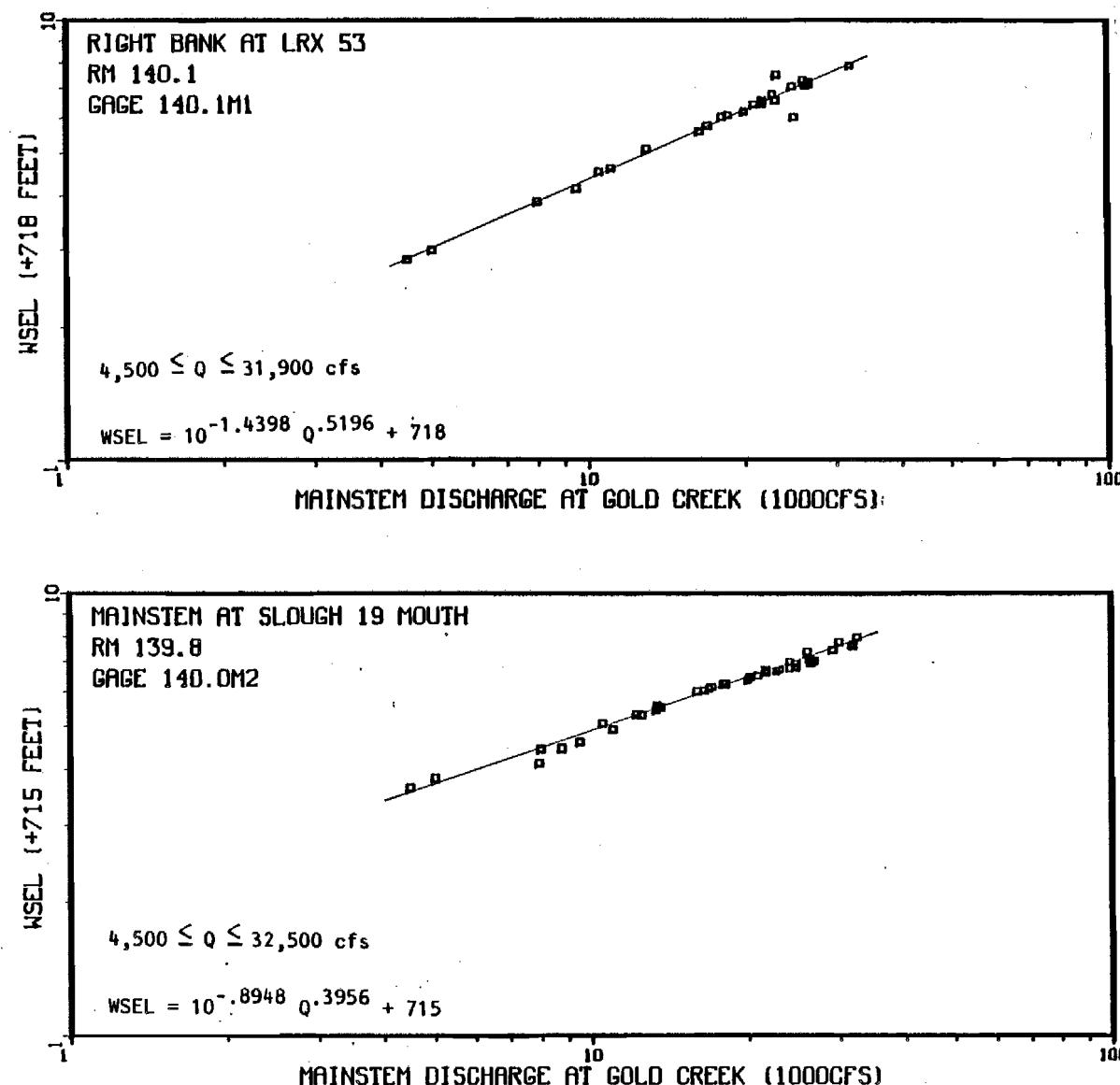
Appendix Figure 1-A-19. Mainstem discharge (Provisional USGS 1983) versus mainstem water surface elevation at Upland Slough 19 mouth and the right bank at LRX 53.
