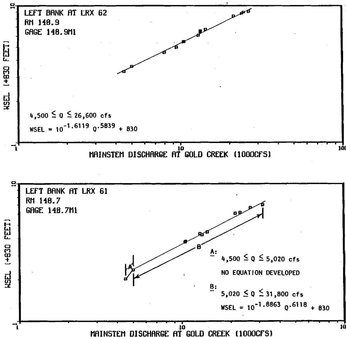
Appendix Figure 1-A-23. Mainstem discharge (Provisional USGS 1983) versus mainstem water surface elevation at the left bank at LRX 61 and the left bank at LRX 62.
