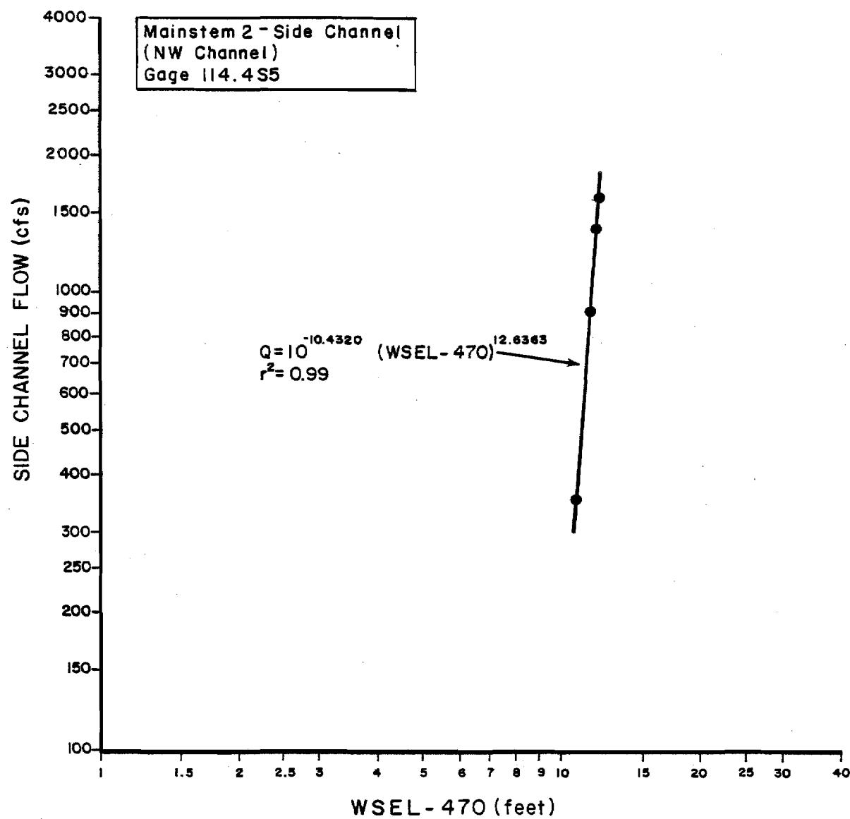
Figure 1-7. Stage versus flow rating curve for Mainstem 2 Side Channel (N.W. Channel), staff gage 114.4S5.
