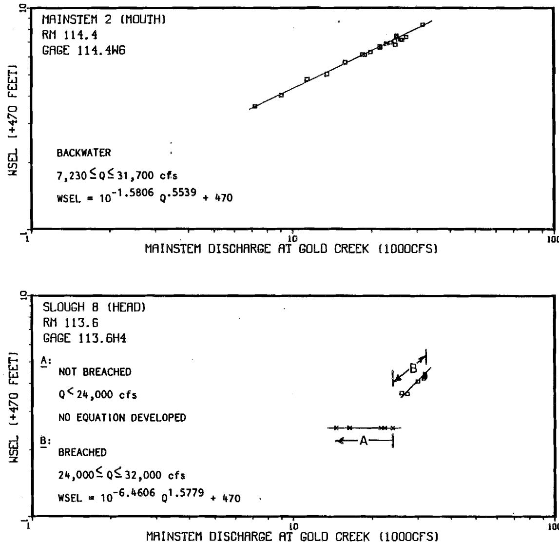
Appendix Figure 1-A-28. Non-Mainstem discharge (Provisional USGS 1983) versus the water surface elevation at Slough 8 head and Mainstem 2 mouth.
