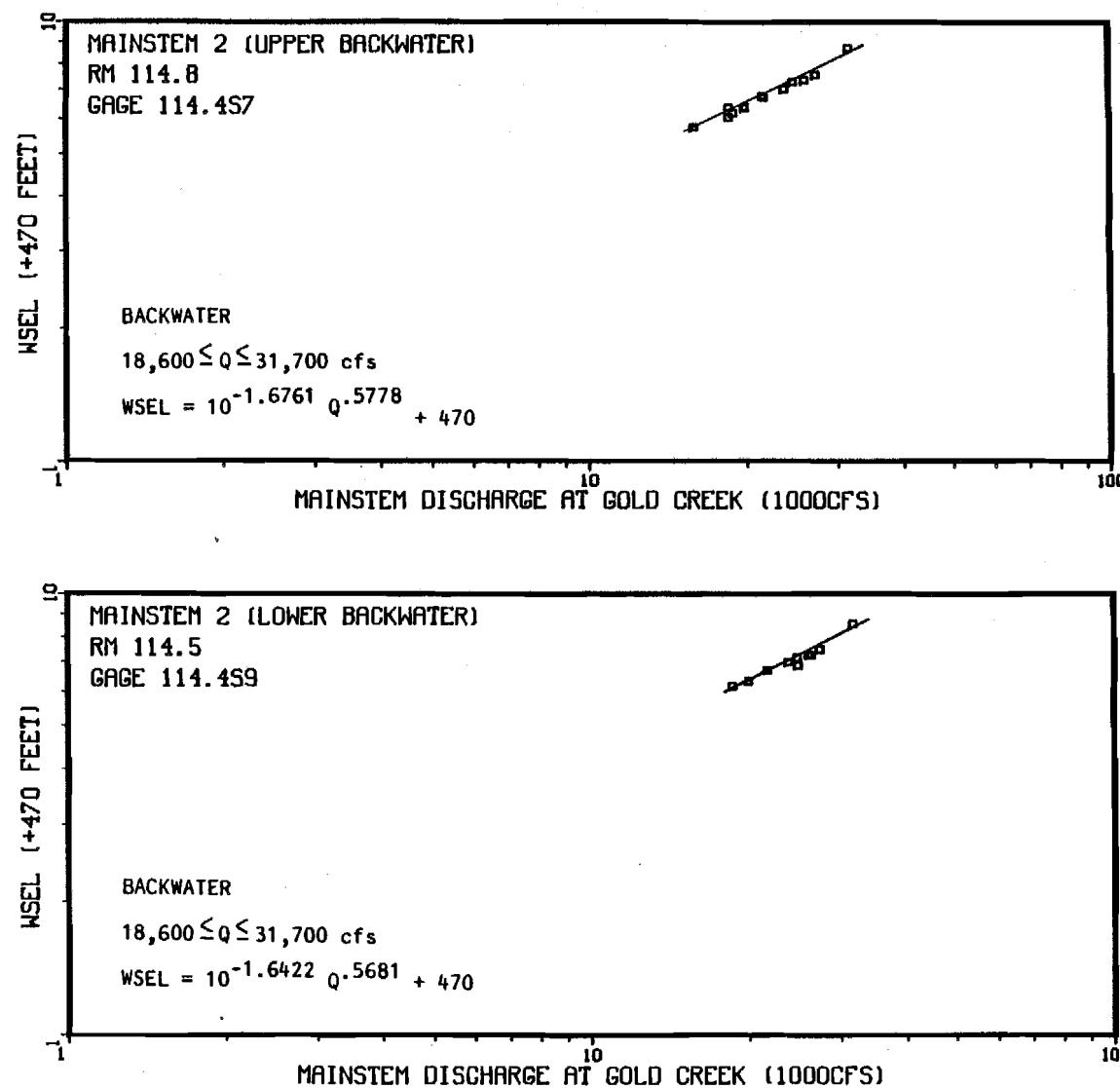
Appendix Figure 1-A-29 Non-Mainstem discharge (Provisional USGS 1983) versus the water surface elevation at Mainstem 2 lower backwater and upper backwater.
