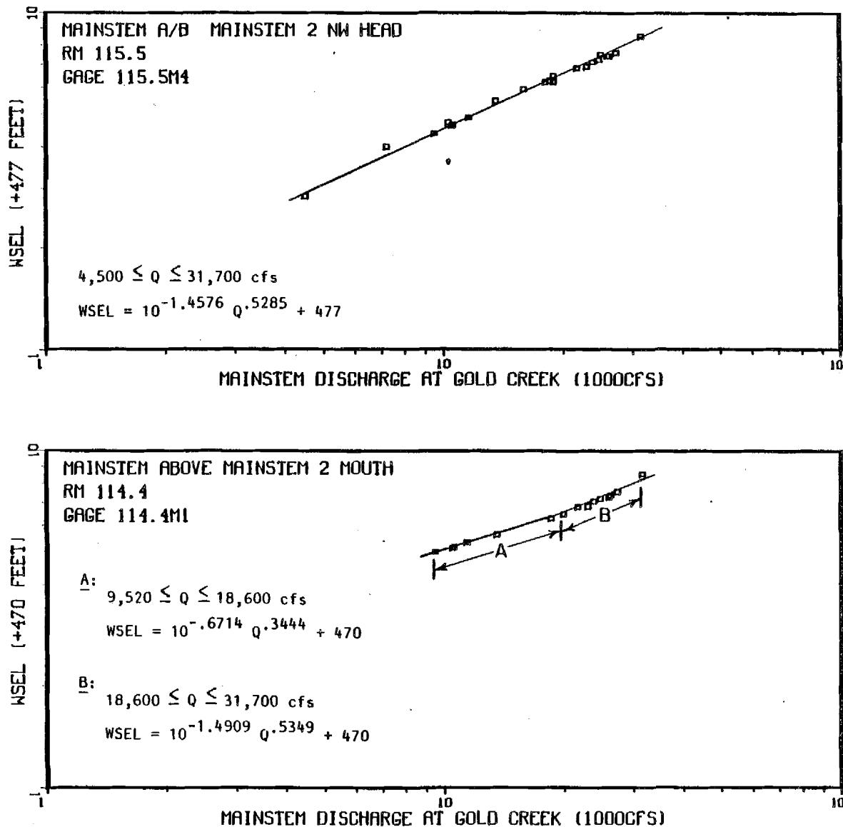
Appendix Figure 1-A-8. Mainstem discharge (Provisional USGS 1983) versus mainstem water surface elevation above Mainstem 2 Side Channel Mouth and above Mainstem 2 Side Channel NW head.
