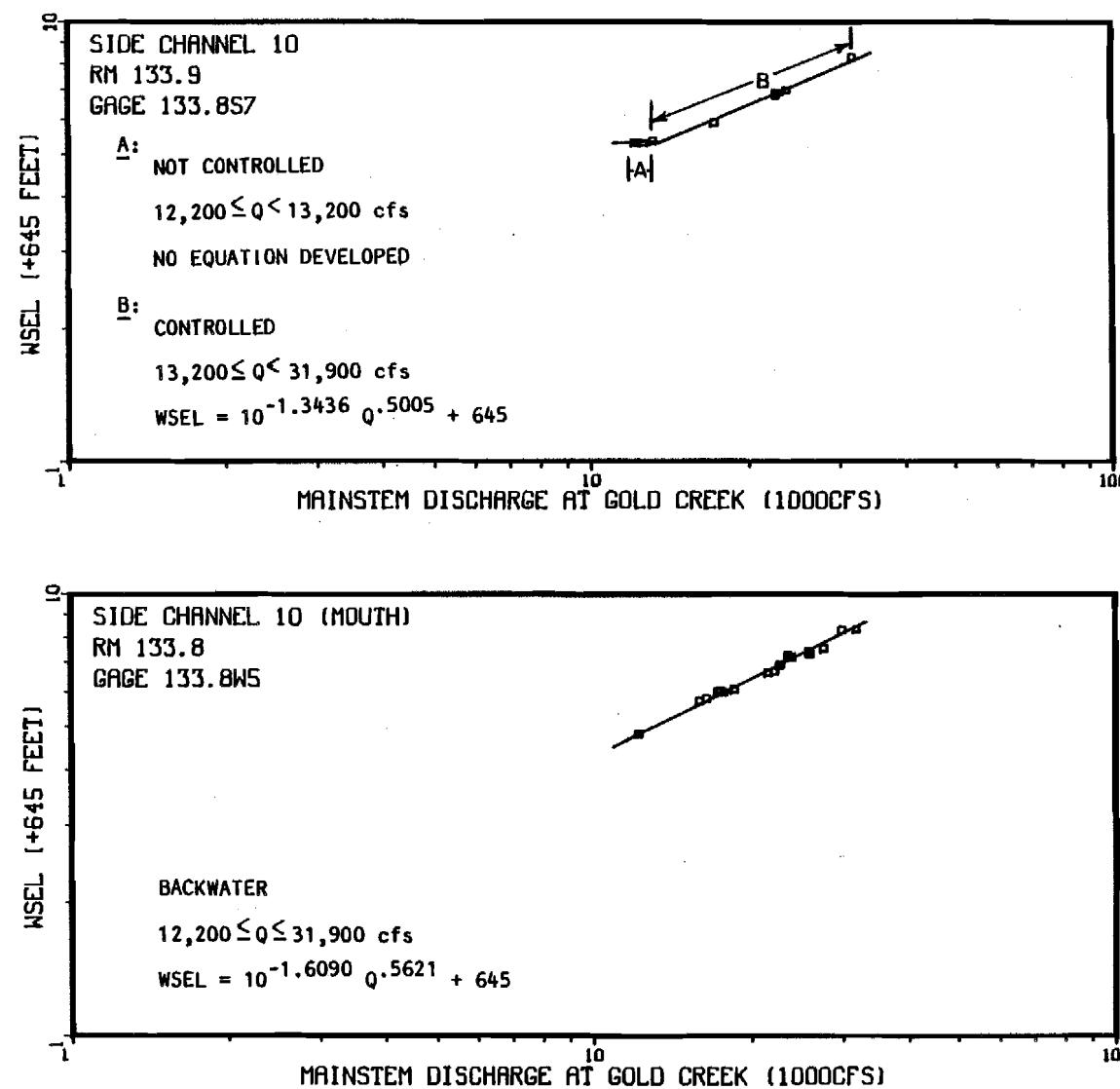
Appendix Figure 1-A-37 Non-Mainstem discharge (Provisional USGS 1983) versus the water surface elevation at Side Channel 10 mouth and Side Channel 10 at staff gage 133.8S7.
