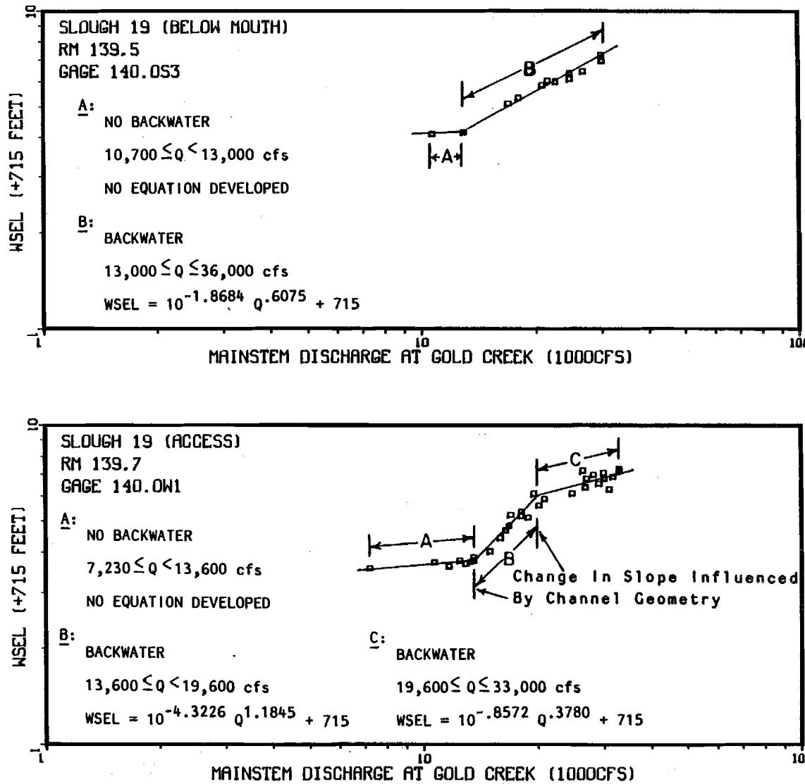
Appendix Figure 1-A-47 Non-Mainstem discharge (Provisional USGS 1983) versus the water surface elevation at Slough 19 access and below mouth.
