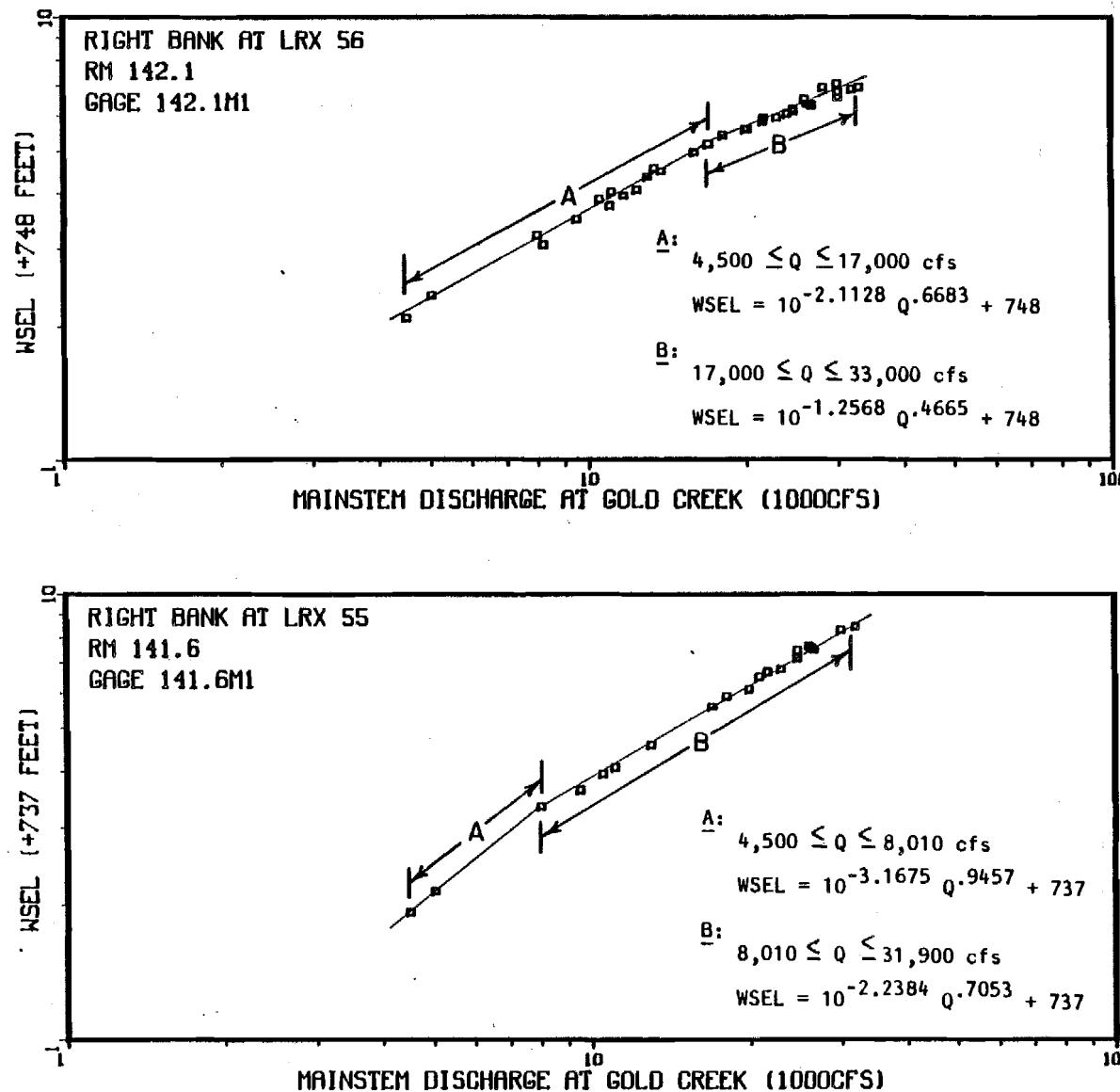
Appendix Figure 1-A-21. Mainstem discharge (Provisional USGS 1983) versus mainstem water surface elevation at the right bank at LRX 55 and the right bank at LRX 56.
