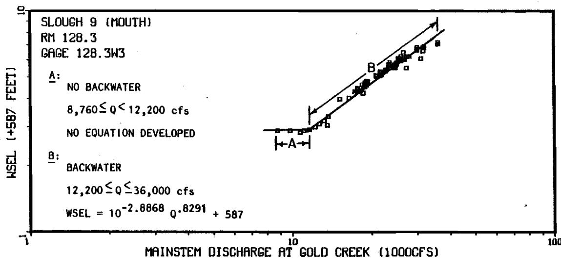
Appendix Figure 1-A-35 Non-Mainstem discharge (Provisional USGS 1983) versus the water surface elevation at Slough 9 mouth.
