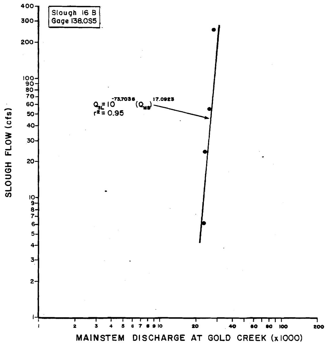
Figure 1-43. Slough flow versus mainstem discharge rating curve for Side Slough 16B, staff gage 138.0S5.
