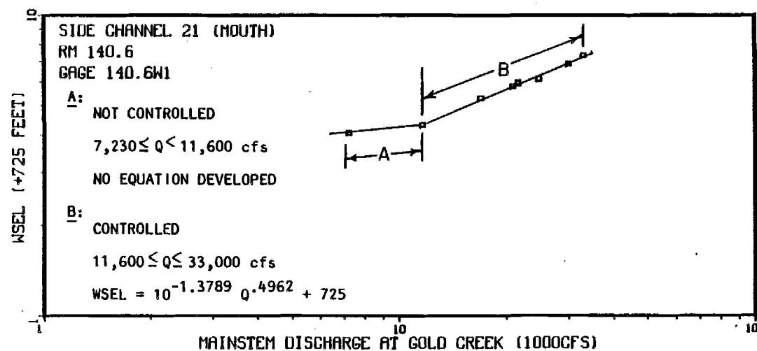
Appendix Figure 1-A-50 Non-Mainstem discharge (Provisional USGS 1983) versus the water surface elevation at Side Channel 21 mouth and Upper discharge site.
