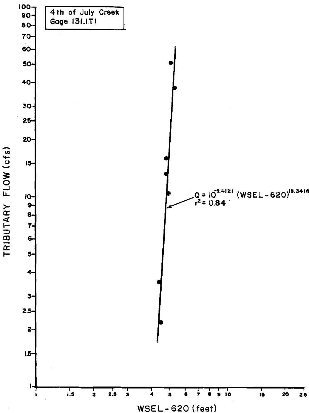
Figure 1-60. Stage versus flow rating curve for Fourth of July Creek staff gage 131.1T1.
