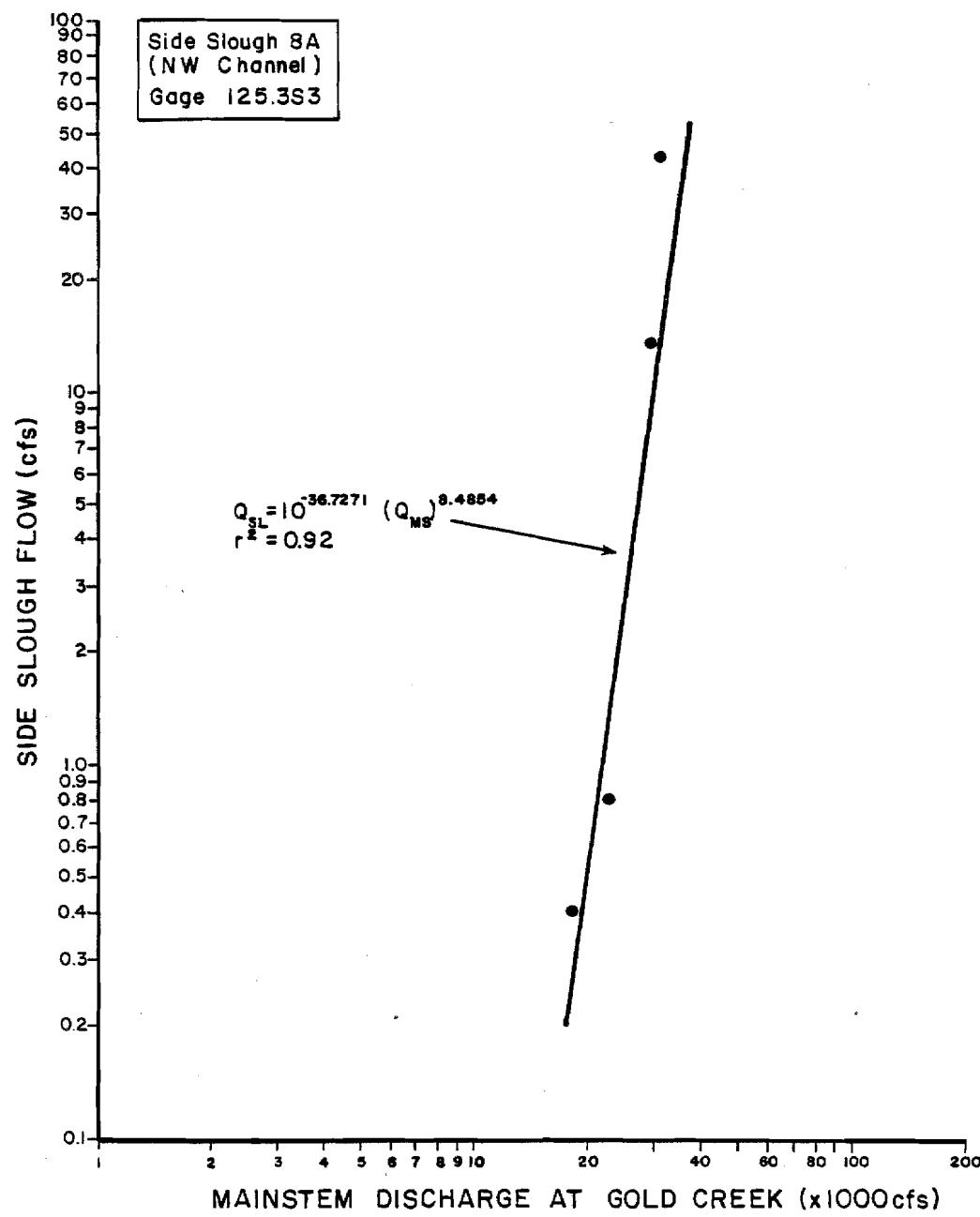
Figure 1-35. Slough flow versus mainstem discharge rating curve for Side Slough 8A, staff gage 125.3S3.
