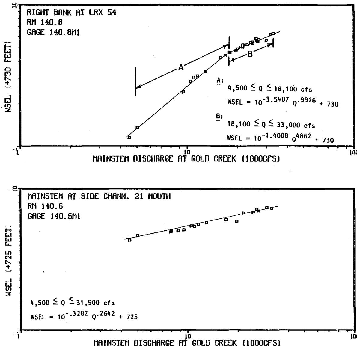
Appendix Figure 1-A-20. Mainstem discharge (Provisional USGS 1983) versus mainstem water surface elevation at Side Channel 21 mouth and the right bank at LRX 54.
