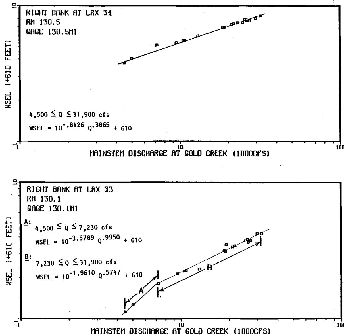
Appendix Figure 1-A-13. Mainstem discharge (Provisional USGS 1983) versus mainstem water surface elevation at the right bank at LRX 33 and at the right bank at LRX 34.
