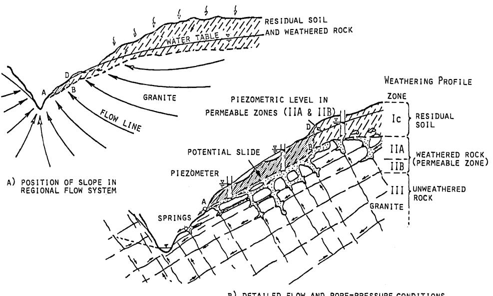
B) DETAILED FLOW AND PORE-PRESSURE CONDITIONS
