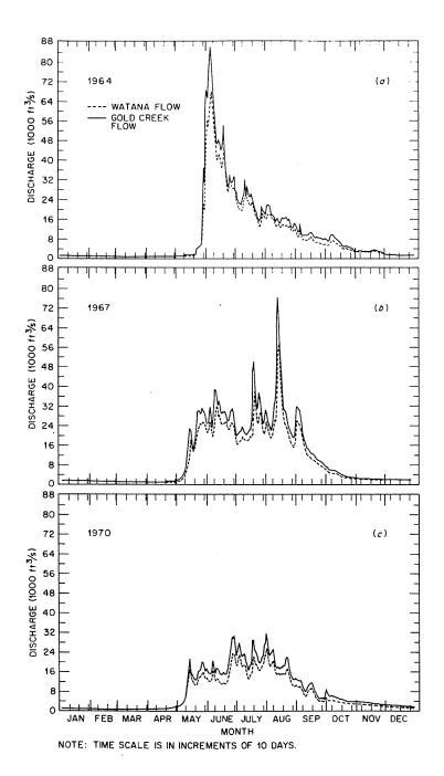
Figure H.2-1. Representatiave annual hydrographs at the Watana dam site and the Gold Creek gaging station for two wet years with spring (1964) and fall (1967) floods and for one dry year (1970). Source: Exhibit E, Figures E.2.24, E.2.25, and E.2.26.
