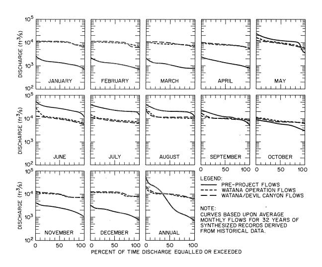
Figure H.2-5. Flow duration curves at Gold Creek for pre-project, Watana, and Watana-Devil Canyon operational flows. Source: Exhibit E, Figures E.2.160 and E.2.208.
