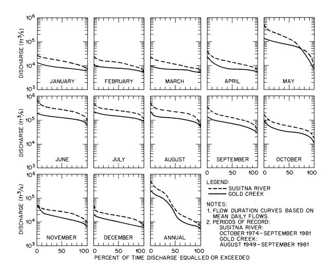
Figure H.2-3. Pre-project flow duration curves for the Gold Creek and Sunshine gaging stations based on mean daily flows. Source: Exhibit E, Figure E.2.39.
