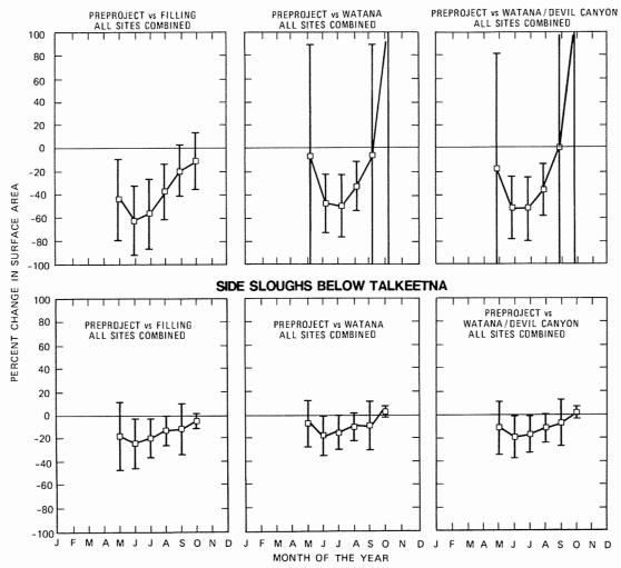
Figure H.3-2. Response of Zone H-II wetted surface area to mainstem flows. Source: ADFG 1983.
