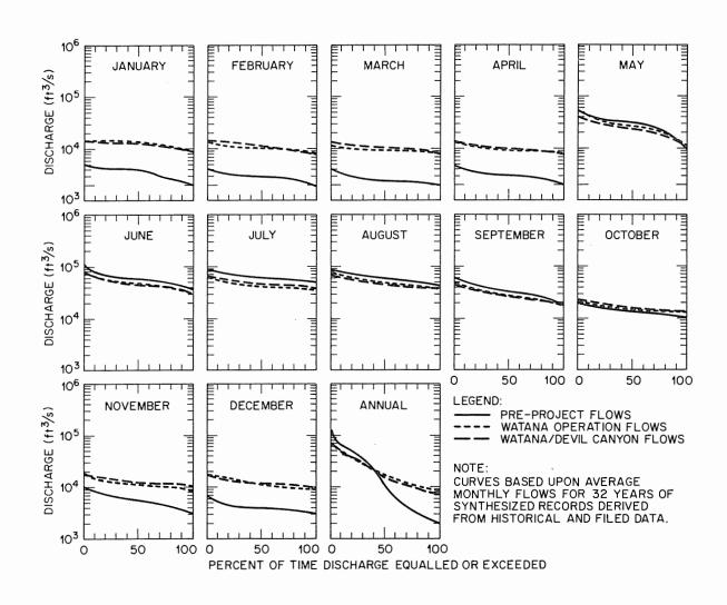
Figure H.2-6. Flow duration curves at Sunshine for pre-project, Watana, and Watana-Devil Canyon operational flows. Source: Exhibit E, Figures E.2.161 and E.2.209.
