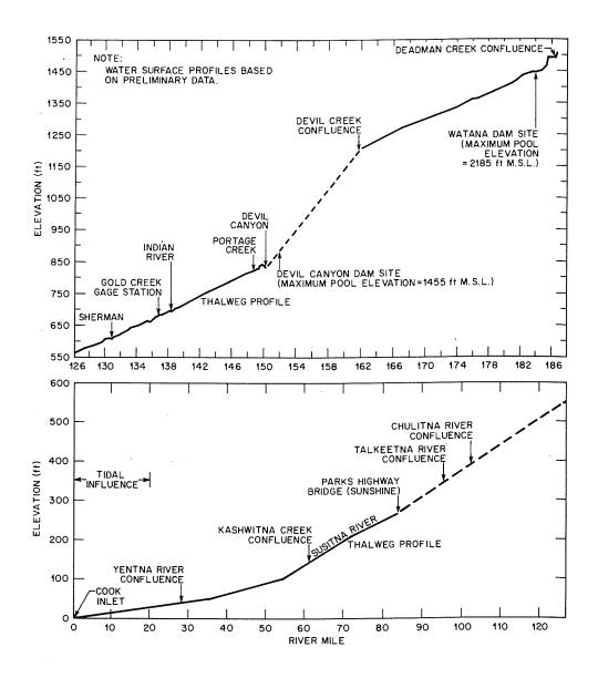
Figure H.1-2. Longitudinal profile of the mainstem of the Susitna River. Source: Redrawn from Exhibit E, Figures E.2.6, E.2.7, and E.2.9.
