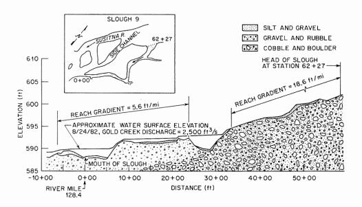
Figure H.1-5. Morphology of a typical side-channel slough. Source: Exhibit E, Figure E.2.21.
