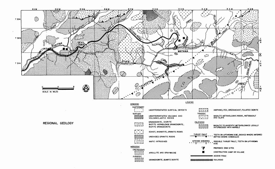
Figure E-4. Regional Geology Underlying Site Features. [Source: Exhibit E, Vol. 7, Chap. 6, Fig. E-6.1] At the proposed Watana dam site the dioritic pluton is generally massive in texture and competent. Small discontinuous alteration zones, fraction zones, and shears, as well as two major and two minor joint sets, have been found at the site. The joints are generally steep and many follow the structural trend of the region.
