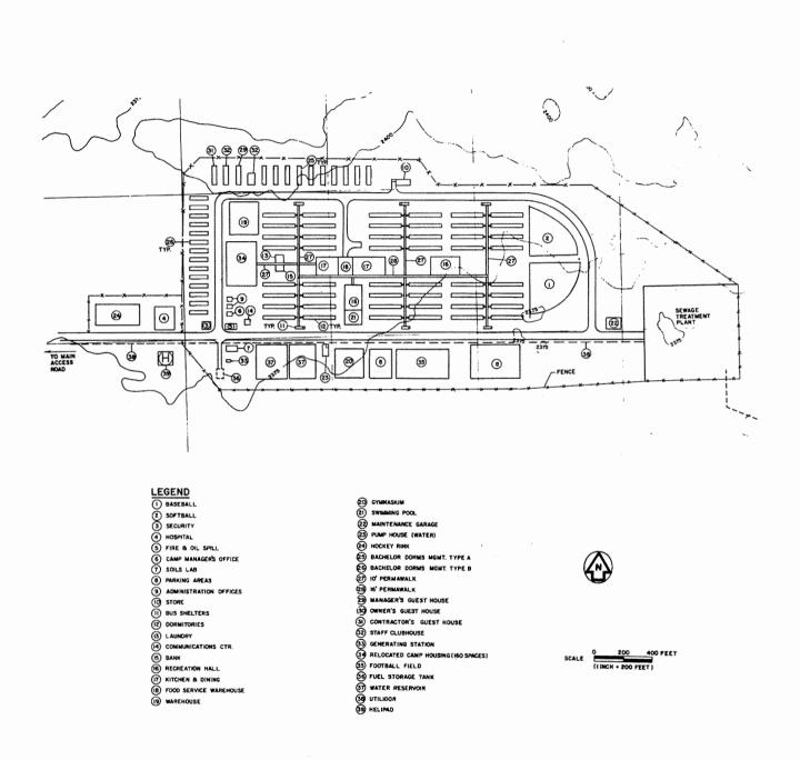
Figure F-5. Proposed Watana Construction Camp. [Source: Exhibit F, Vol. 3, Plate F36]
