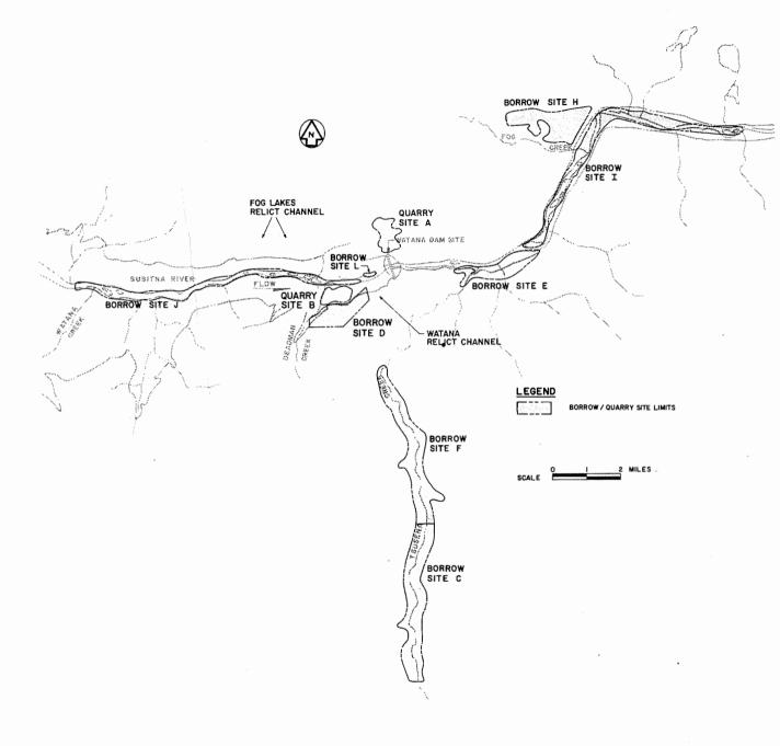
Figure E-2. Watana Borrow/Quarry Sites. [Source: Exhibit E, Vol. 9, Chap. 10, Fig. E.10.13]
