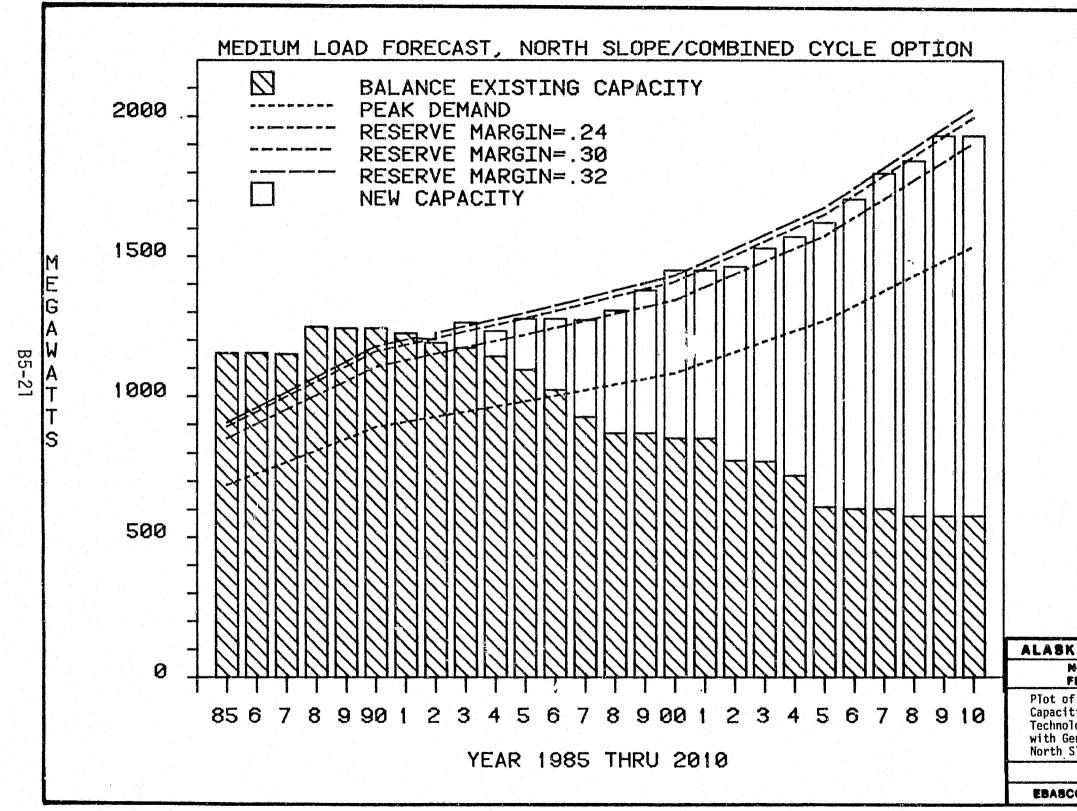
ALASKA POWER AUTHORITY NORTH SLOPE GAS Plot of System Requirements and Capacities for Combined Cycle Technology, Medium Load Forecast, with Generating Facilities at the North Slope. FIGURE 85-10 EBASCO SERVICES INCORPORATED
