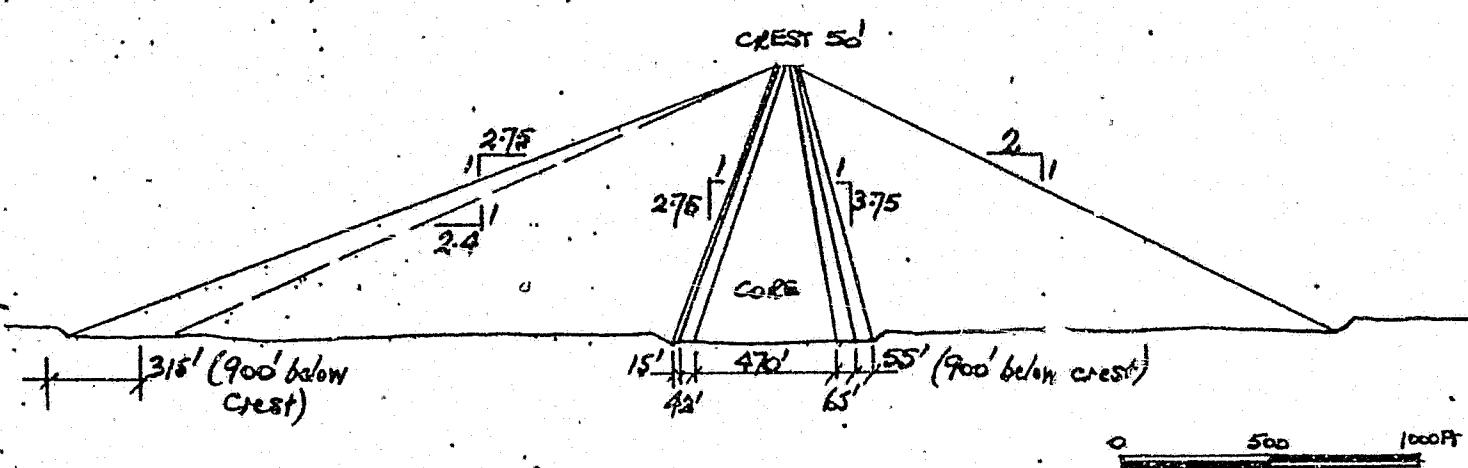
$$\text{CORE THICKNESS} = 20 + 0.5 \text{ DEPTH BELOW CREST}$$
