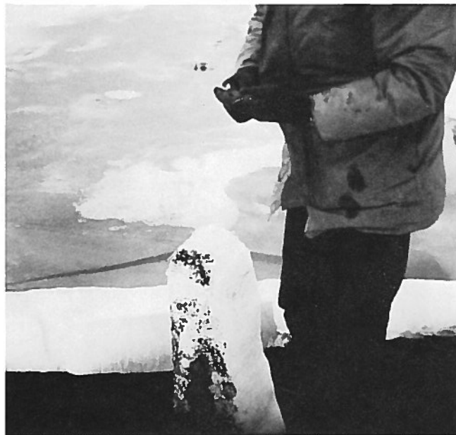
Figure 9. Sediment frozen to the bottom of ice laid down onto the reservoir bed (February 1974, Lake Koocanusa, Montana).
