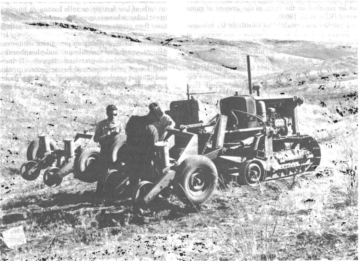
Fig. 20.1. Two Hansen browse seed drills hooked on a tandem bar behind a tractor. The purpose of this arrangement was to drill over 1020 ha burned by wildfire on critical deer ranges. (U.S. Bureau of Land Management photo by Jim Yoakum.)
