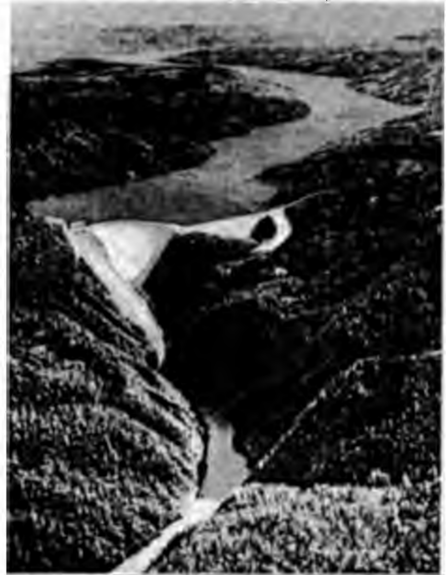
The Watana dam would be an earth-fill structure 885 feet high, 4100 feet long, with an installed capacity of 1020 MW. The Devil Canyon dam would be a concrete arch dam 645 feet high, about 1500 feet long at the crest, with an installed capacity of 600 MW. The Watana dam would create a reservoir 48 miles long; Devil Canyon a reservoir 28 miles long.
