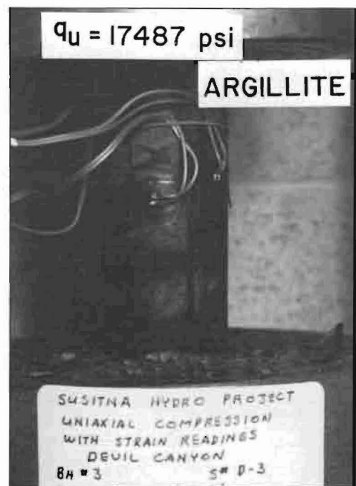
TYPICAL COMPRESSION TEST WITH STRESS-STRAIN READINGS
