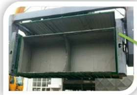
Lid Lifted & internal reinforcement
