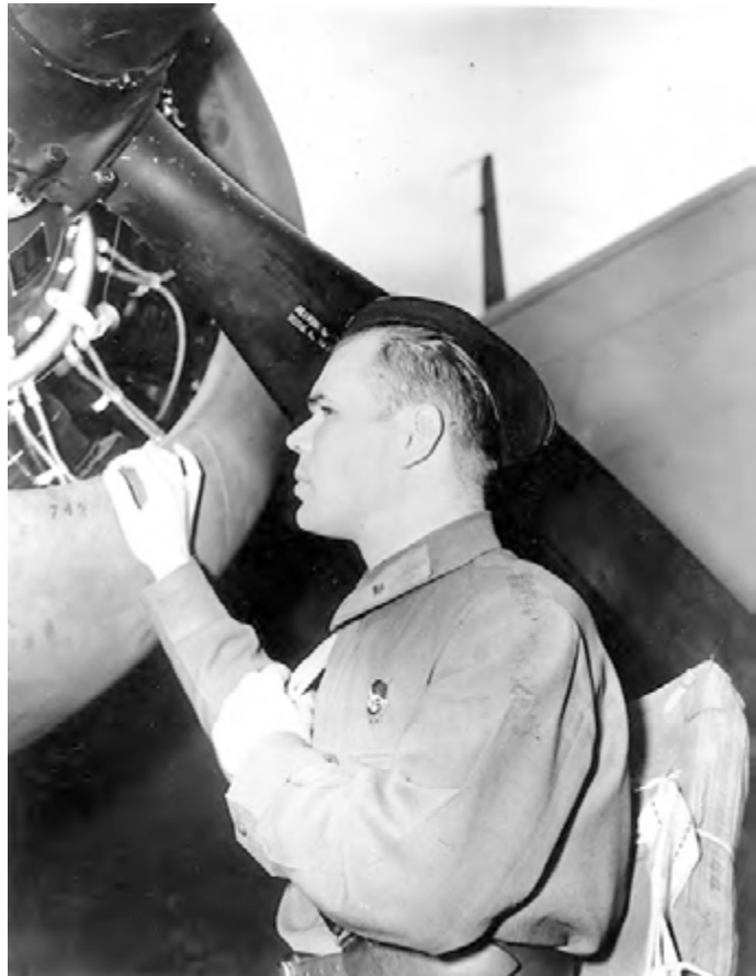
Soviet airman examines the Wright Double Cyclone R-2600 engine of a Douglas A-20 as part of his pre-flight check before ferrying the airplane into Russia. Photo: USAF via Blake W. Smith.
