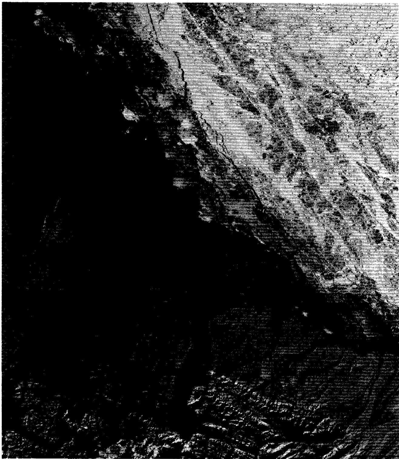
Figure 1: This is a band 7 Landsat scene (of the Beaufort Sea Lease Area) taken at 2015 hours local time on July 7, 1977. The satellite was on the ascending node of its orbit. The sunlight is from the north at a low angle. This low-angle north lighting provides a good enhancement of minor geomorphic features. Temperature 43°F, Wind was from 070° at 8.8 mph.
