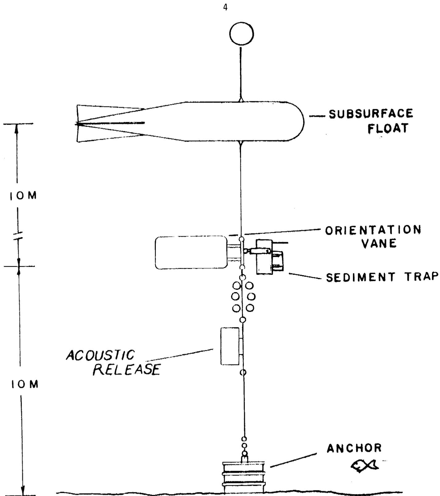
Figure 1. Diagram of Sediment Trap Mooring.
