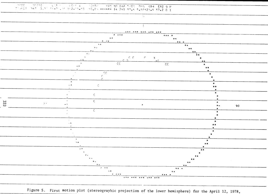
magnitude 5.8 earthquake off Kodiak Island. (C = compression, B = two compression, X = one dilitation and one compression)
