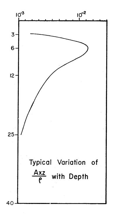
Figure 1. Typical variation of the eddy viscosity with depth.
