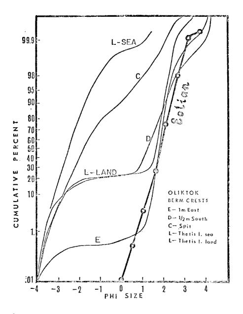
Figure 5. Grain size distribution of eolian sediment in Egg Island plume, superimposed on curves representing berm crest sediments from the Oliktok area (Figure 3) with depositional environment similar to that of Egg Island. (Figure modified after Dygas, et.al., 1972).
