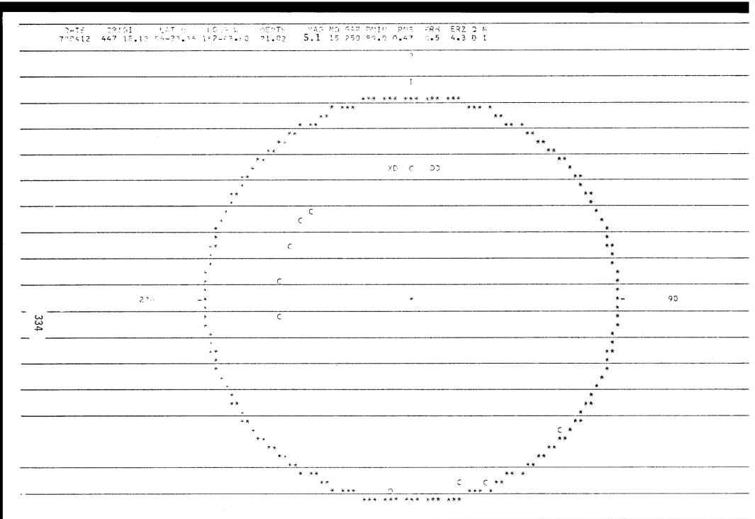
Figure 6. First motion plot (stereographic projection of the lower hemisphere) for the April 12, magnitude 5.1 aftershock of 0447.
