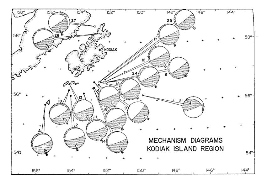
Figure 3. Mechanism diagrams (stereographic projections) of earthquakes in the Kodiak Island region. Shaded areas represent rarefaction quadrants; arrows represent direction of P (pressure) axes(from Stauder and Bollinger).
