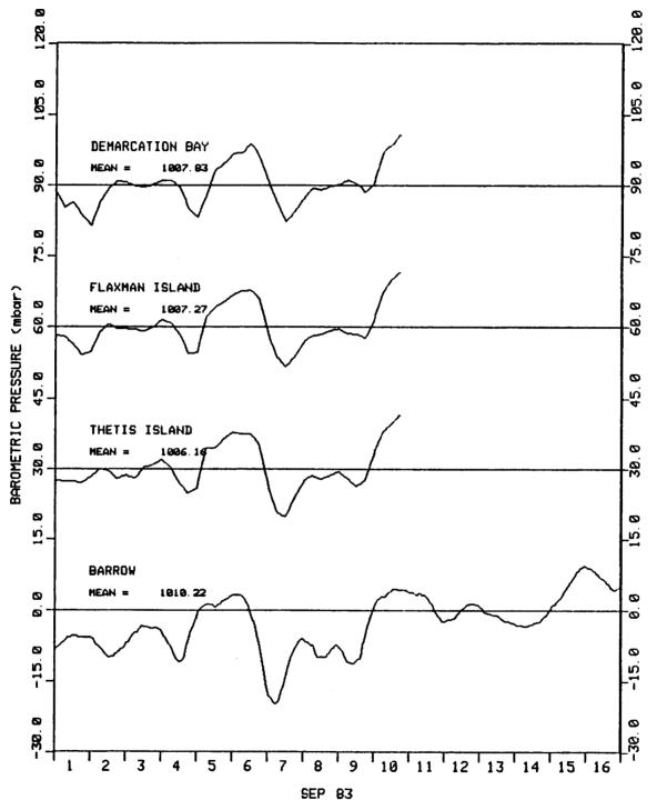
Fig. 16. Barometric Pressure Fluctuations Used to Correct Absolute Pressure Data from Stations 5 through 8 in September 1983
