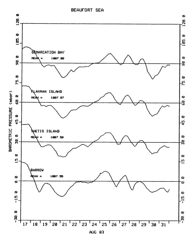
Fig. 15. Barometric Pressure Fluctuations Used to Correct Absolute Pressure Data from Stations 5 through 8 in August 1983 (contd)
