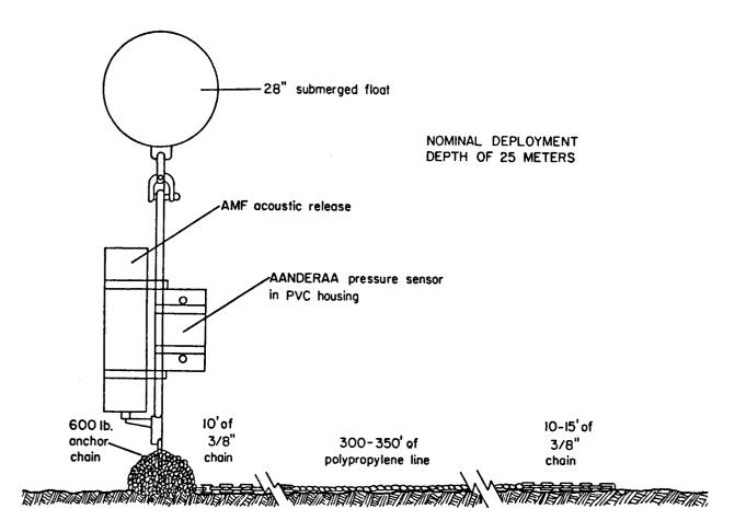
Figure 3 Mooring Design for Norton Sound and Chukchi Sea Deployments
