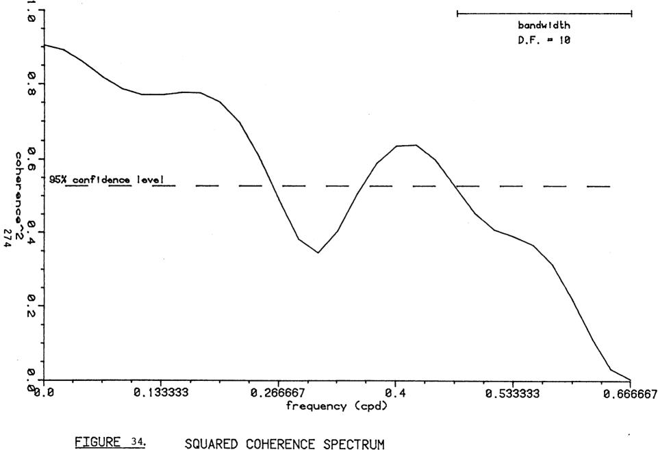
PT. BARROW-CAPE LISBURNE BAROMETRIC PRESSURE DIFFERENCES VS. INSHORE BARROW (BOTTOM) DRIFT CURRENT (35.9 DEGREE COMPONENT) 0659 8 AUG 1981 - 0659 4 SEPT 1981
