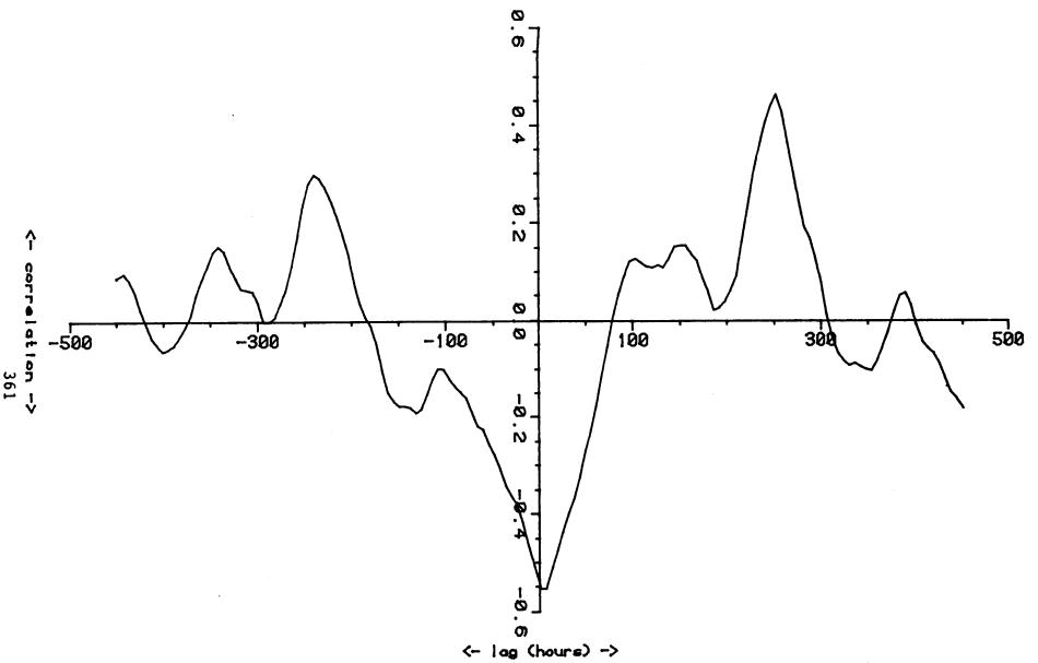
FIGURE A-44 CROSS CORRELATIONS PT. BARROW-CAPE LISBURNE BAROMETRIC PRESSURE DIFFERENCES VS. LAGGED PT. BARROW WIND (35.9 DEGREE COMPONENT) 0158 1 AUG 1981 - 1358 4 SEPT 1981
