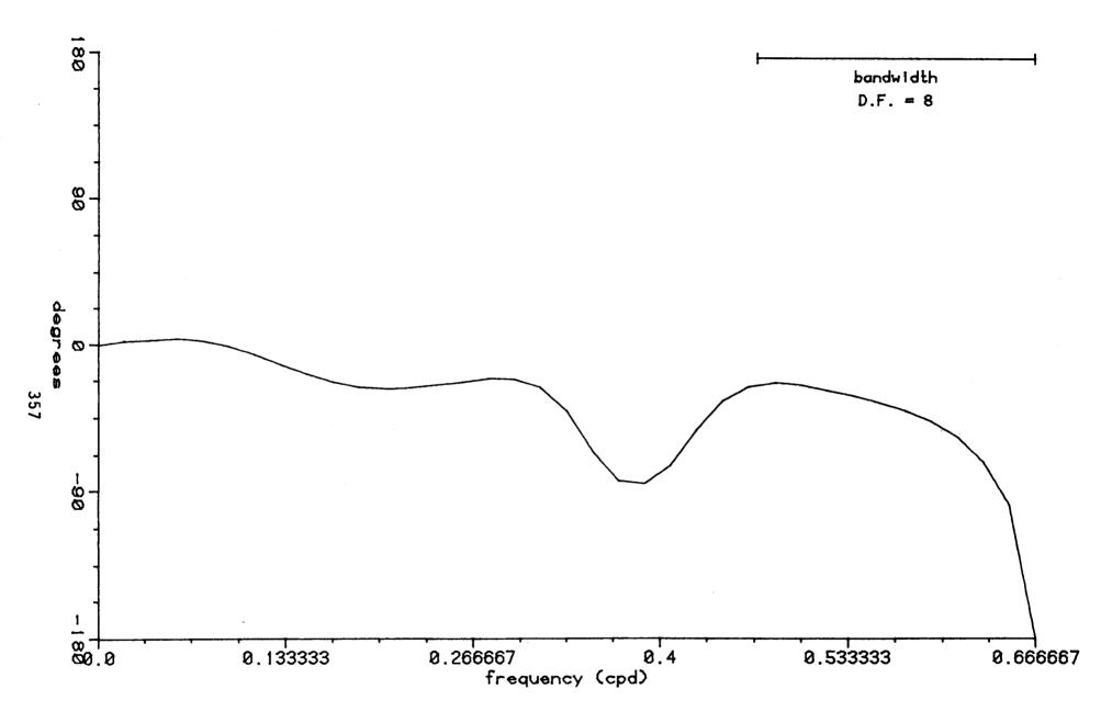
EIGURE A-43 PHASE SPECTRUM WAINWRIGHT WIND (33.7 DEGREE COMPONENT) VS. INSHORE WAINWRIGHT (BOTTOM) DRIFT CURRENT (33.7 DEGREE COMP.) 1751 12 AUG 1981 - 1751 1 SEPT 1981
