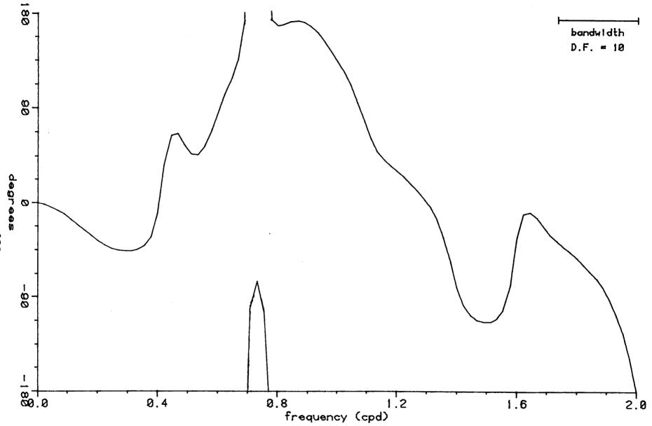
EIGURE A-41 PHASE SPECTRUM WAINWRIGHT WIND (33.7 DEGREE COMPONENT) VS. INSHORE WAINWRIGHT (BOTTOM) DRIFT CURRENT (33.7 DEGREE COMP.) 1751 12 AUG 1981 - 1751 1 SEPT 1981
