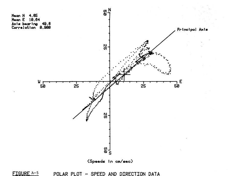
POLAR PLOT - SPEED AND DIRECTION DATA OFFSHORE BARROW (BOTTOM) DRIFT CURRENT 1010 8 AUG 1981 - 1610 7 SEPT 1981
