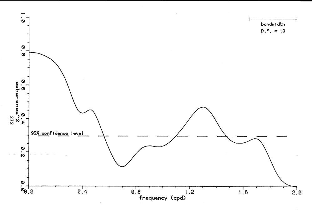
FIGURE 32. SQUARED COHERENCE SPECTRUM PT. BARROW-CAPE LISBURNE BAROMETRIC PRESSURE DIFFERENCES VS. INSHORE BARROW (BOTTOM) DRIFT CURRENT (35.9 DEGREE COMPONENT) 0659 8 AUG 1981 - 1859 4 SEPT 1981
