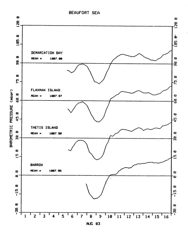
Fig. 15. Barometric Pressure Fluctuations Used to Correct Absolute Pressure Data from Stations 5 through 8 in August 1983
