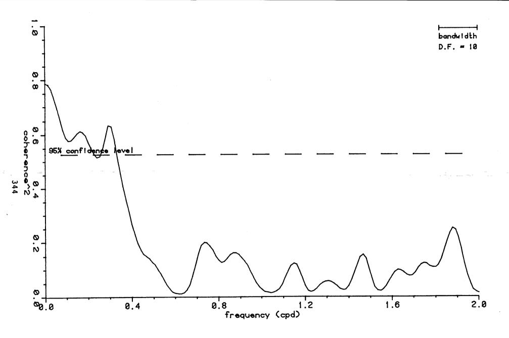
FIGURE A-33 SQUARED COHERENCE SPECTRUM PT. BARROW WIND (35.9 DEGREE COMPONENT) VS. INSHORE BARROW (BOTTOM) DRIFT CURRENT (35.9 DEGREE COMPONENT) 0700 8 AUG 1981 - 1300 6 SEPT 1981
