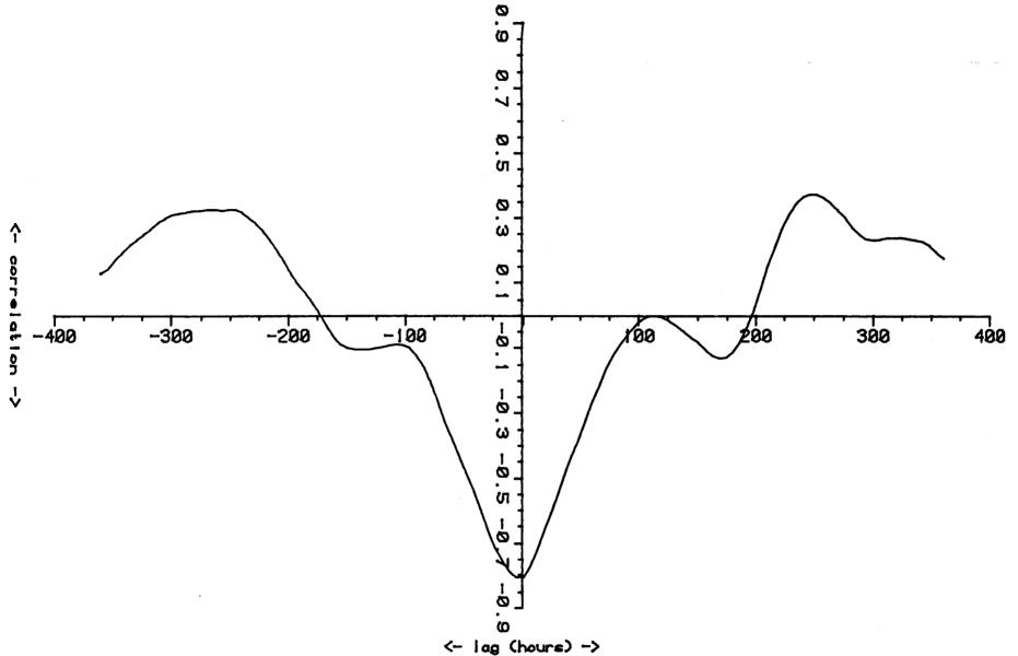
FIGURE A-25 CROSS CORRELATIONS BARROW-LISBURNE BAROMETRIC PRESSURE DIFFERENCES VS. LAGGED INSHORE WAINWRIGHT (BOTTOM) DRIFT CURRENT (33.7 DEG. COMP.) 1350 12 AUG 1981 - 1350 1 SEPT 1981
