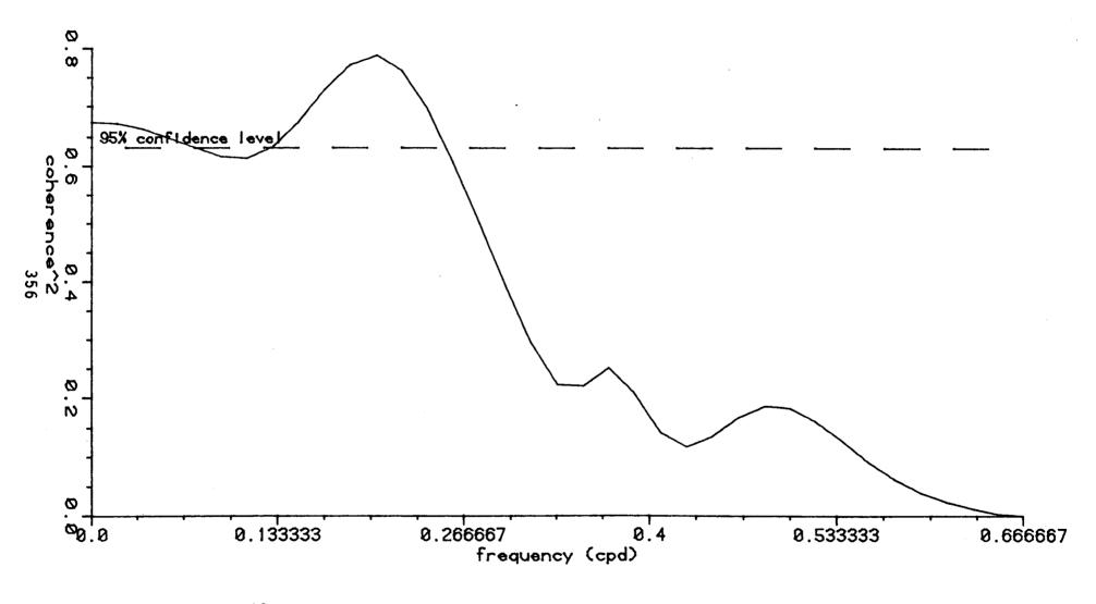
FIGURE A-42 SQUARED COHERENCE SPECTRUM WAINWRIGHT WIND (33.7 DEGREE COMPONENT) VS. INSHORE WAINWRIGHT (BOTTOM) DRIFT CURRENT (33.7 DEGREE COMP.) 1751 12 AUG 1981 - 1751 1 SEPT 1981
