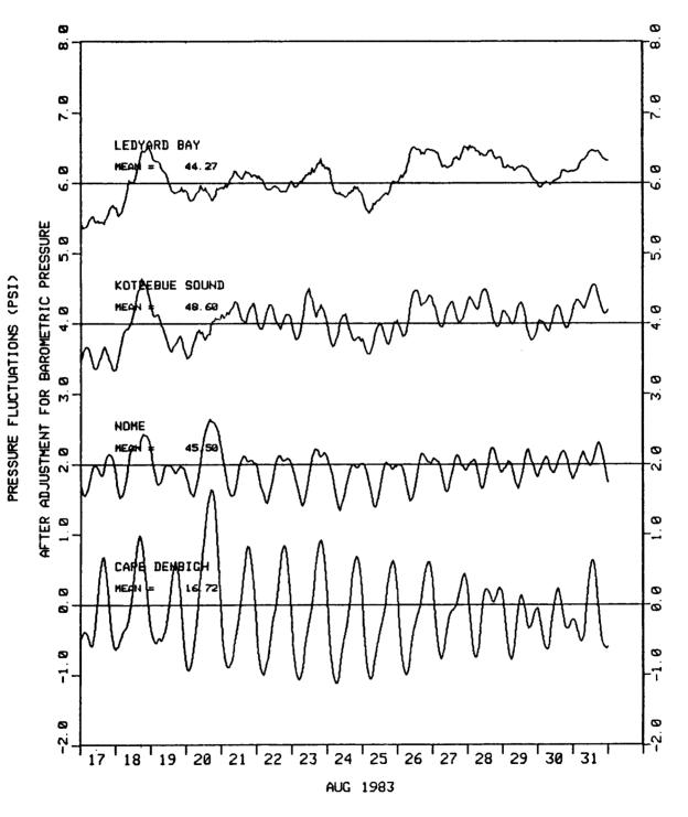
Fig. 5. Pressure Fluctuations About the Monthly Mean at Stations 1 through 4 in August 1983 (contd)
