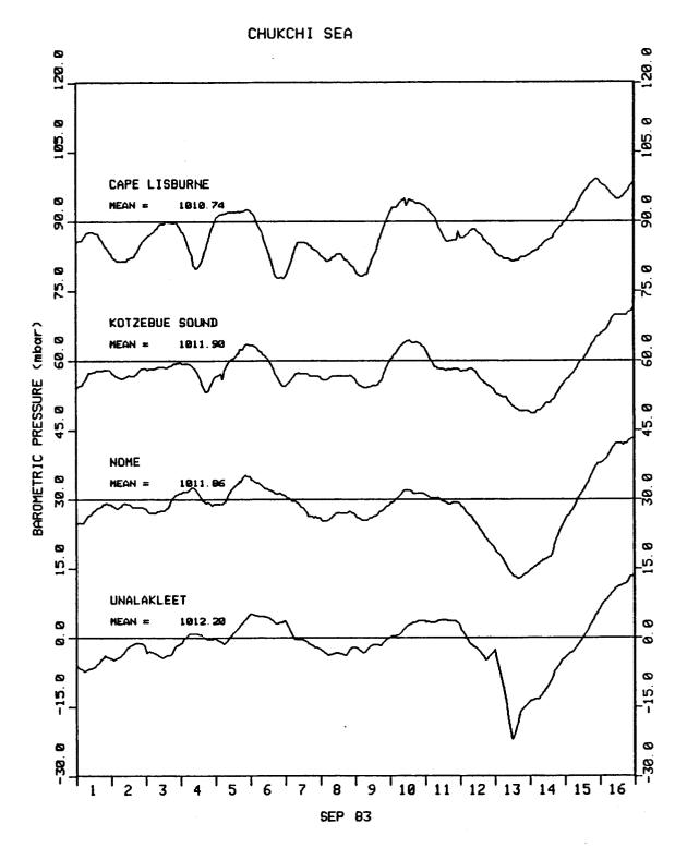
Fig. 14. Barometric Pressure Fluctuations Used to Correct Absolute Pressure Data from Stations 1 through 4 in September 1983
