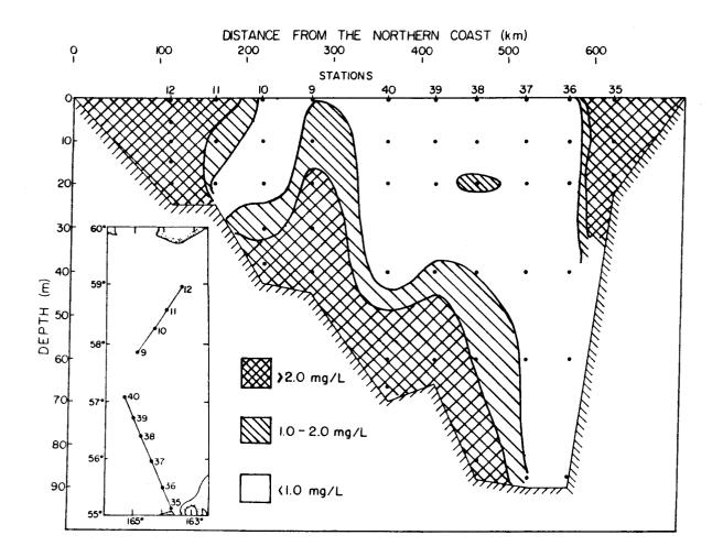
Figure 36. Vertical cross-section of the distribution of total suspended matter for stations 9 thru 12 and 35 thru 40 in the southeastern Bering Shelf (Cruise RP-4-Di-75B-III, 12 September - 5 October 1975).
