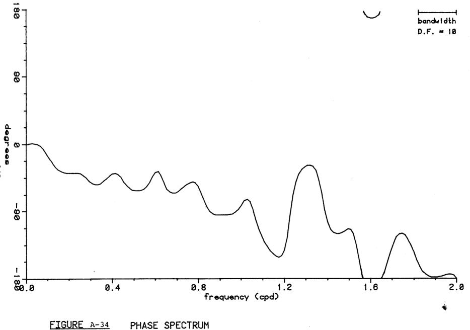
PHASE SPECTROM PT. BARROW WIND (35.9 DEGREE COMPONENT) VS. INSHORE BARROW (BOTTOM) DRIFT CURRENT (35.9 DEGREE COMPONENT) 0700 8 AUG 1981 - 1300 6 SEPT 1981
