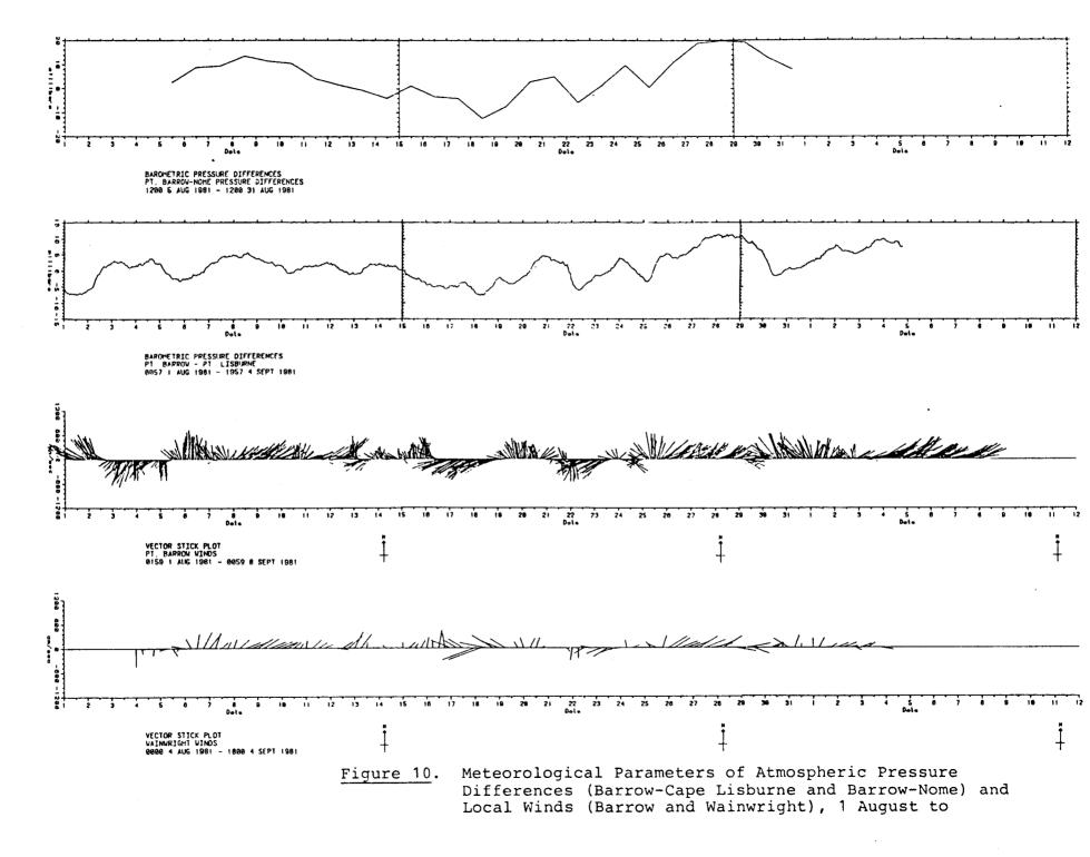
through August 1981 (Figure 10). Noticeable divergence in the trend occurs during 6 - 10 August, when greater differences were recorded between Barrow and Nome than between Barrow and Lisburne. The divergence occurs when westward moving high pressure areas create large differences between Nome and Lisburne leaving a series of isobars between the two areas (Figure 11).
