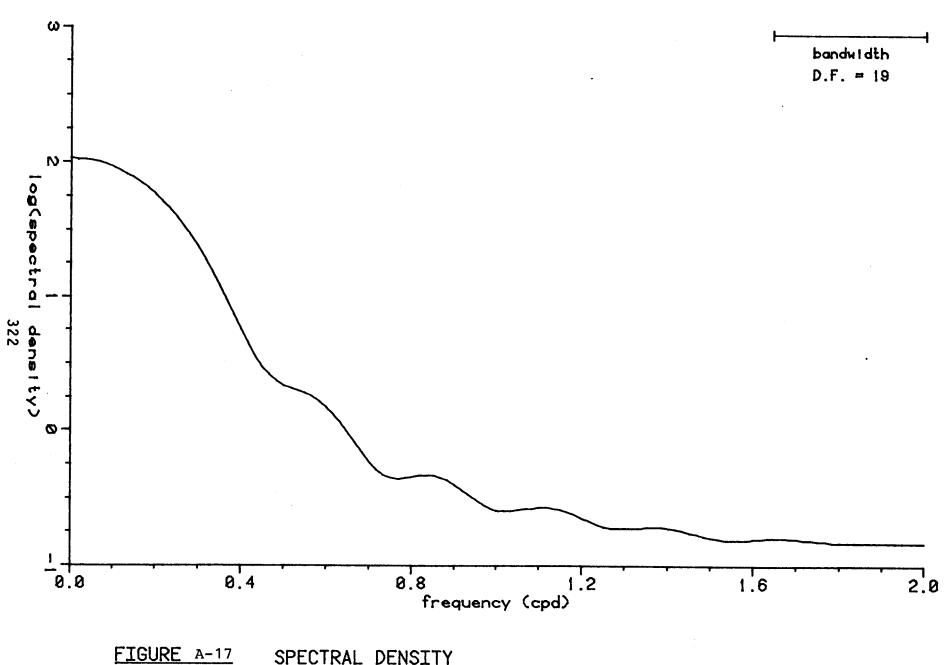
SPECTRAL DENSITY INSHORE BARROW (BOTTOM) DRIFT CURRENT (35.9 DEGREE COMPONENT) 0659 8 AUG 1981 - 1859 4 SEPT 1981
