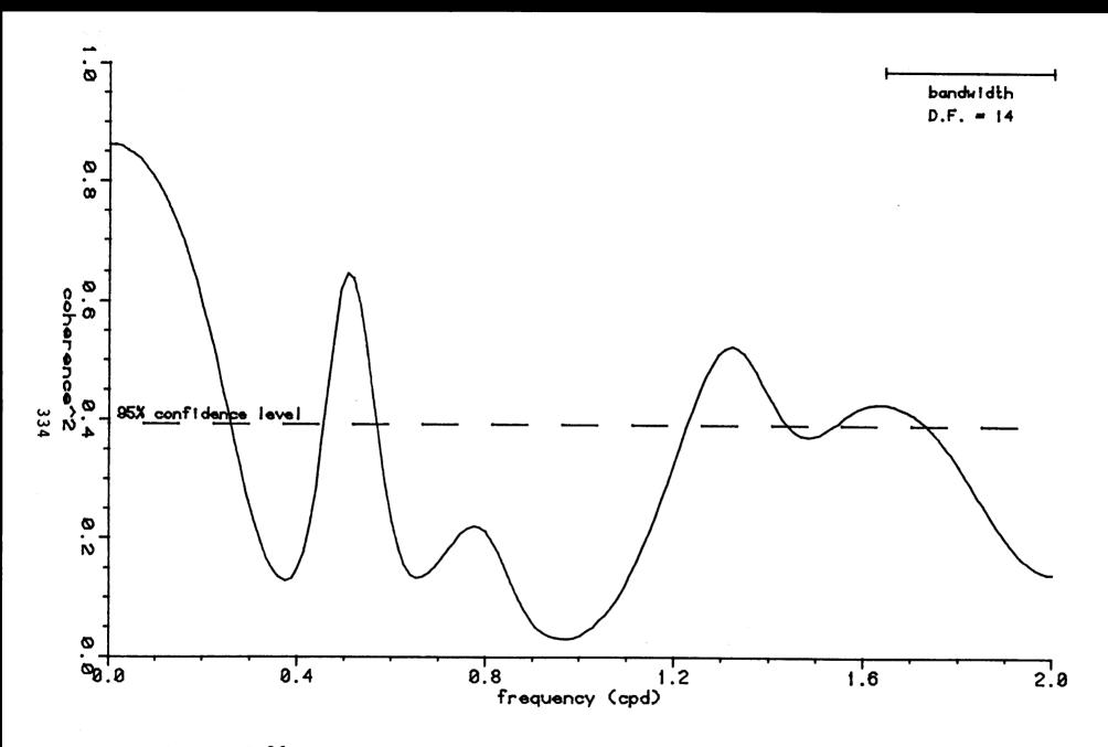
EIGURE A-26 SQUARED COHERENCE SPECTRUM BARROW-LISBURNE PRESSURE DIFFERENCES VS. INSHORE WAINWRIGHT (BOTTOM) DRIFT CURRENT (33.7 DEGREE COMPONENT) 1350 12 AUG 1981 - 1350 1 SEPT 1981
