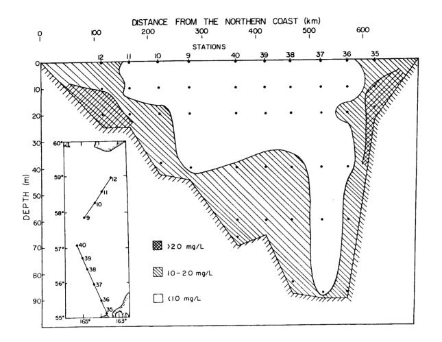
Figure 37. Vertical cross-section of the distribution of total suspended matter for stations 9 thru 12 and 35 thru 40 in the southeastern Bering Shelf (Cruise RP-4-MW-76B-VIII, 24 June -9 July 1976). in which the sum of the major inorganic element concentrations is also greater than 60 percent of the total weight. Group III contains all the stations in between in which the sum is less than 60 percent of the total suspended load.
