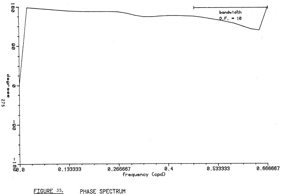
PHASE SPECTRUM PT. BARROW-CAPE LISBURNE BAROMETRIC PRESSURE DIFFERENCES VS. INSHORE BARROW (BOTTOM) DRIFT CURRENT (35.9 DEGREE COMPONENT) 0659 8 AUG 1981 - 0659 4 SEPT 1981
