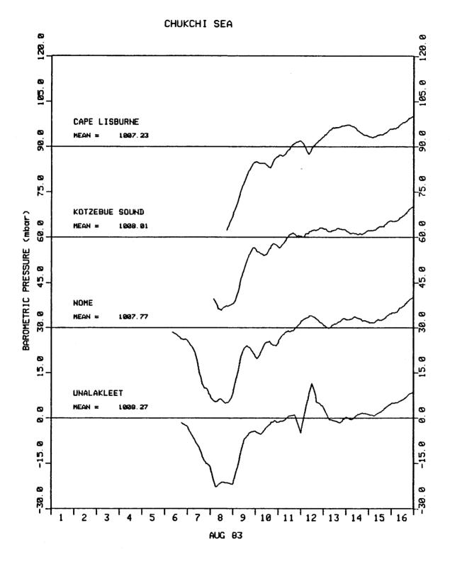
Fig. 13. Barometric Pressure Fluctuations Used to Correct Absolute Pressure Data from Stations 1 through 4 in August 1983
