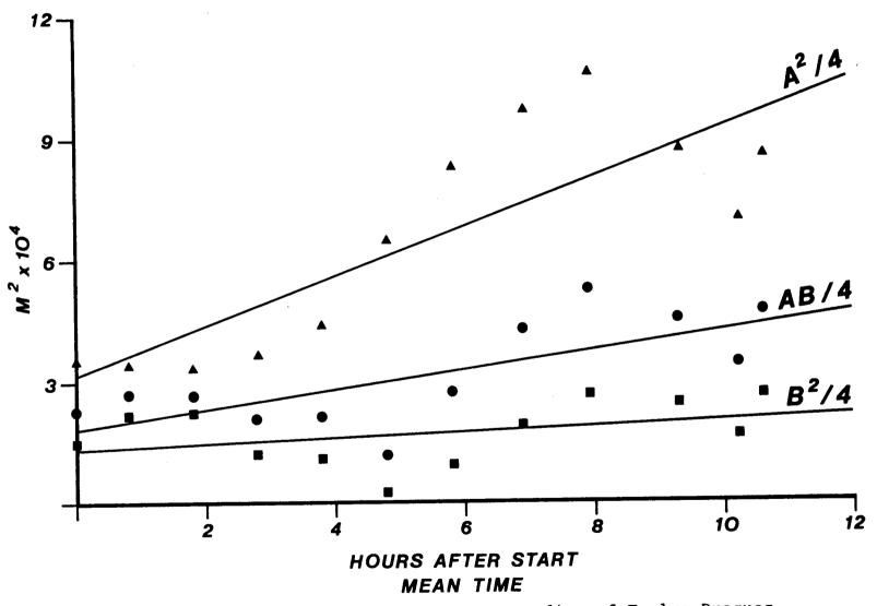
Figure 21. Variances Calculated From The Spreading of Twelve Drogues
