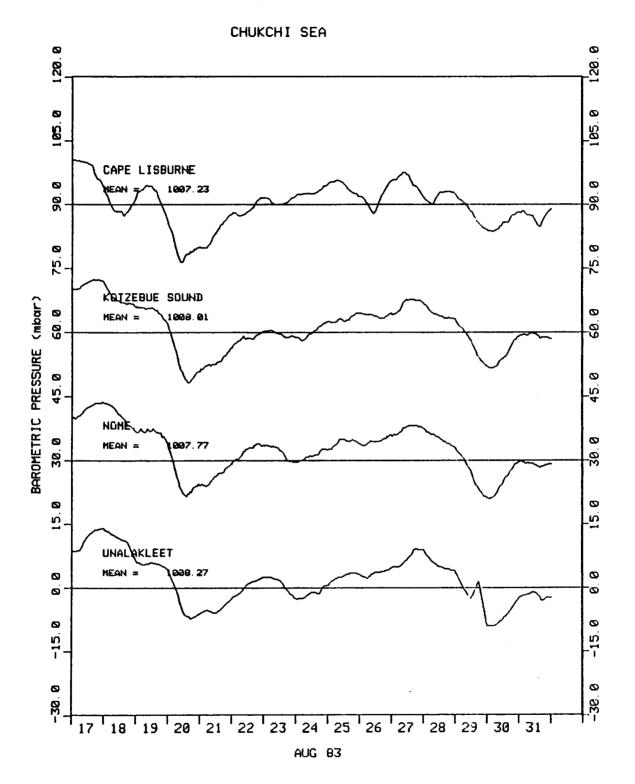
Fig. 13. Barometric Pressure Fluctuations Used to Correct Absolute Pressure Data from Stations 1 through 4 in August 1983 (contd)
