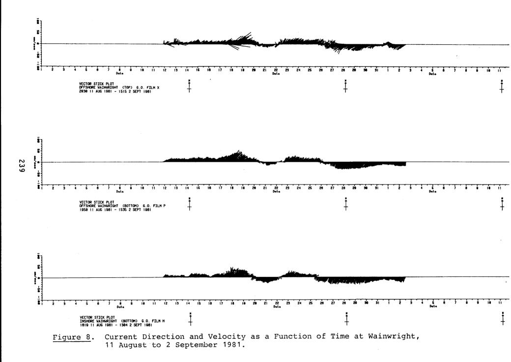
station show a similar pattern of current direction, but emphasize a difference in local current velocities. The initial peak in velocity of 8 August is not evident at either bottom station of offshore or inshore Barrow, while the reversal evident in the records of Barrow during 31 August and 1 and 2 September registers as a cessation of current velocity at Wainwright (Figure 8).
