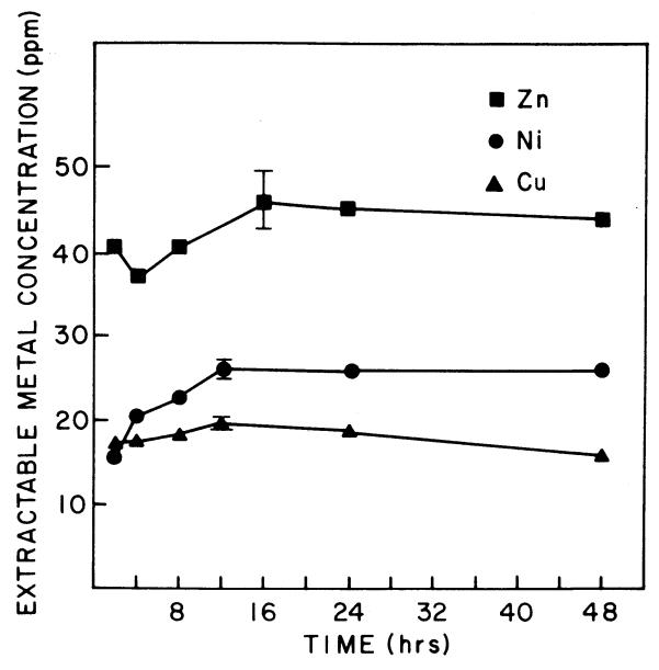
Figure 11. Extractable metal concentrations versus time in contact with 0.3 N HCl for Zn, Ni, and Cu. The range of values is given for duplicate samples at 12 hours.
