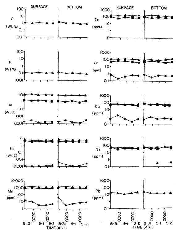
Figure 30. Temporal variations of major and trace elements in suspended matter (total concentration [▲], weak acid extractable [■], and peroxide extractable [●] from station CB-10 in lower Cook Inlet.) Samples were collected 31 August and 1-2 September 1978).
