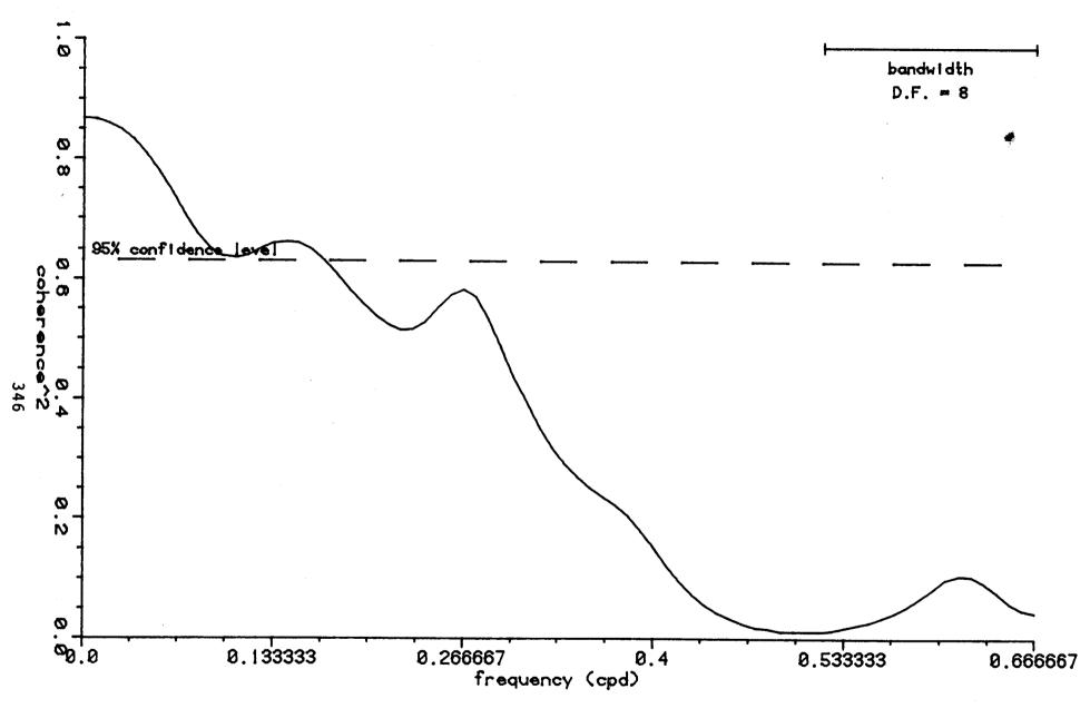
FIGURE A-35 SQUARED COHERENCE SPECTRUM PT. BARROW WIND (35.9 DEGREE COMPONENT) VS. INSHORE BARROW (BOTTOM) DRIFT CURRENT (35.9 DEGREE COMPONENT) 0700 8 AUG 1981 - 1300 6 SEPT 1981
