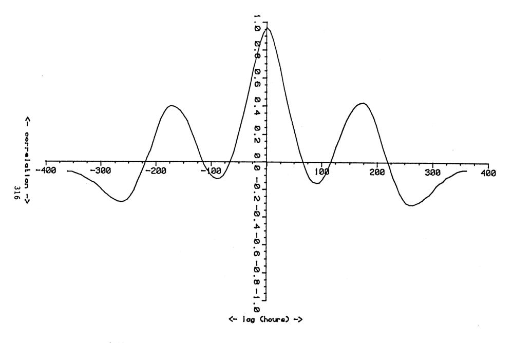
EIGURE A-14 CROSS CORRELATIONS INSHORE BARROW (BOTTOM) DRIFT CURRENT VS. LAGGED INSHORE BARROW (BOTTOM) CURRENT (35.9 DEGREE COMPONENTS) 0703 8 AUG 1981 - 1303 6 SEPT 1981
