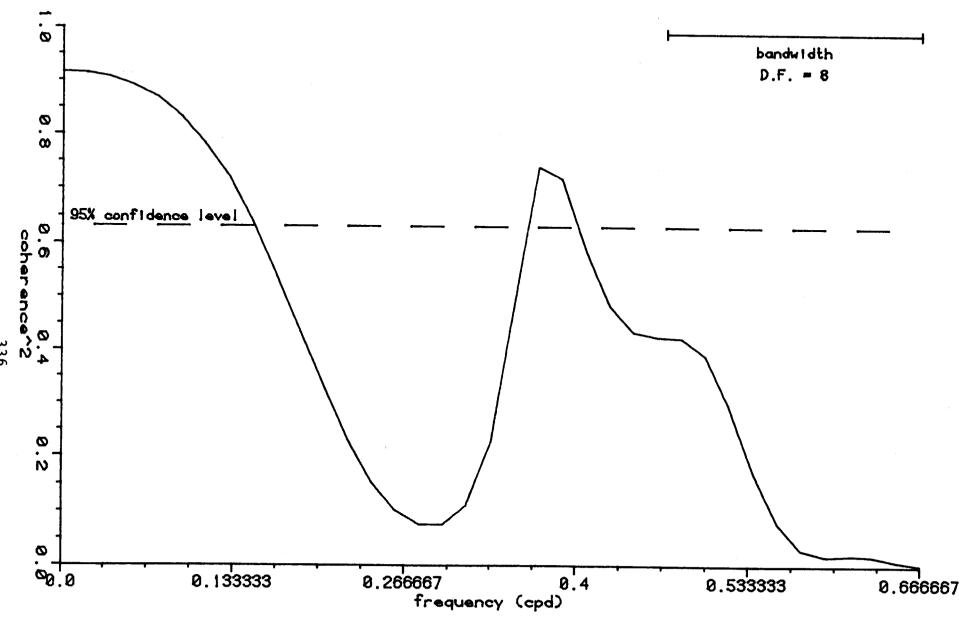
EIGURE A-28 SQUARED COHERENCE SPECTRUM BARROW-LISBURNE BAROMETRIC PRESSURE DIFFERENCES VS. INSHORE WAINWRIGHT (BOTTOM) DRIFT CURRENT (33.7 DEGREE COMP.) 1350 12 AUG 1981 - 0150 1 SEPT 1981
