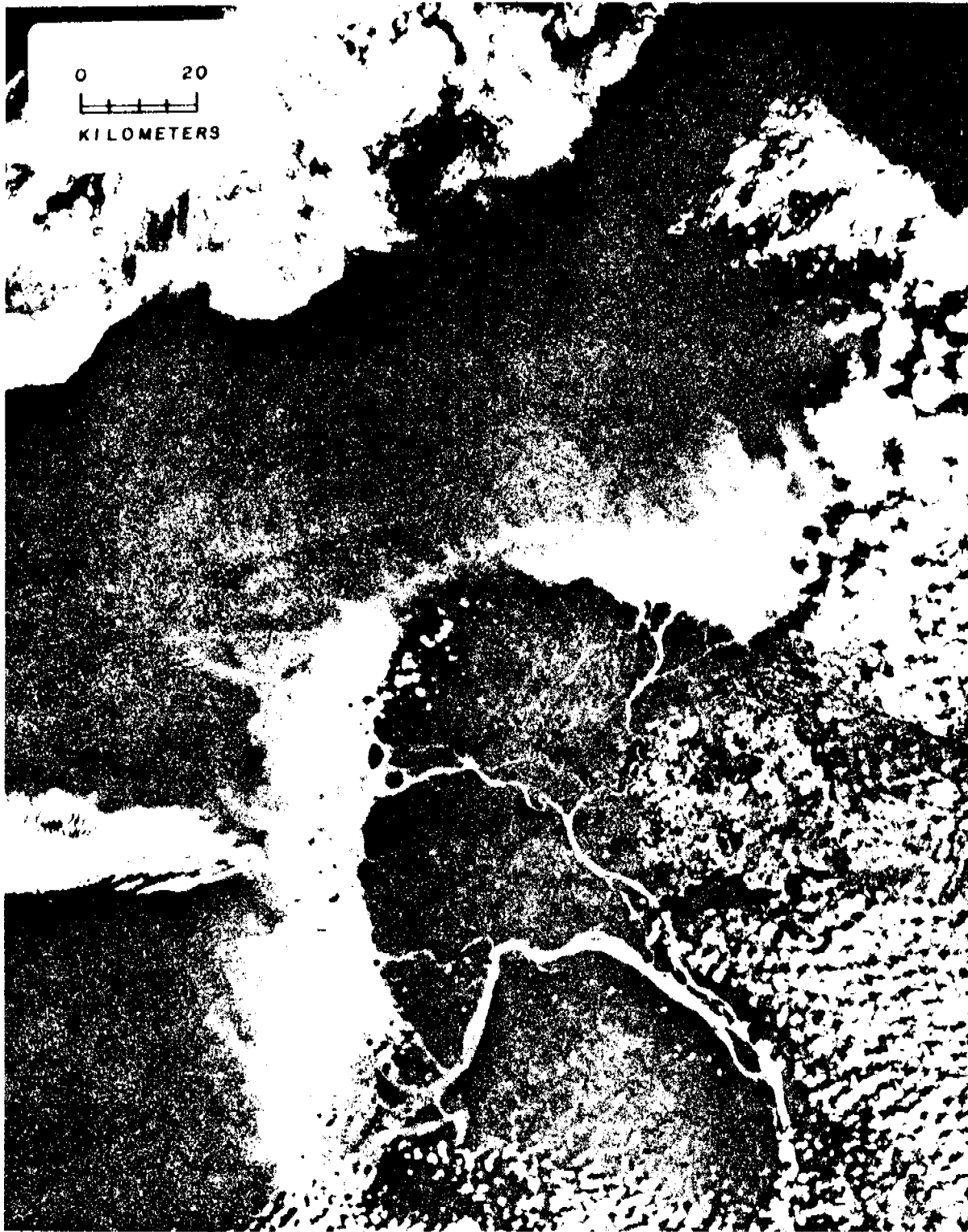
Figure 33. MSS Band 5 of LANDSAT images E-21640-21360-5 and E-21640-21363-5 taken on July 20, 1979, showing evidence for suspended matter (appearing lighter in tone than the less turbid water) transport into Norton Sound.
