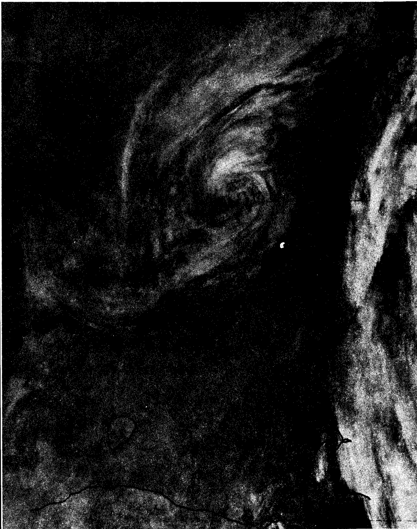
Figure 2. NOAA VHRR infra-red image of the area off western Alaska acquired at 1219 hrs. AST, December 30, 1977. North is approximately at the upper-left corner of the picture. Point Barrow is indicated by the 'x'. Note the lead system along the coast east of Point Barrow.
