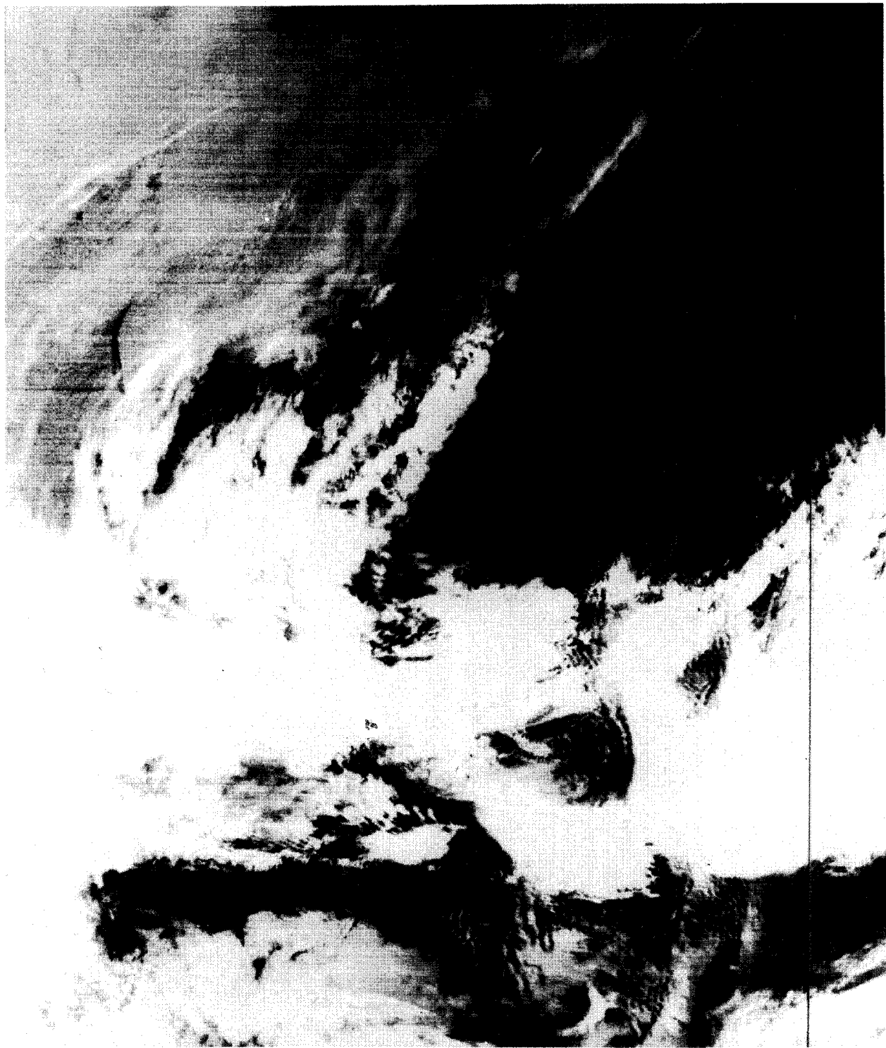
FIGURE 58: This image is identical to that of Figure 57 except that it is in the thermal infrared band (10.5 - 12.5 \mu ). This image is also specifically calibrated to depict both snowfree area (black) and areas at 0° C (stippled white and black). This imagery is quite valuable for monitoring rates and areal extent of snowmelt.
