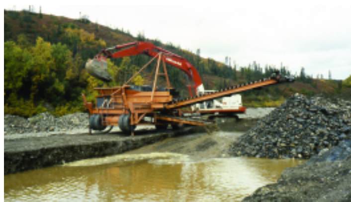
Figure 3: Modern placer mining operation in the early 1980s in the Kantishna area of Denali. An excavator feeds a washplant which cleans and sizes material allowing gold to be trapped in the sluice box.
