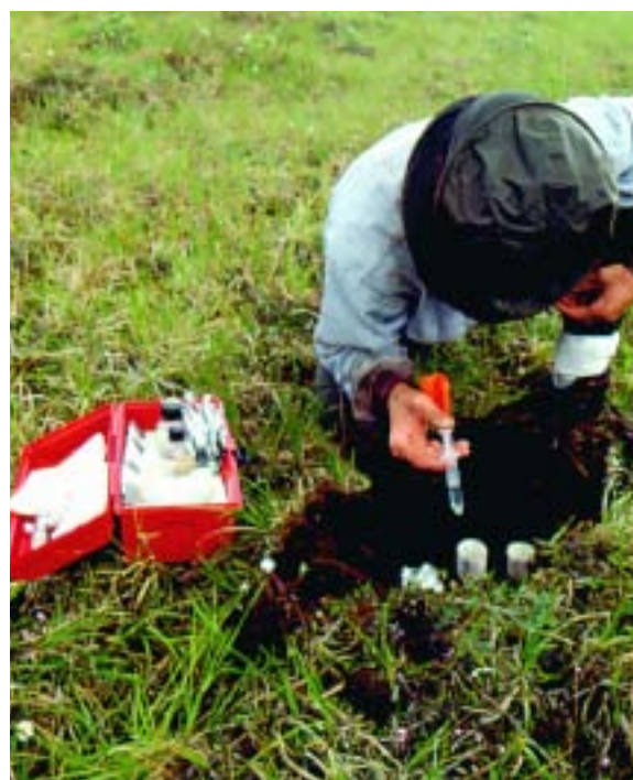
Figure 6. Inoculating soil cores with ^{15}\text{N} to quantify how nitrogen availability might respond to change in soil temperature and moisture in different vegetation types, Asik watershed, Noatak National Preserve.
