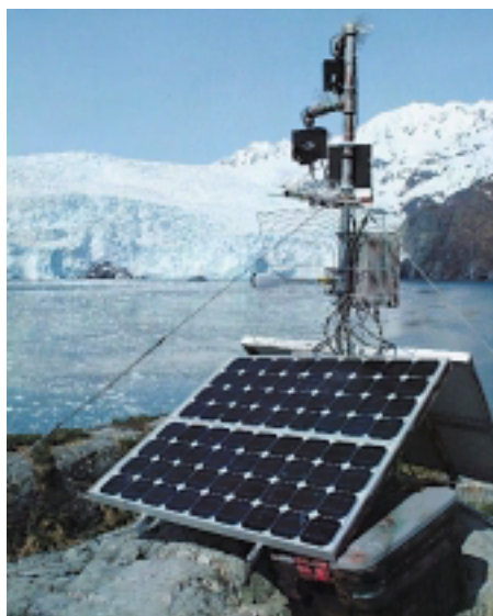
Figure 3. Powered by solar panels and wind-driven generators, three camera stations transmit signals between upper Aialik Bay and the Alaska SeaLife Center.
