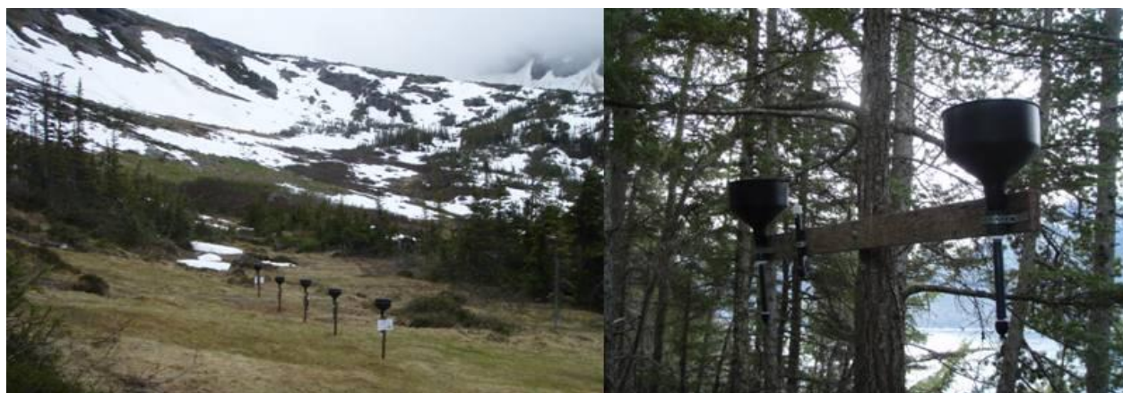
Figure 8. A) Open (or bulk) resin tube deposition sampling array at Upper Dewey, and B) closed canopy (or throughfall) resin tube deposition sampler arrays at Lower Dewey. Open sites had five samplers and one blank while closed sites had ten samplers and one blank.
