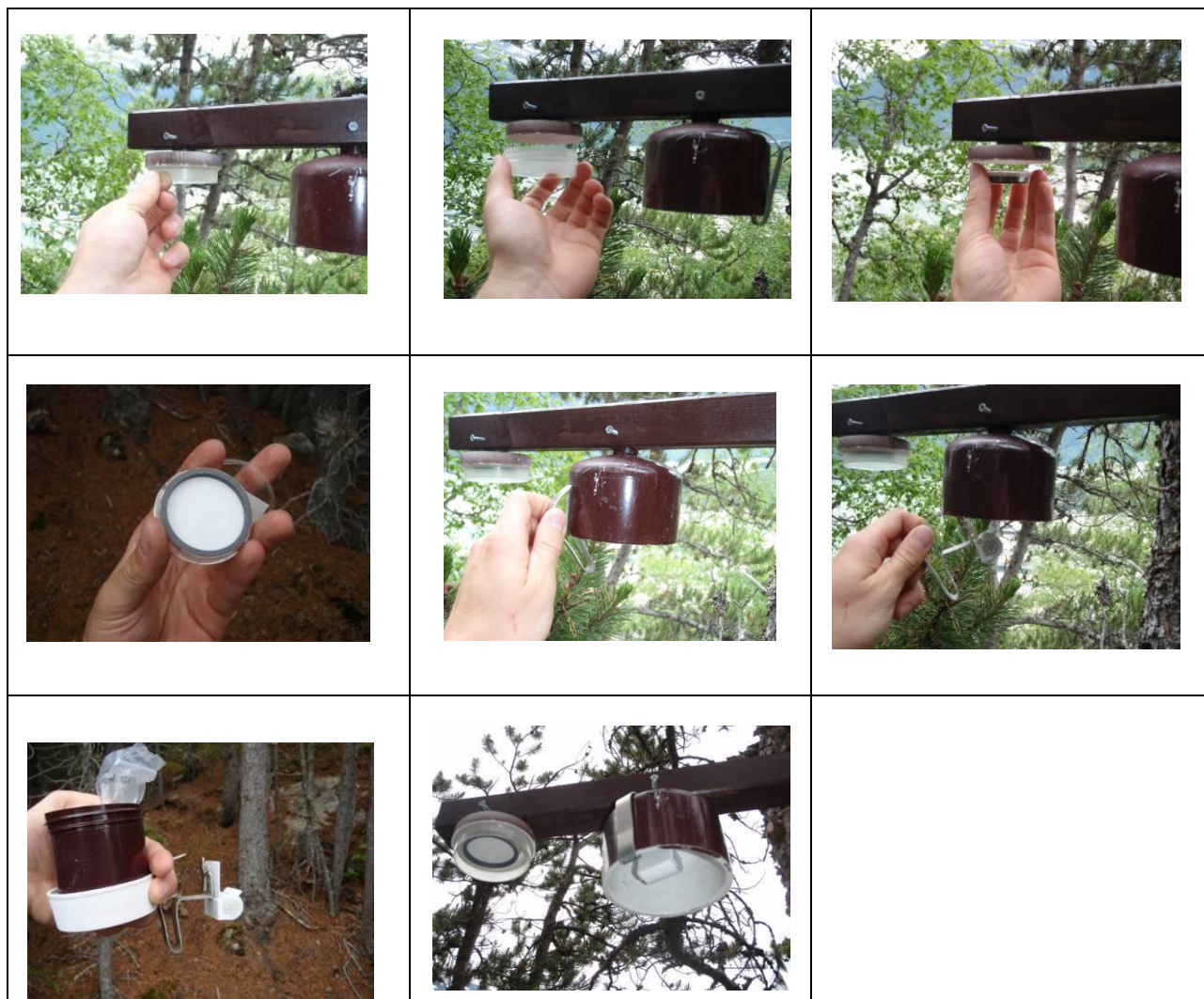
Figure A.1. Removing and replacing membrane sampler filters and Ogawa filter housing.
