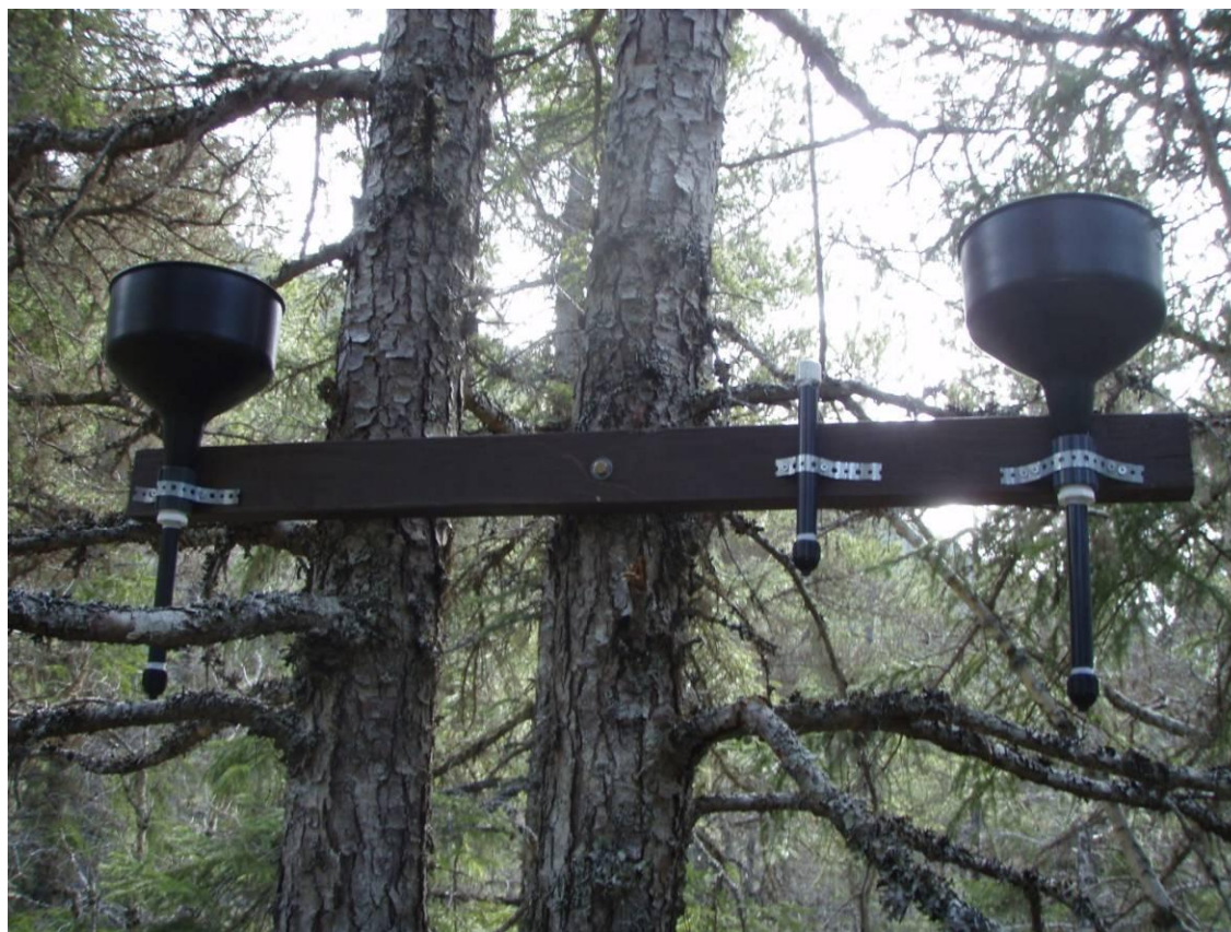
Figure B.5. Throughfall deposition samplers (far left and right) and blank IER column (center).
