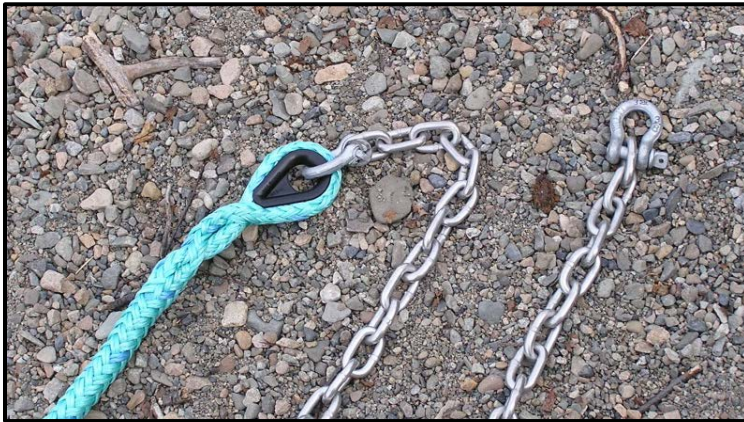
Figure 8.4. Thimble spliced into the lower end of the instrument line. The shackle and anchor chain are attached. The swivel described in Step 3 (above) is not pictured.
