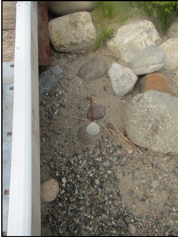
Figure 7.13. Reference point for conducting the “tape down” measurements at Lake Camp, located just upstream of the Naknek Lake Outlet boat dock (KATM).
