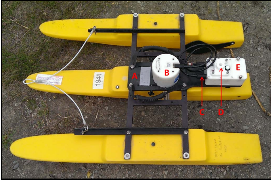
Figure 6.1. Partly assembled ADCP-Trimaran unit, including the instrument mounting plate (A), M9 ADP core unit (B), connection cable (C), attachment point for the DGPS mounting rod (D), and PCM unit (E).
