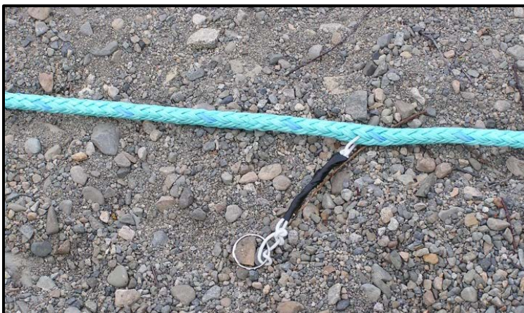
Figure 8.6. Gagnon cord threaded into the instrument line serves as an attachment point for a data logger. Initially, a stainless steel split ring (shown at the distal end of the cord) was used to attach the cord to the logger, but these rings corroded over time so they were omitted from the SOP.
