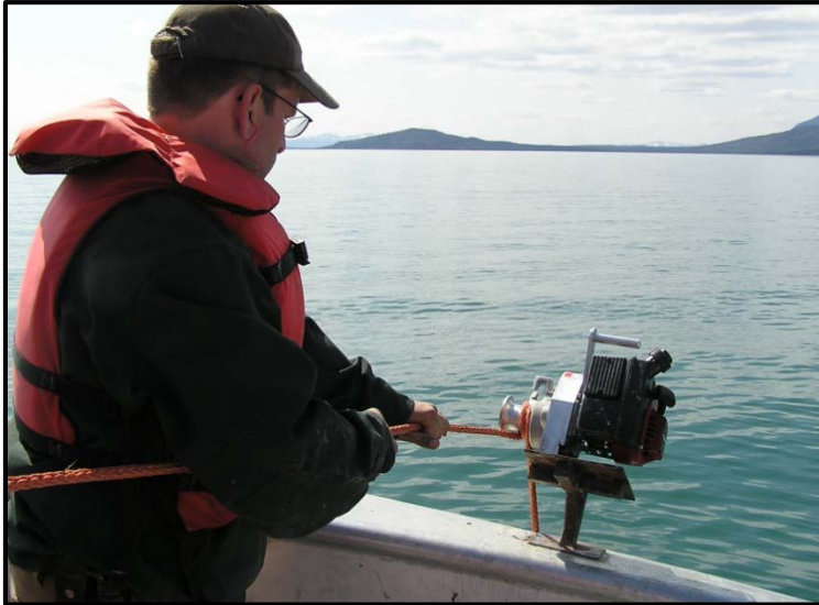
Figure 8.10. Capstan winch and the best position of line with two wraps and slight pressure applied during retrieval.
