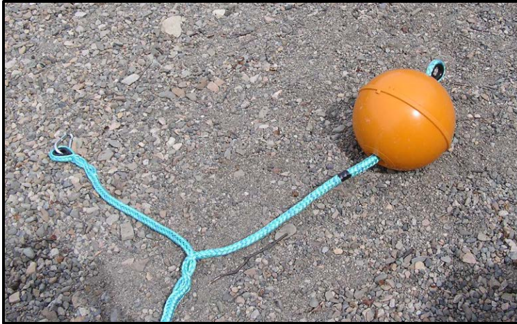
Figure 8.5. Instrument line with submersible buoy and horizontal 1-m long attachment point.
