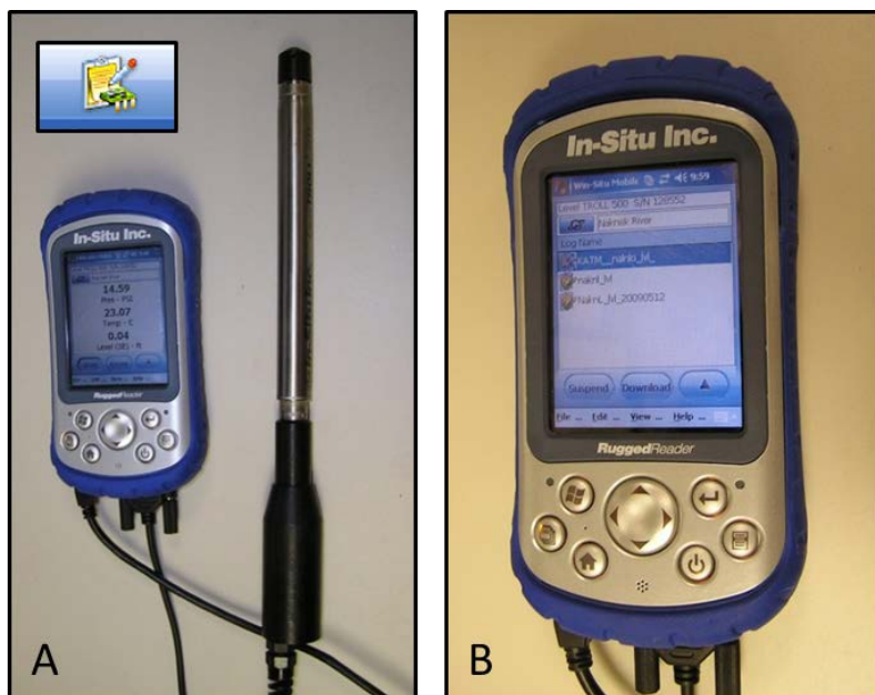
Figure 10.7. The Rugged Reader connected to the LevelTroll via the TrollCom and serial cable (A). Downloading is initiated by selecting the Logging icon (inset), and then highlighting the active file and clicking the Download button (B).
