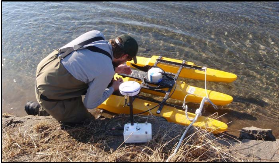
Figure 6.2. Assembling the ADCP-Trimaran unit on the lower Brooks River, Katmai National Park and Preserve. The DGPS mounting rod and antenna are pictured in the foreground.
