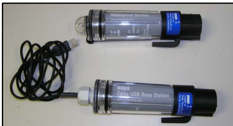
Figure 8.7. Optical readers for Onset HOBO Water Temp Pro v2 loggers: the Optic USB Base Station (bottom) and the Waterproof Shuttle (top).
