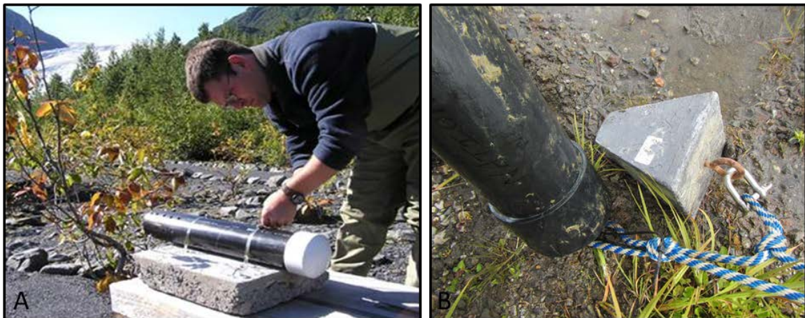
Figure 4.4. For continuous monitoring, the sonde is placed in a PVC housing moored via hose clamps cast in concrete (panel A) or line secured to a metal anchor (panel B).
