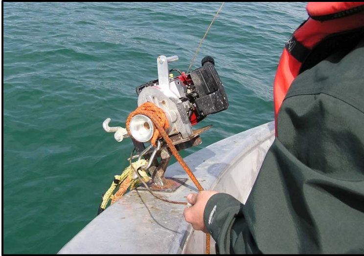
Figure 8.9. The capstan winch is used to retrieve the instrument line to the depth of the bridle line. Although not worn in this photo, gloves are strongly encouraged.
