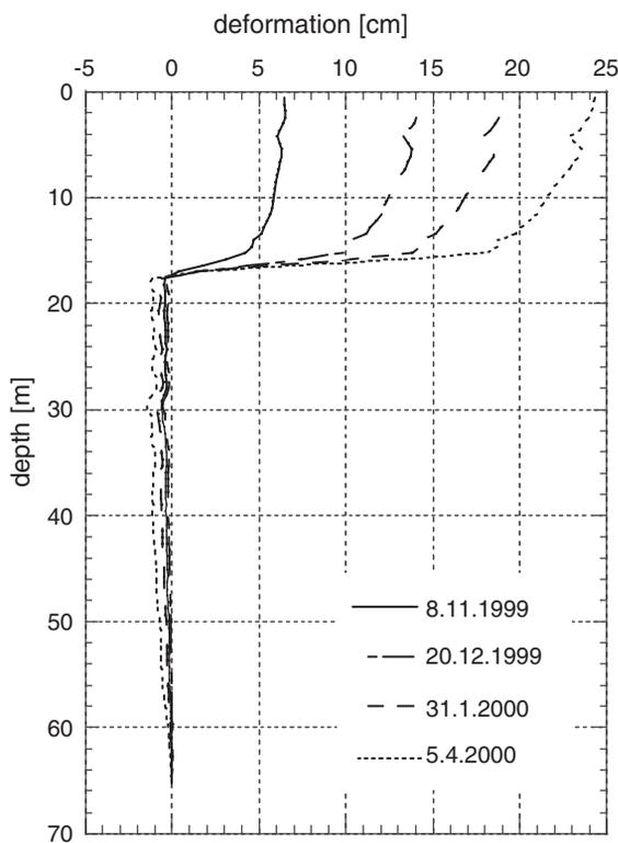
Figure 1. Deformation profile of Muragl rock glacier, borehole BH4 (from Arenson & Springman 2000).
