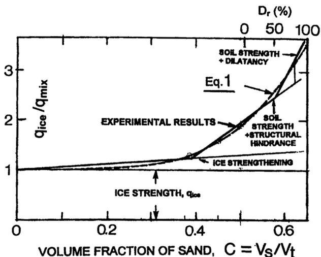
Figure 3. Variation of unconfined compressive strength of frozen Ottawa sand at  $-7^{\circ}\text{C}$ , and at a strain rate of  $4.4 \times 10^{-4} \text{ s}^{-1}$  (modified from Ting et al. 1983).
