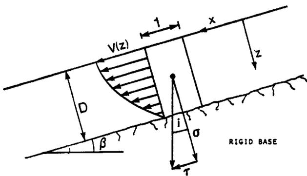
Figure 5. Notation for creep of an infinite slope on bedrock (after Andersland & Ladanyi 1994).
