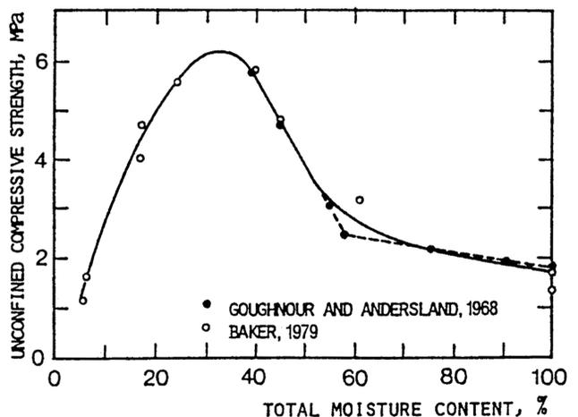
Figure 2. Effect of total moisture content on the unconfined compressive strength of a frozen fine sand at  $-12^{\circ}\text{C}$ , and at a strain rate of  $2.2 \times 10^{-6} \text{ s}^{-1}$  (after Baker 1979).
