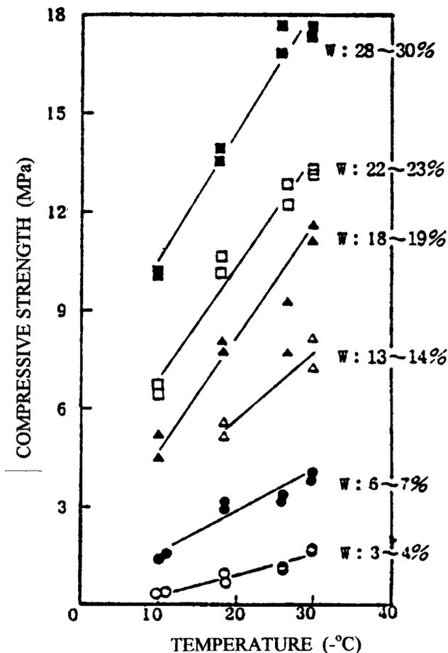
Figure 4. Relationship between uniaxial compressive strength and temperature for a frozen sand at different total water contents (after Kuribayashi et al. 1985).
