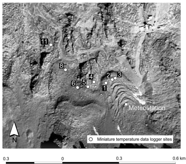
Figure 2. Measurement sites with miniature temperature data loggers in the Murtèl-Corvatsch area, Upper Engadine, Switzerland. Background: Infrared aerial (here presented in greyscale) photograph of the Swiss Office of Topography from 7.9.1988. Aerial photograph archive FD/KSL, Flightline: 061161, Image No. 4770.
