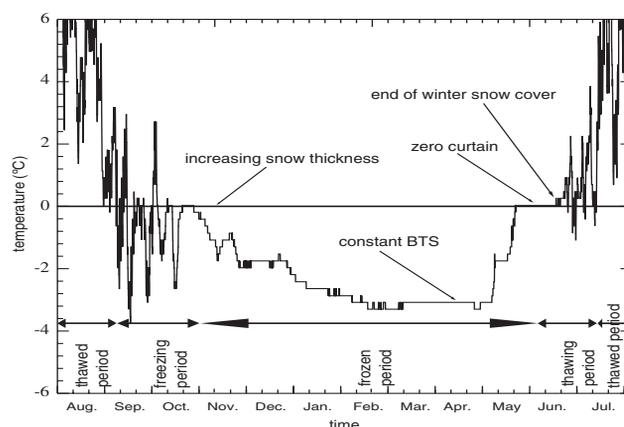
Figure 1. Typical miniature temperature data logger recording from permafrost in the Alps, indicating a set of interesting site characteristics.
