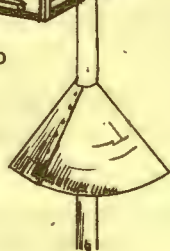
An inverted aluminum cone can be used to prevent squirrels from climbing the pole to a tray feeder. If trees or shrubs are nearby, however, squirrels will leap onto the feeder.
