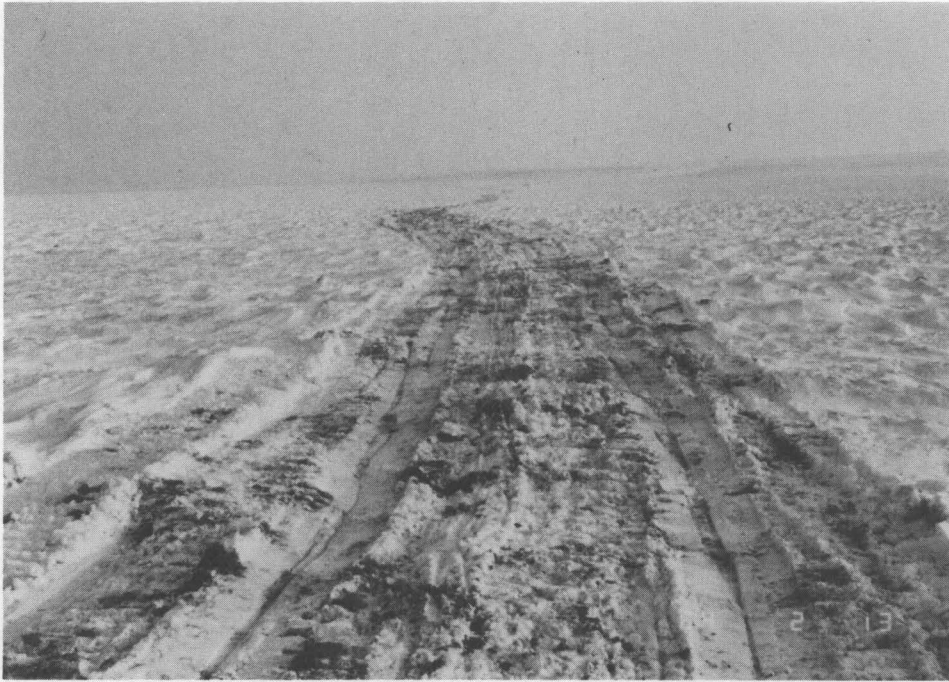
Plate 7. Disturbance due to multiple vehicle passes along a narrow trail in an area of high micro-relief.
