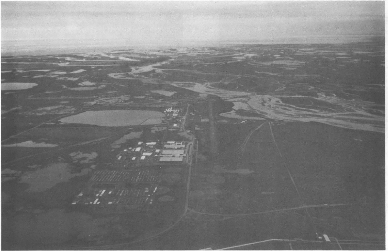
Plate 15. The ARCO complex at Prudhoe Bay, consisting of gravel roads, gravel pads for storage and buildings, and a gravel airstrip. The Sagavanirktok River empties into the Beaufort Sea in the background.
