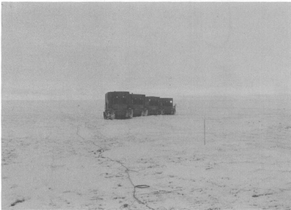
Plate 3. Tracked vibrators proceeding along seismic line in parallel.
