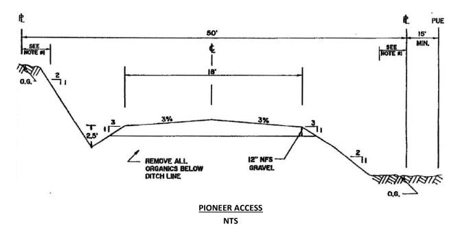
NOTES: #1 ROW OR SLOPE EASEMENT TO CONTAIN ALL CONSTRUCITON +5'. #2 MORE THAN 12" NFS GRAVEL MAY BE NEEDED FOR STABLE ROAD, DEPENDING ON SUBBASE.
