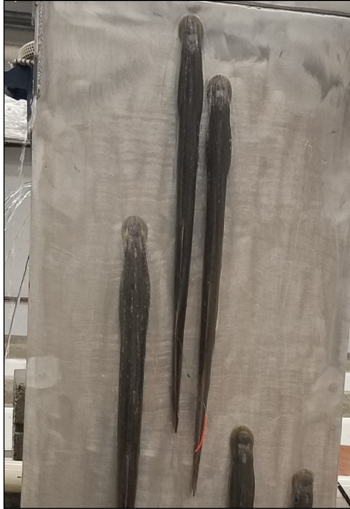
Figure 2. Example of Pacific Lamprey climbing a vertical surface during evaluation of wetted-wall structures designed to improve passage at dams. Credit: D. Lumley, Yakama Nation Fisheries.
